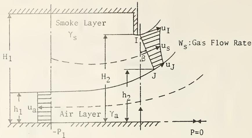
Effluent Gas Flow Rate Given by The Weir Flow Assumption
