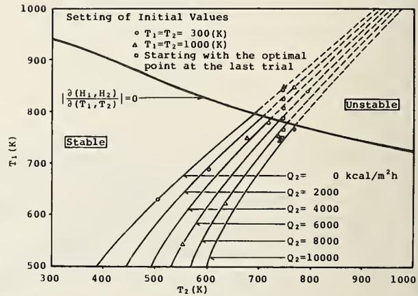
Figure 10 An Example of the Distribution of Augmented Lagrange Function in the Near Field of one Equilibrium Curve on  $Q_2$
