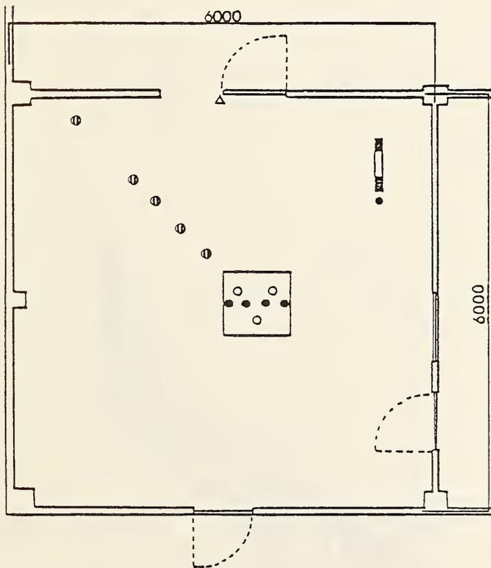
Figure 1. Experimental Setup of Burning Tests of Chairs
