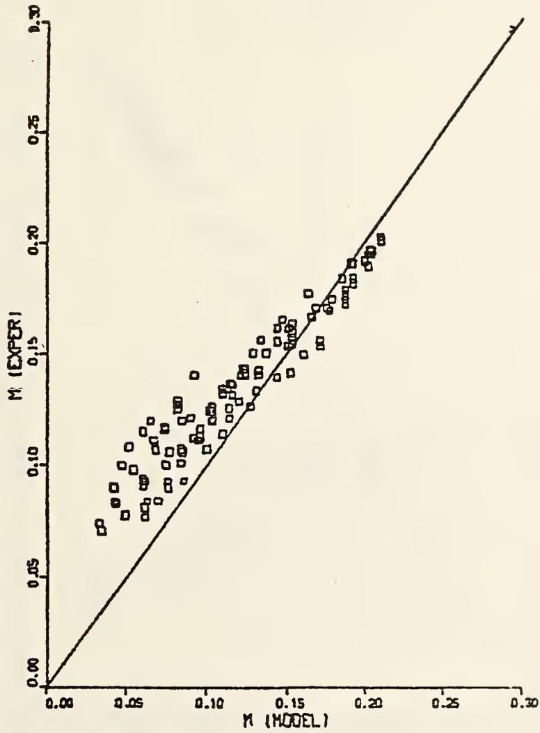
Figure 9. Comparison of dimensionless vent flow rate, experiment with theory
