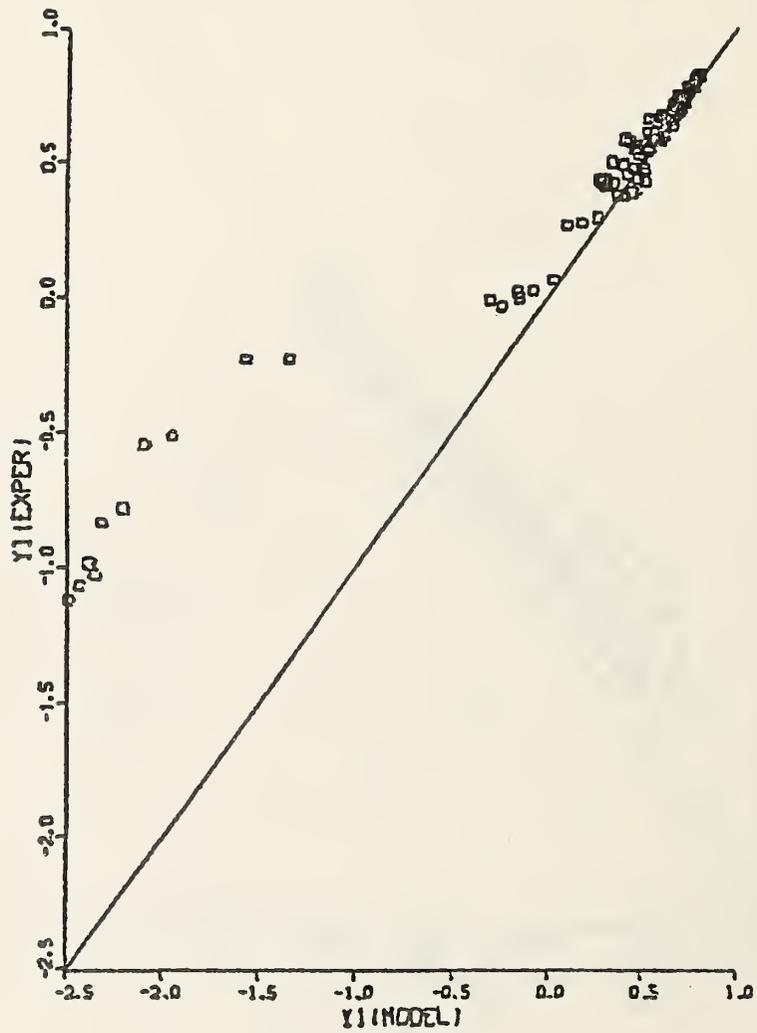
Figure 10. Comparison of dimensionless layer position, experiment with theory
