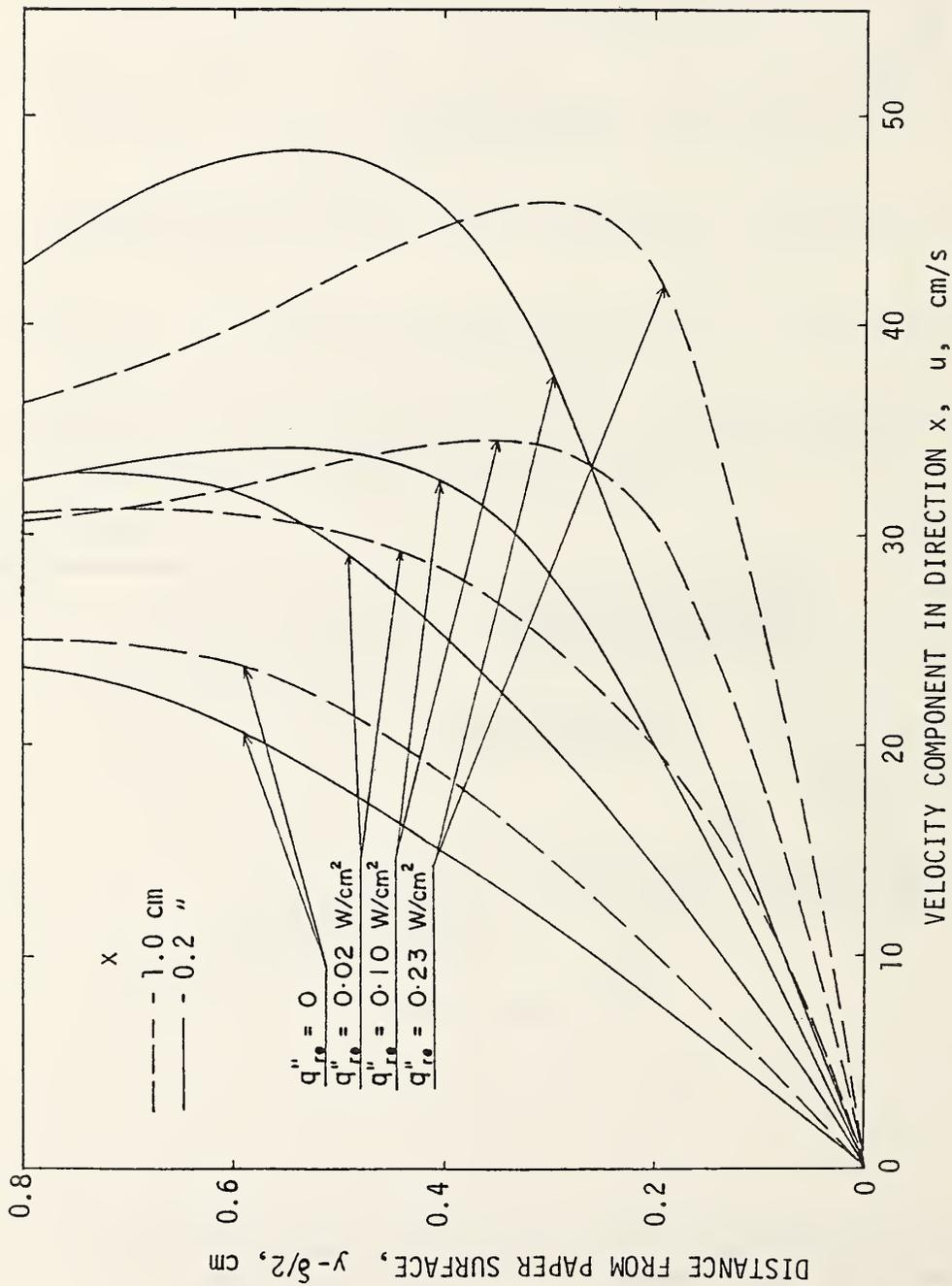
Figure 2. Velocity profiles just ahead of the pyrolysis front.  $x$ : distance from the pyrolysis front;  $\delta$ : test piece (paper sheet) thickness = 0.026 cm;  $q''_{re}$ : external radiation intensity.
