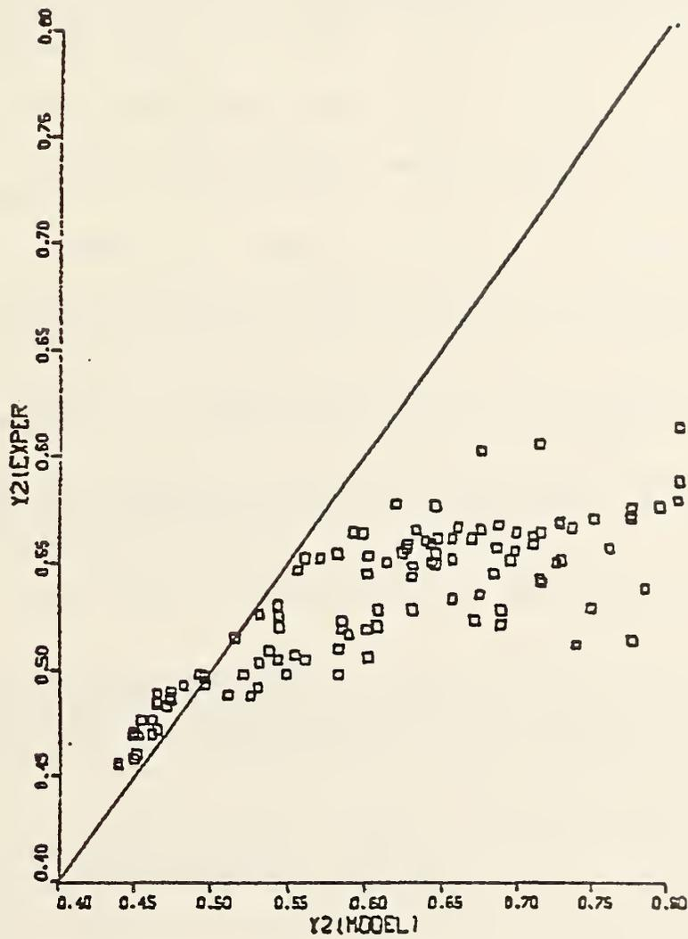
Figure 11. Comparison of dimensionless neutral plane, experiment with theory
