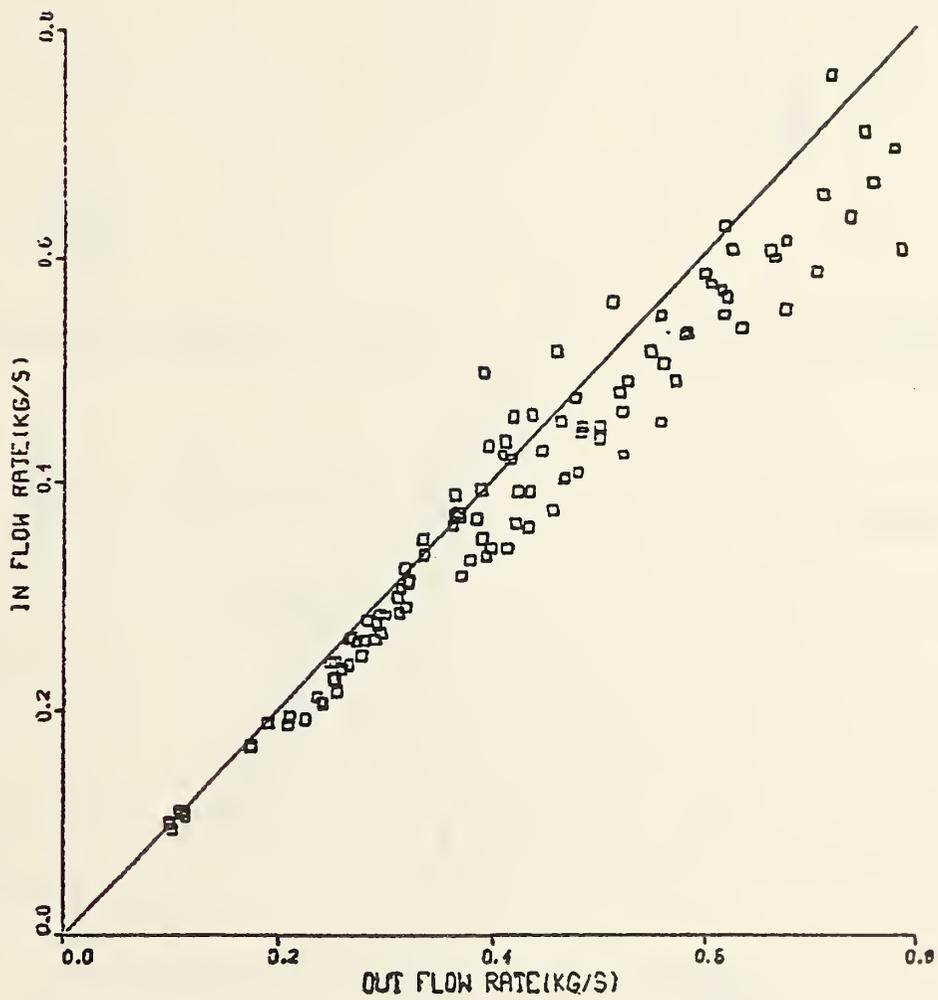
Figure 3. Comparison of inflow and outflow rates by approximate methods
