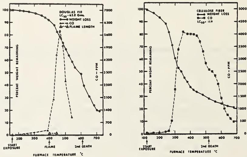
Figure 3. Decomposition pattern of Douglas fir and cellulose fiber (with flame retardant) and carbon monoxide evolution. Arrow at second death indicates the temperature at which the second of four exposed animals died (50% lethality).
