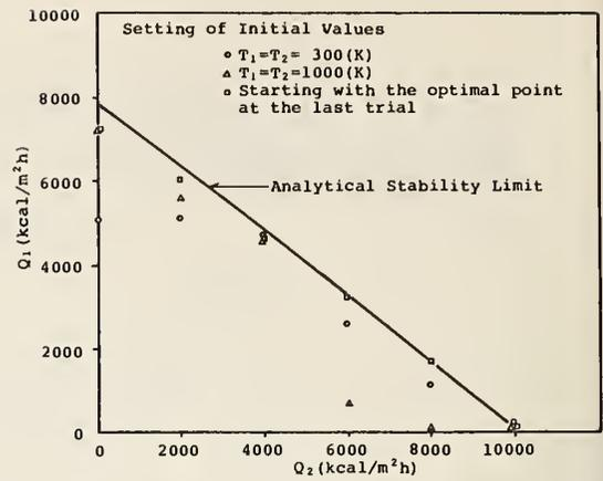
Figure 9(b) Comparison of Analytical and Numerical Stability Limit of Equilibria(Numerical Calculation by Augmented Lagrange Function Method with  $k=100$ )
