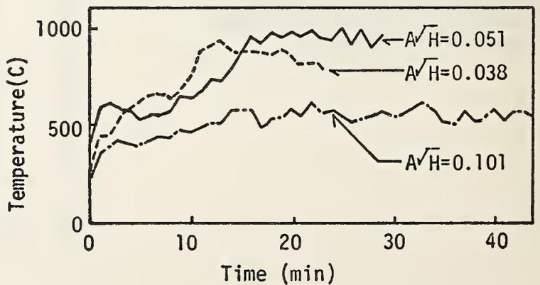
Figure 7 Time History of Total Heat Flux to Fuel Surface (0.15x0.15m Tray)
