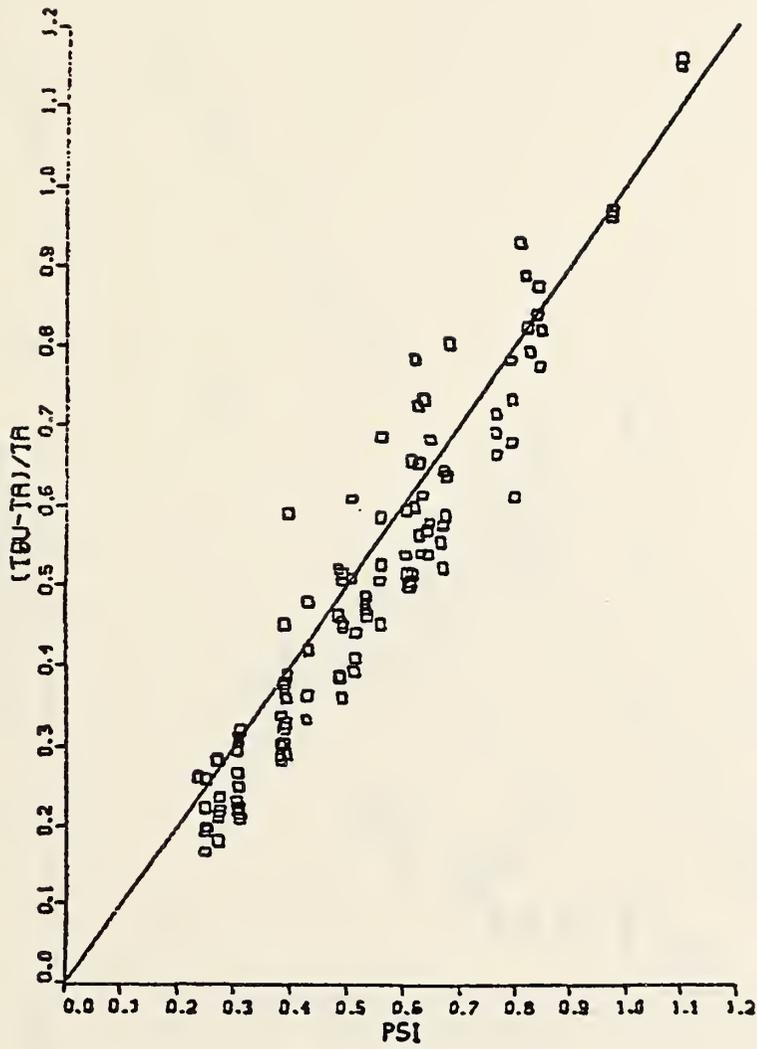
Figure 5. Dimensionless upper layer temperature correlation
