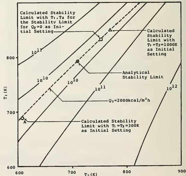
Figure 11(a) Comparison of Analytical and Numerical Criteria on the Occurrence of Flashover (Numerical Calculation by Augmented Lagrange Function Method with  $k=0.01$ )
