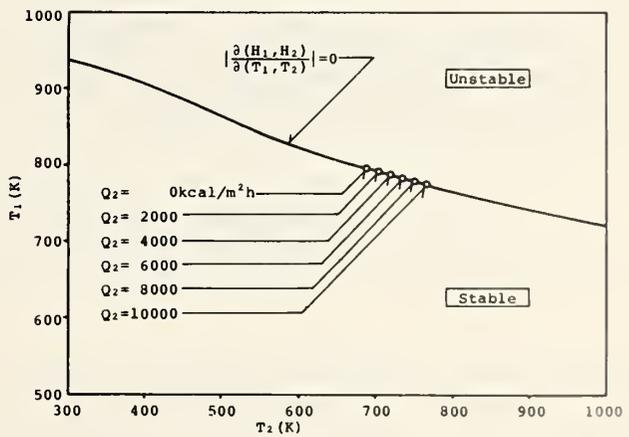
Figure 12 Comparison of Analytical and Numerical Lower Bounds of the Critical Temperature of Zone 1
