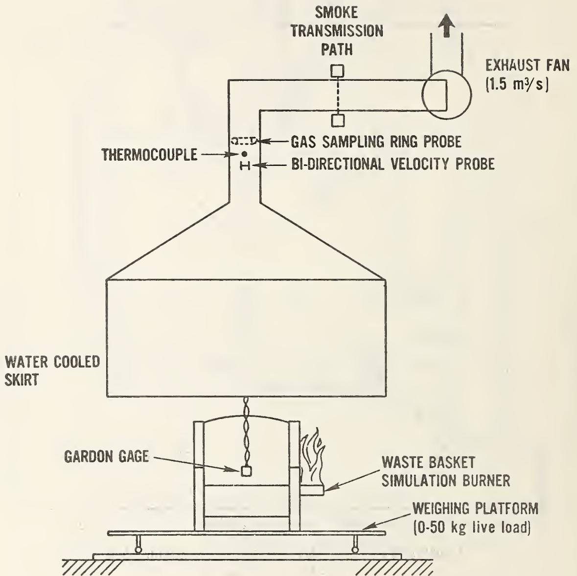
Figure 4. Schematic layout of furniture calorimeter
