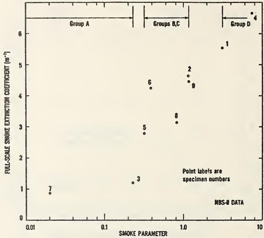
Figure 2. Relation between smoke measurements taken in bench-scale and full-scale behavior of mattresses in room fires
