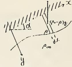
Fig 2 Diagram of flow below the inclined ceiling
