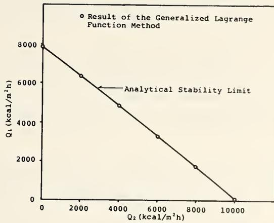
Figure 11(b) Comparison of Analytical and Numerical Stability Limit of Equilibria (Numerical Calculation by Augmented Lagrange Function Method with  $k=0.01$ )
