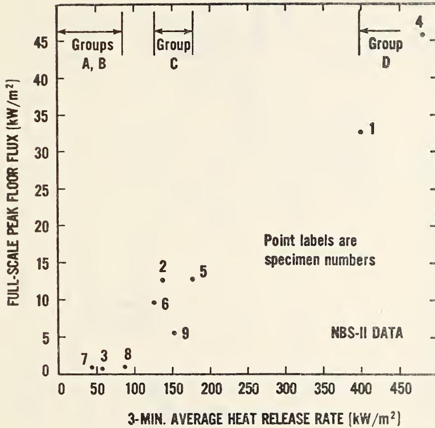
Figure 1. Relation between bench-scale heat release rate measurements and full-scale behavior of mattresses in room fires
