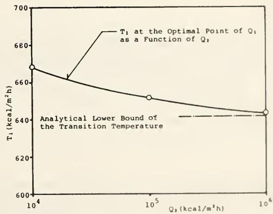
Figure 13 Influence of Combustion Heat of Material on the Criteria of the Occurrence of Flashover
