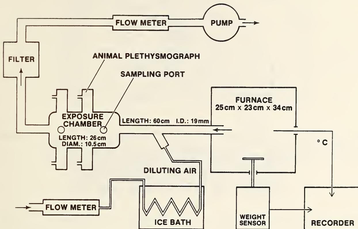
Figure 1. Experimental arrangement to study toxicity of smoke from thermal decomposition of synthetic or natural polymers. From Alarie and Anderson, 1979.
