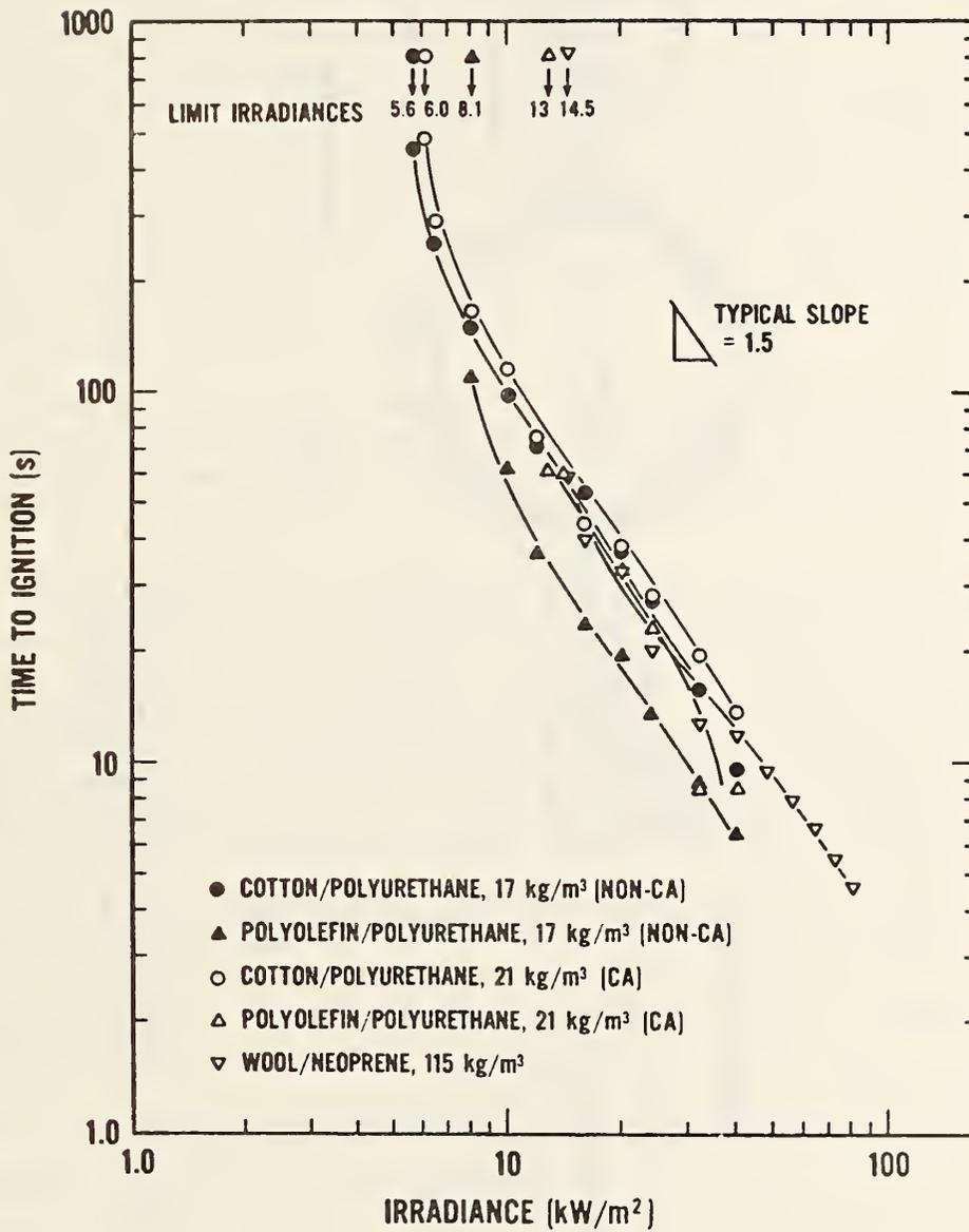
Figure 7. Typical ignition curves for a range of upholstered furniture fabric/filling combinations
