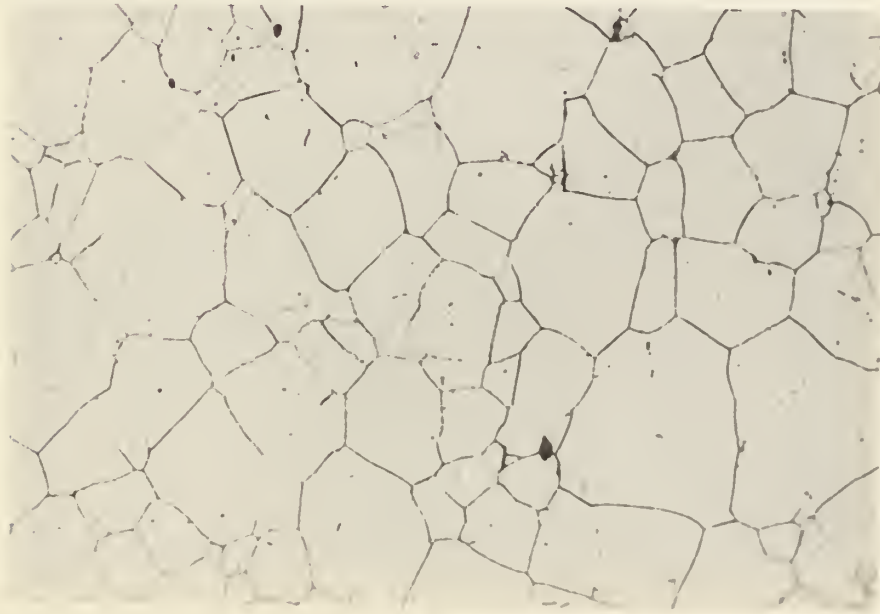
Triple Walled Material - Chimney Sensitized 500X
