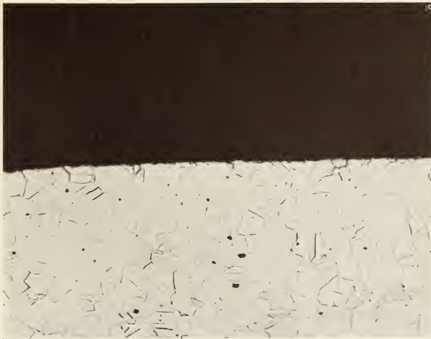
Edge of Double Walled Material 500X After Sensitization
