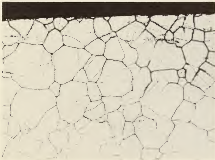
Triple Walled Material After Sensitization 500X
