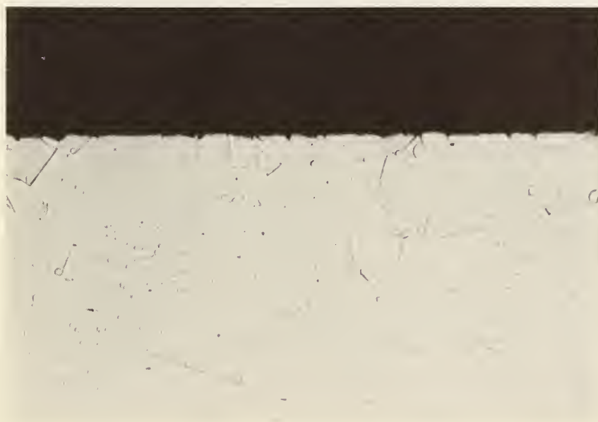
Edge of Type 304 Chimney Section from Field 500X
