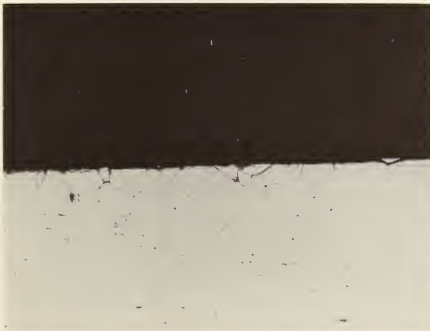
Edge of Triple Walled Material After Exposure 500X
