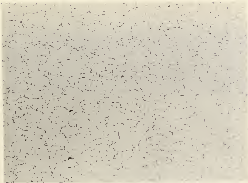
Type 321 Stainless Steel After Sensitization Heat Treatment
