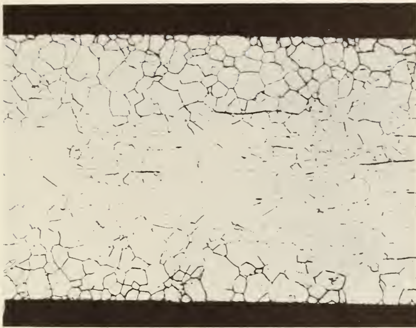
Through Thickness Section of Triple Walled 200X Material After Sensitization
