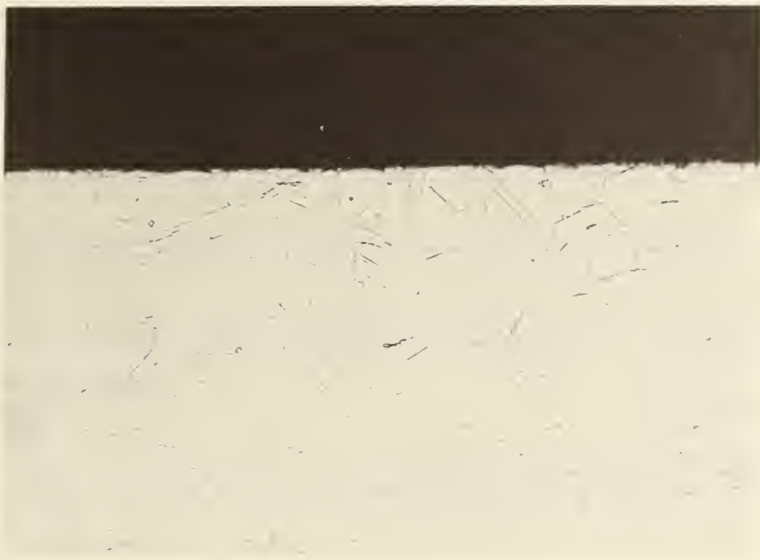
Type 304 Chimney from Lab Tests 500X Showing Carbides
