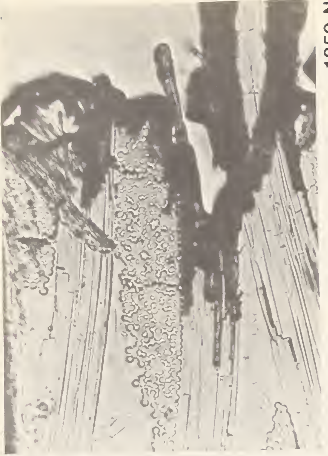
Figure 10. Edge damage corresponding to loads of Fig. 9. Note large crack opening displacements between broken fiber ends at 1850 N in the region of final fracture.
