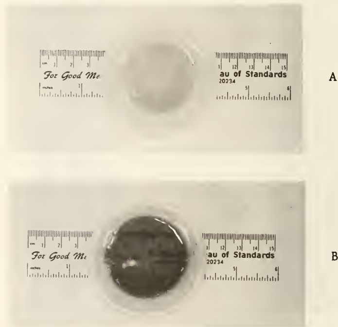
Figure 4. G-11 resin system as hand mixed (A) and after three minutes of ultrasonic blending (B).
