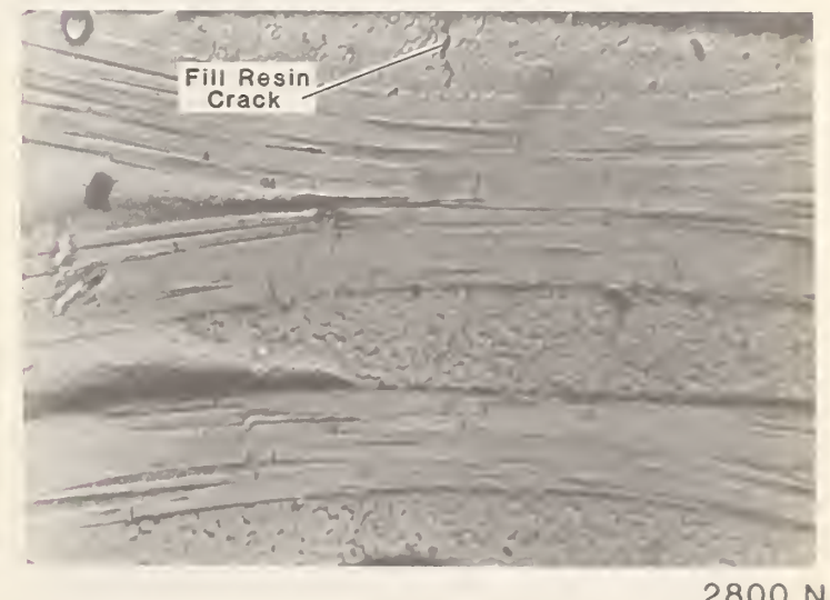
Figure 12. Top and edge views of damage corresponding to loads of Fig. 11. Damage in top views are fill resin cracks often observed as shadows below the surface.
