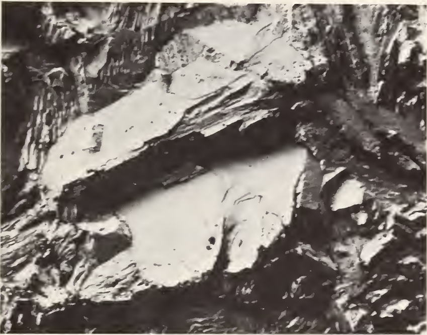
Figure 4. Crystallographic facets on the overload fracture zone of coarse-grained Fe-18Cr-3Ni-13Mn-0.37N steel fractured at 4 K.
