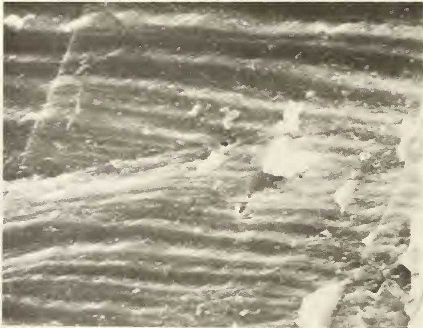
Figure 5. Microscopic steps and fine slip-line traces on a fatigue zone facet (facet a of Fig. 3).
