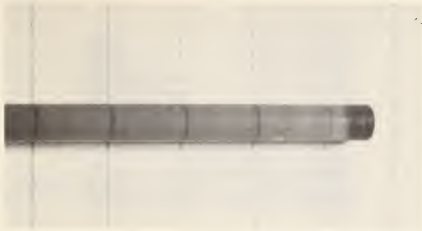
Figure 1. Transparency of a 3 mm diameter specimen containing 58 v/o glass indicates excellent fiber wetting and absence of porosity.
