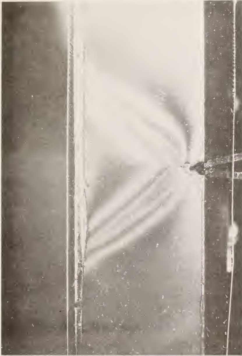
Figure 33. Photoelastic strain pattern of an SENT specimen; a/W \approx 0.2 .
