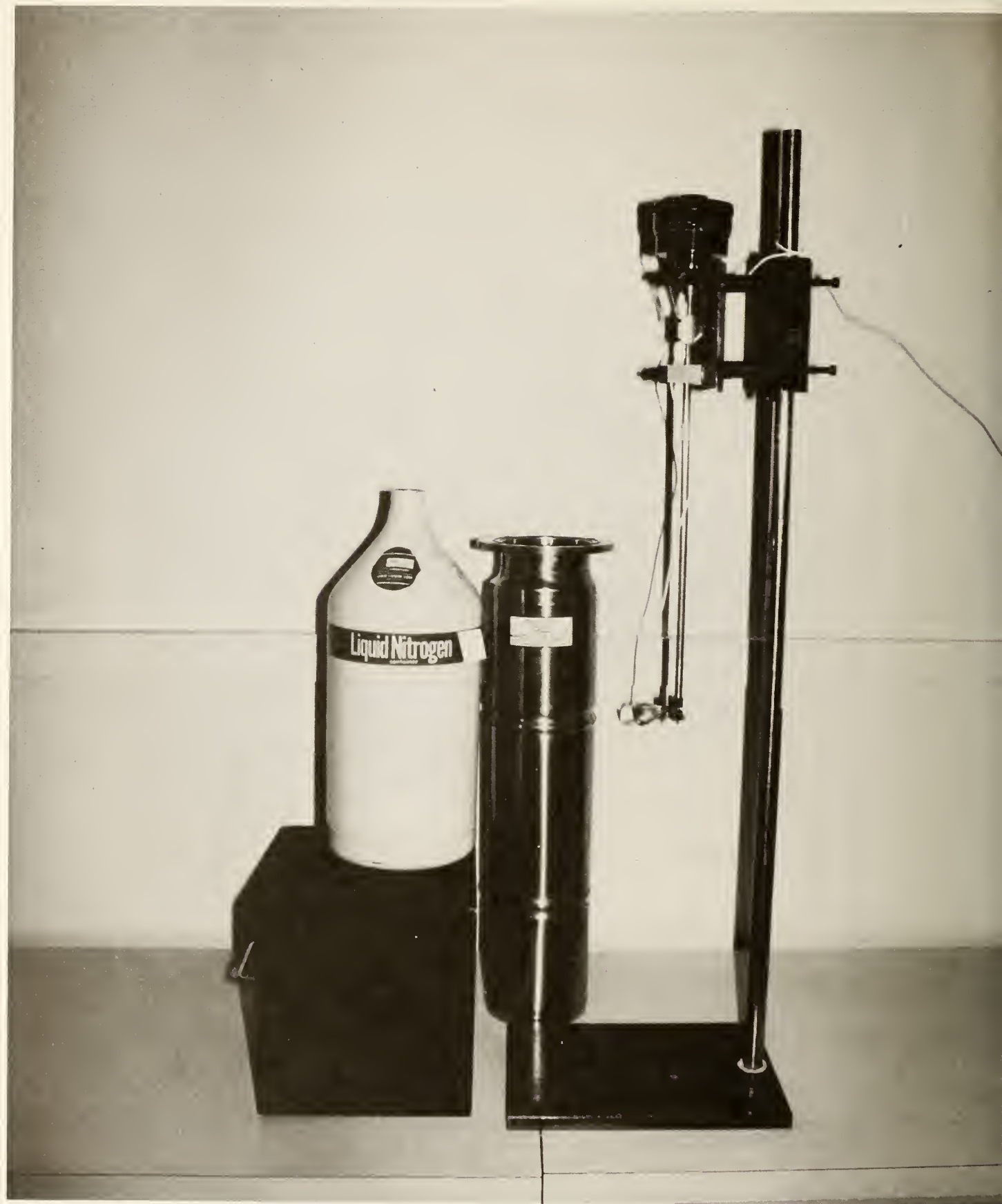
Figure 4. Cryogenic gage calibration apparatus.
