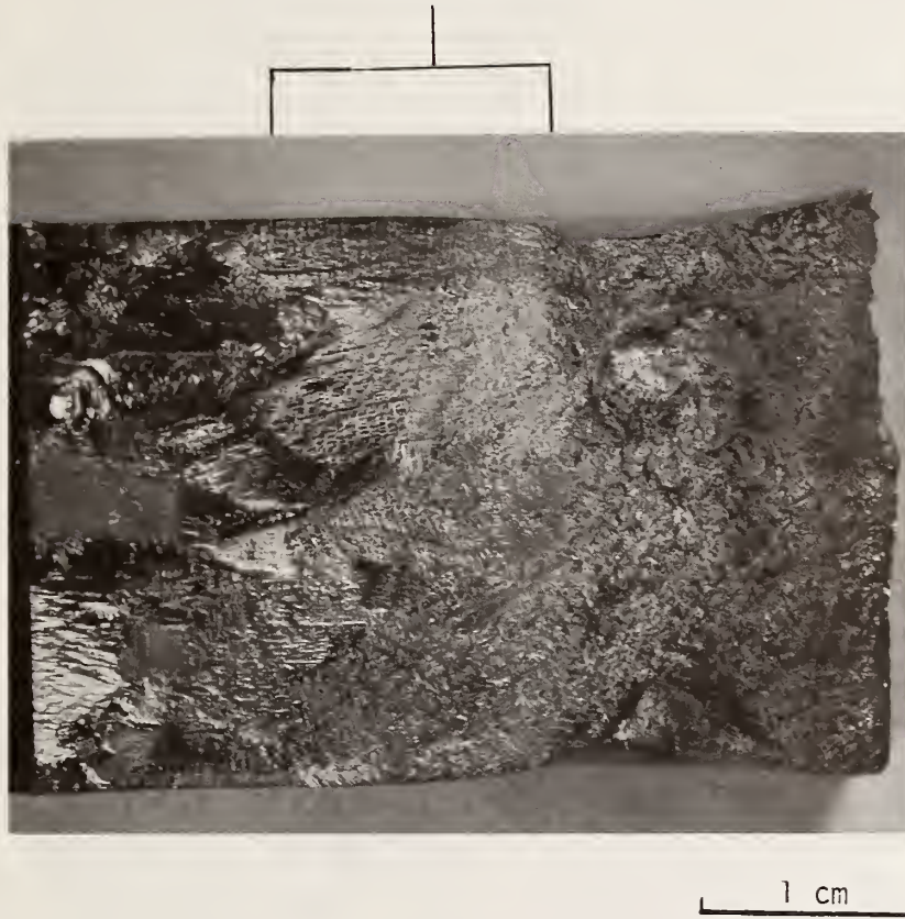
Figure 5 Fracture surface of CF8M casting with 1% ferrite at low magnification showing the relative roughness of the surface. The fracture surfaces of the castings with 8 and 29% ferrite appeared to be similar.
