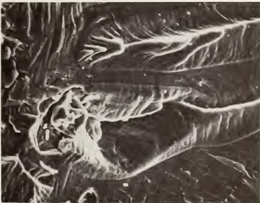
Figure 9. SEM photomicrograph of fatigue fracture surface of CF8M casting with 29% delta ferrite low \Delta K conditions.
