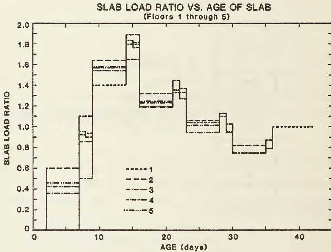
Figure 5.2 - Plot of Slab Load Ratio vs. Age of Slab
