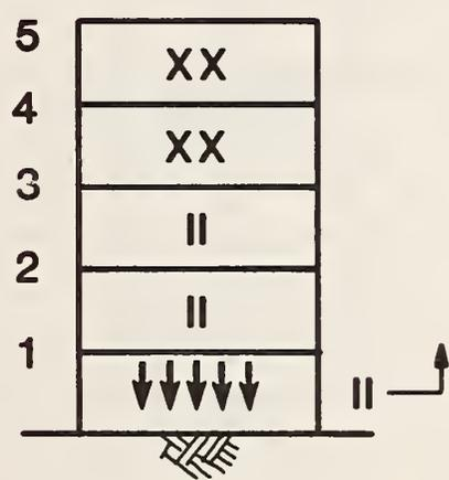
Figure 2.2 - Phase 2: Remove Reshores from the First Story
