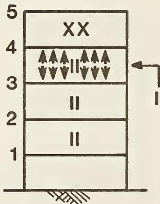
Figure 2.4 - Phase 4: Reshore the Fourth Story with Precompression
