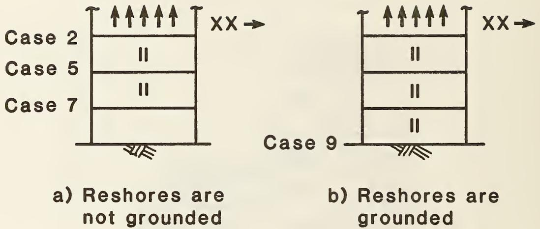
Figure 4.9 - Phase 3b Configurations
