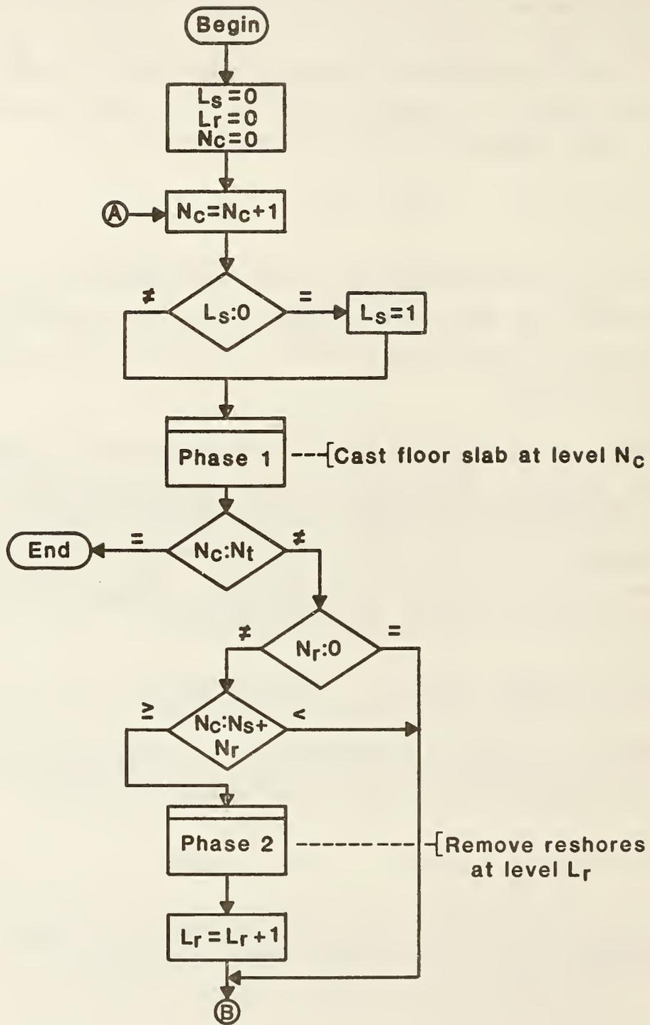
Figure 4.1 - Flowchart for Determining Next Phase
