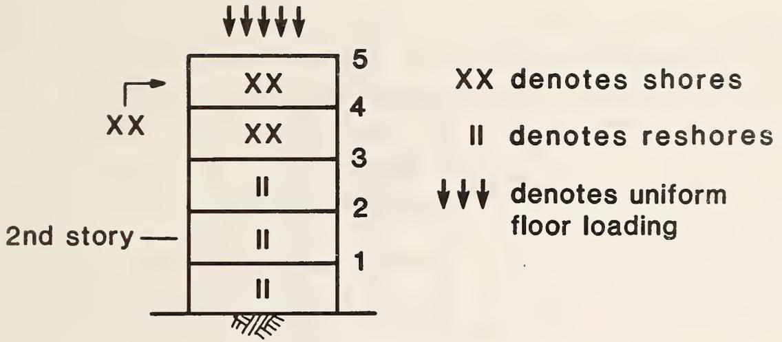
Figure 2.1 - Phase 1: Install Forms and Shores and Cast the Fifth Floor
