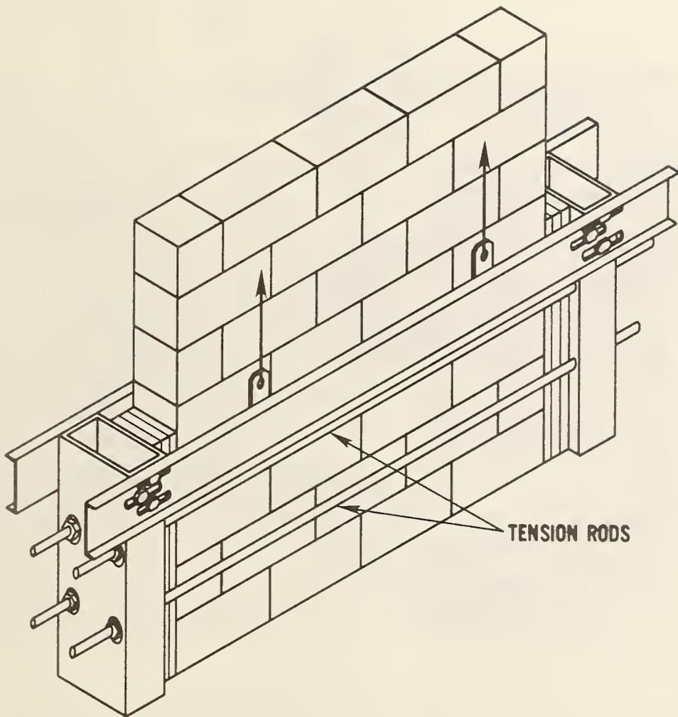
Figure 4.6 Wall panel transport harness
