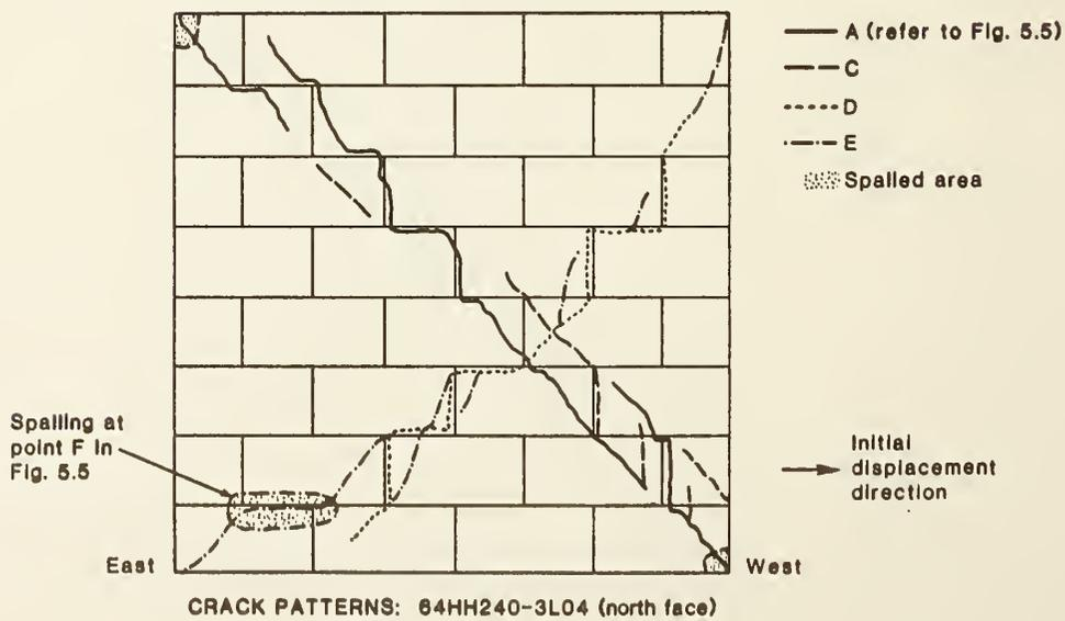
Figure 5.6 Specimen 64HH240-3L04 crack pattern
