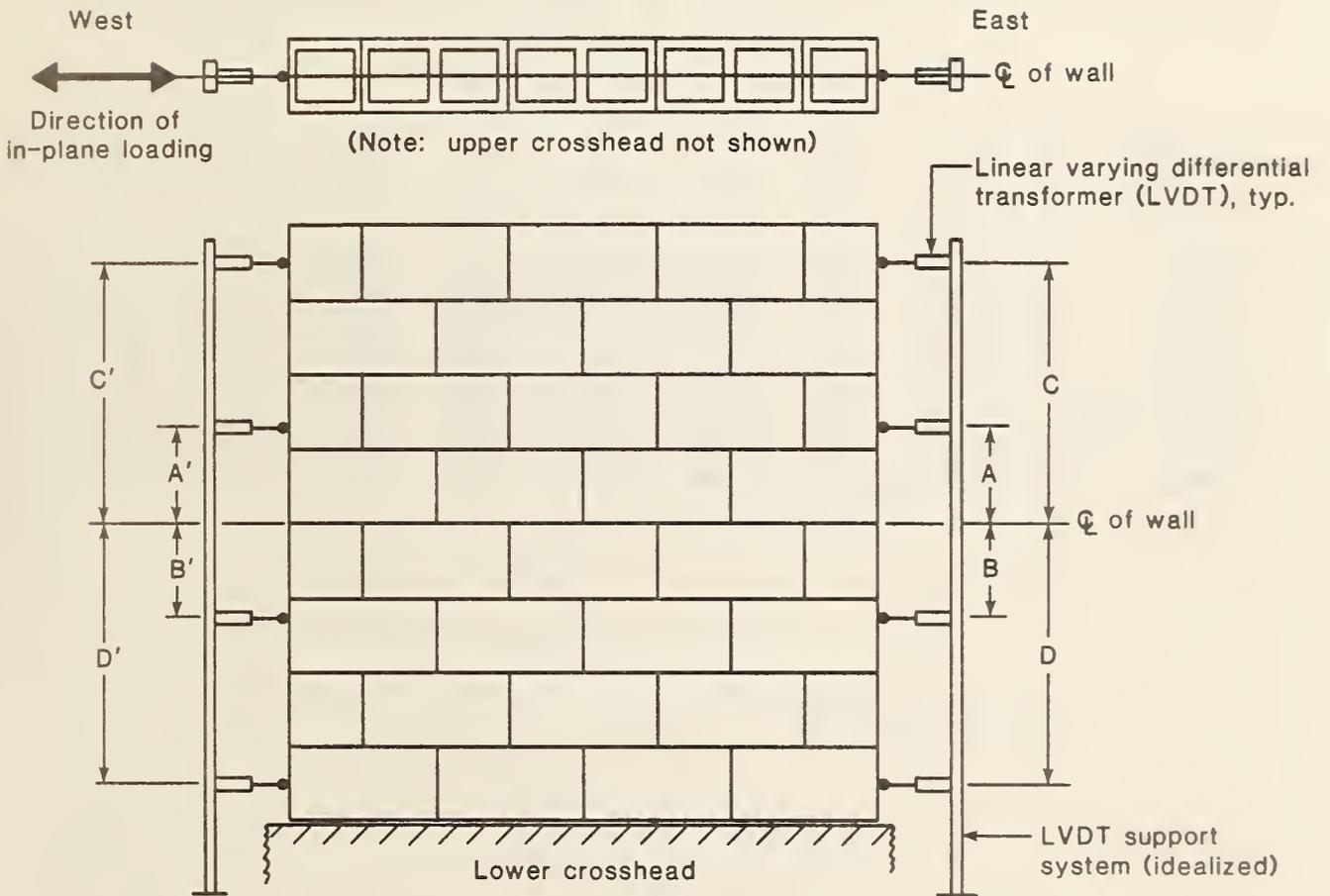
Figure 4.2 Wall panel LVDT layout
