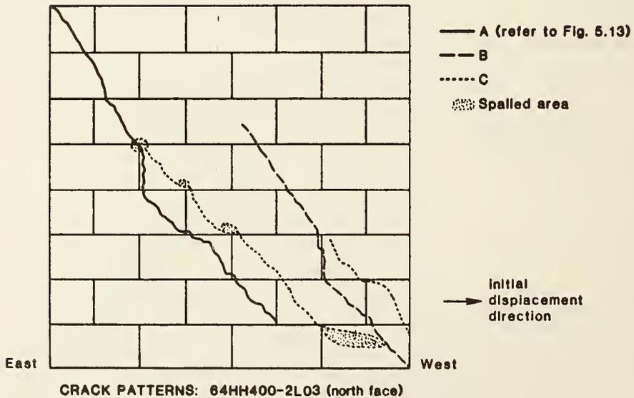
Figure 5.14 Specimen 64HH400-2L03 crack pattern
