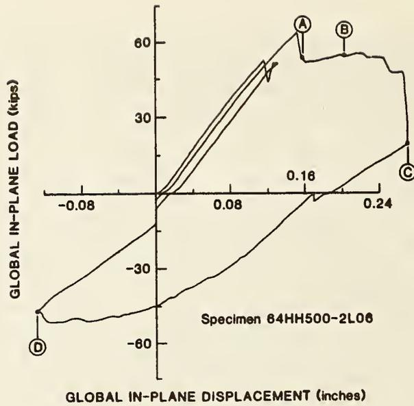
Figure 5.15 Specimen 64HH500-2L06 load-displacement curve
