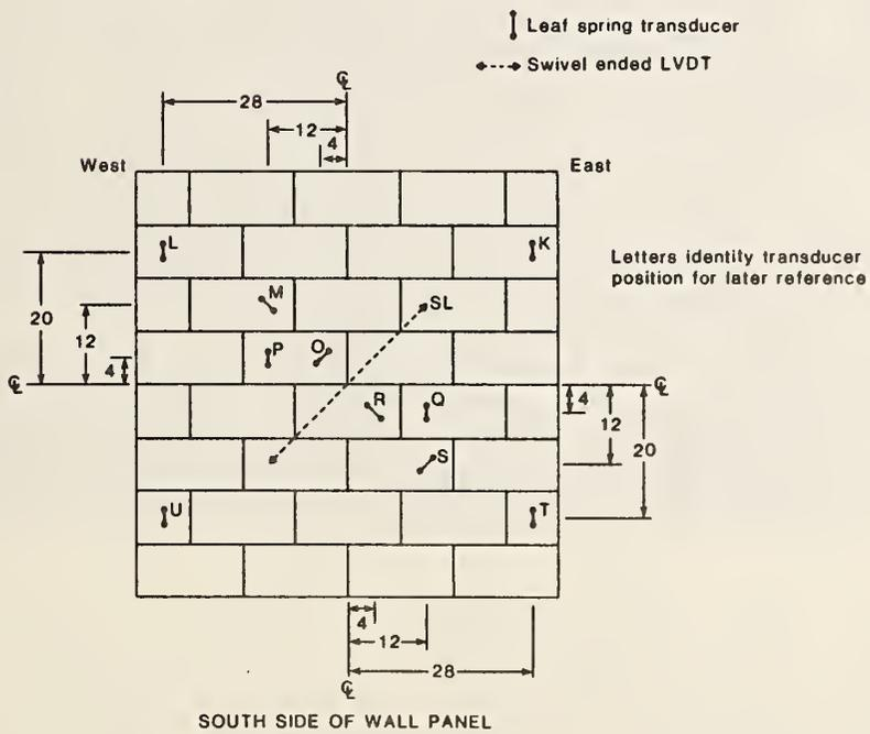
Figure 4.3 Wall panel instrumentation
