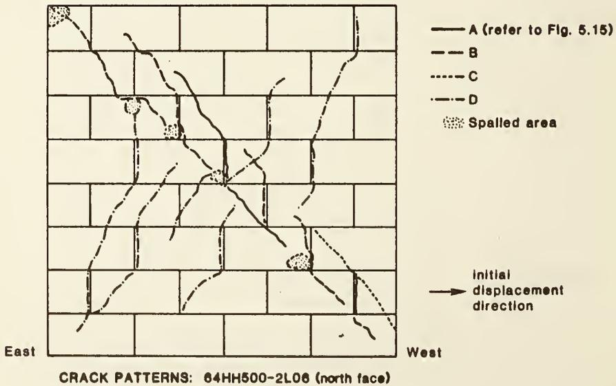
Figure 5.16 Specimen 64HH500-2L06 crack pattern
