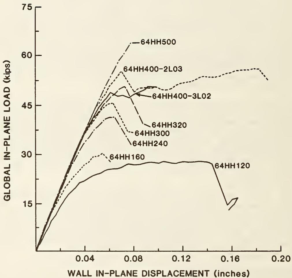
Figure 6.1. Combined load-displacement curves
