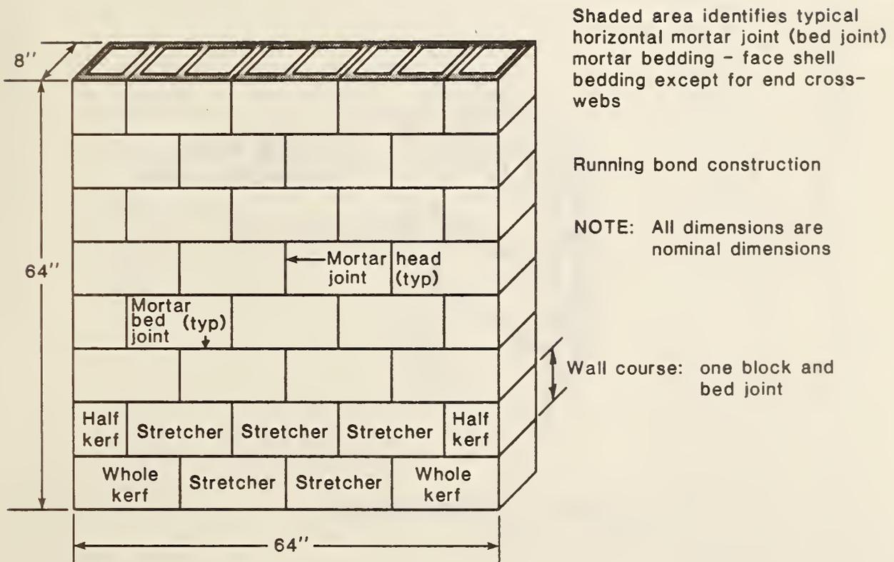
Shaded area identifies typical horizontal mortar joint (bed joint) mortar bedding - face shell bedding except for end cross-webs
