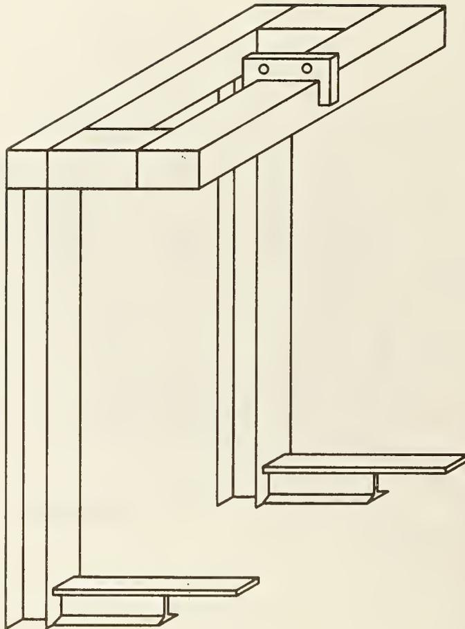
Figure 4.7 Wall panel lifting hook
