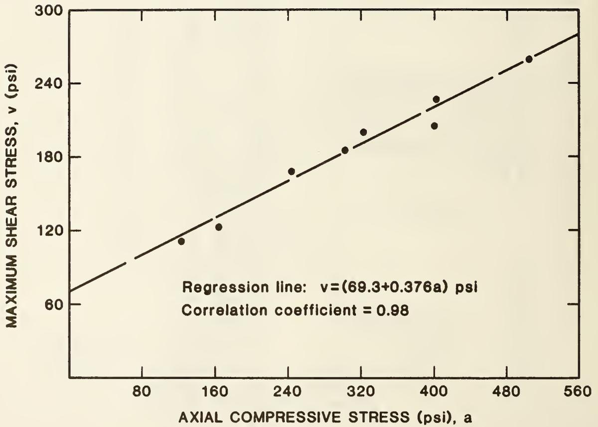
Figure 6.4. Maximum shear resistance versus axial stress
