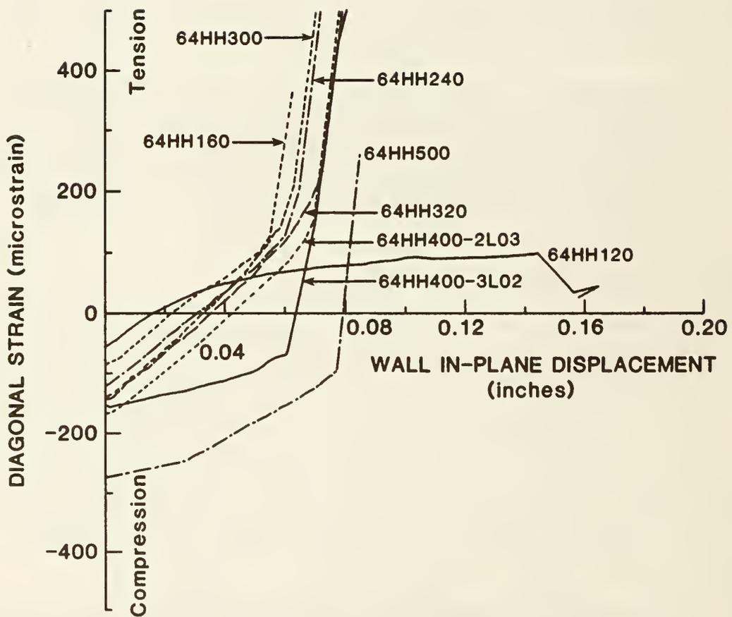
Figure 6.2. Combined diagonal strain-displacement curves
