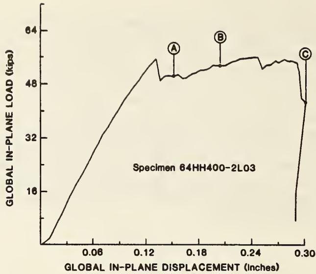
Figure 5.13 Specimen 64HH400-2L03 load-displacement curve
