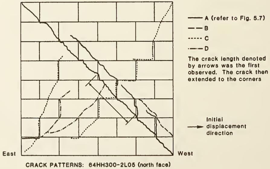
Figure 5.8 Specimen 64HH300-2L05 crack pattern
