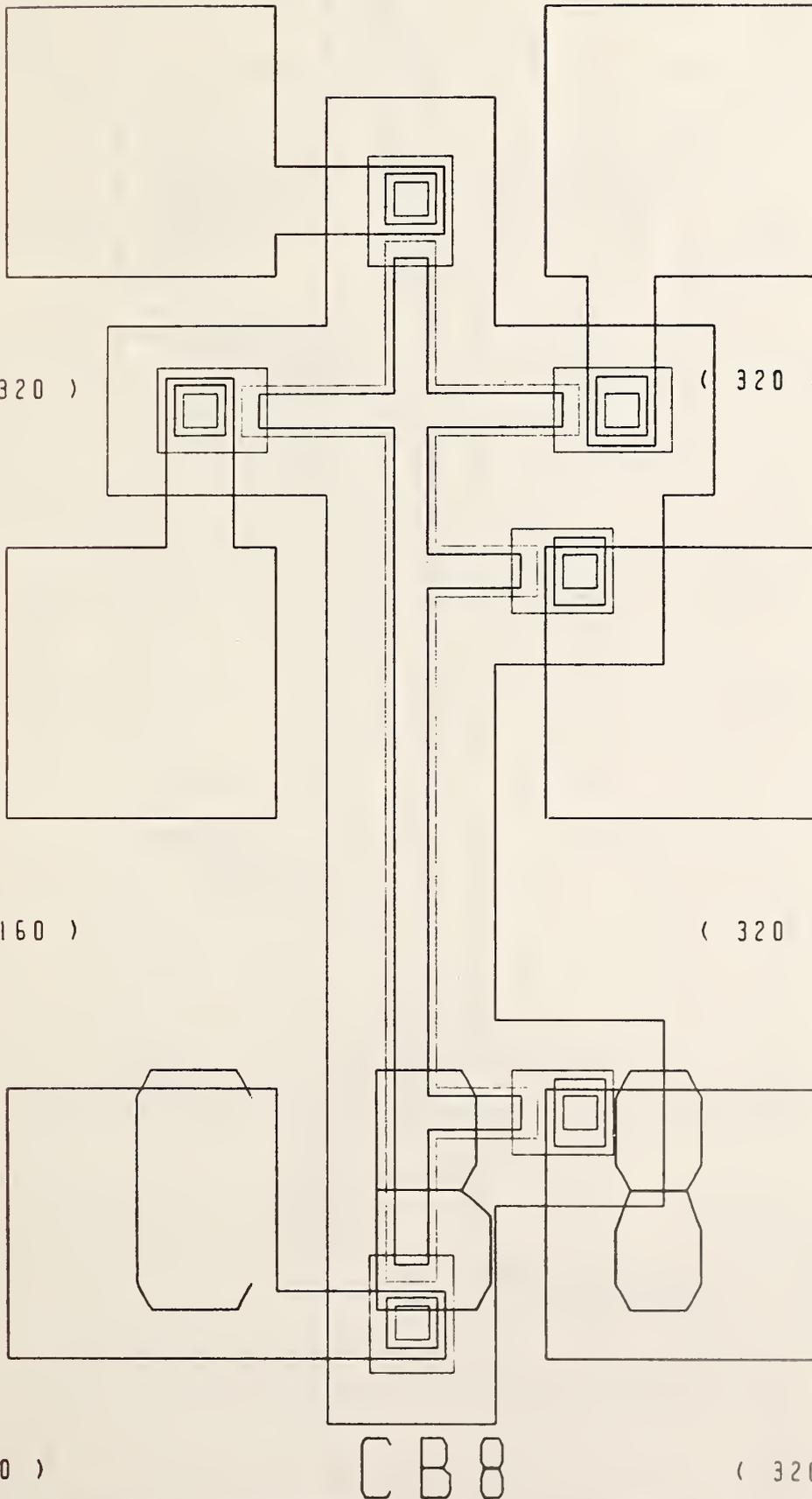
Figure 7. Cross-bridge sheet resistor CB-8.
