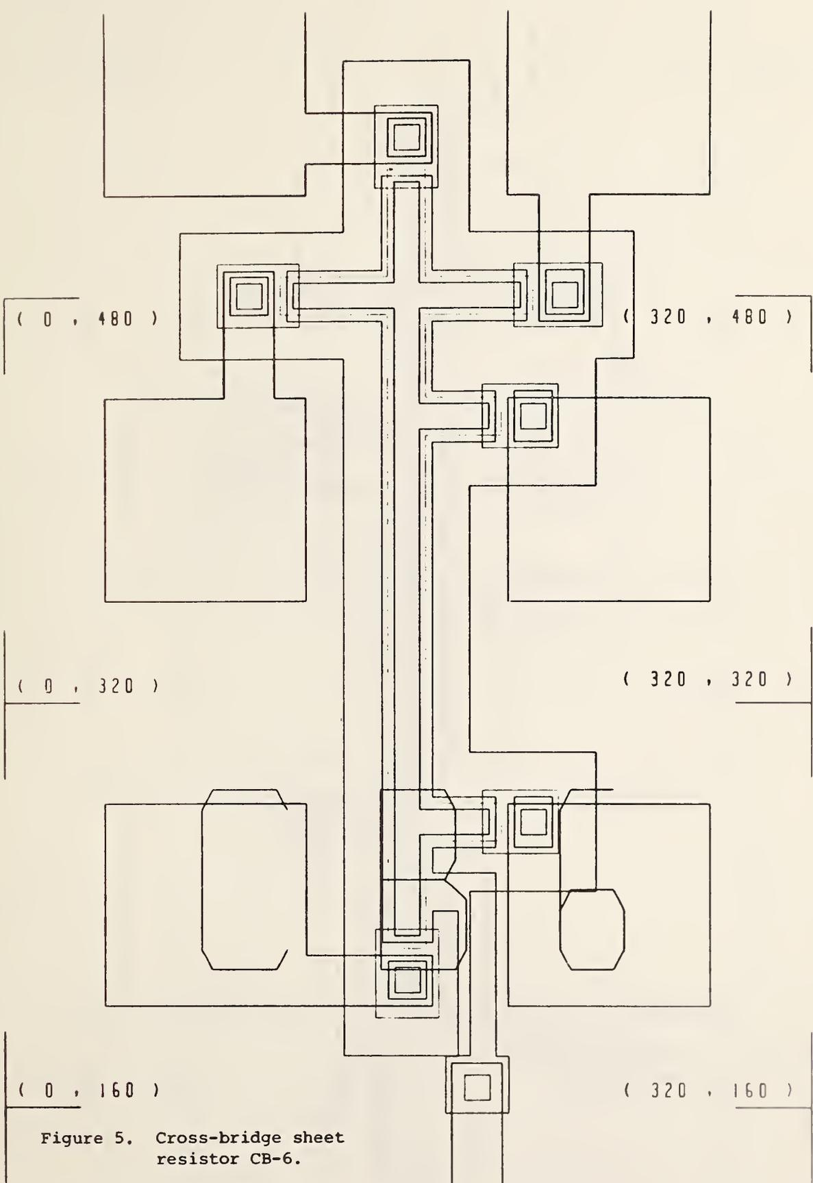
Figure 5. Cross-bridge sheet resistor CB-6.
