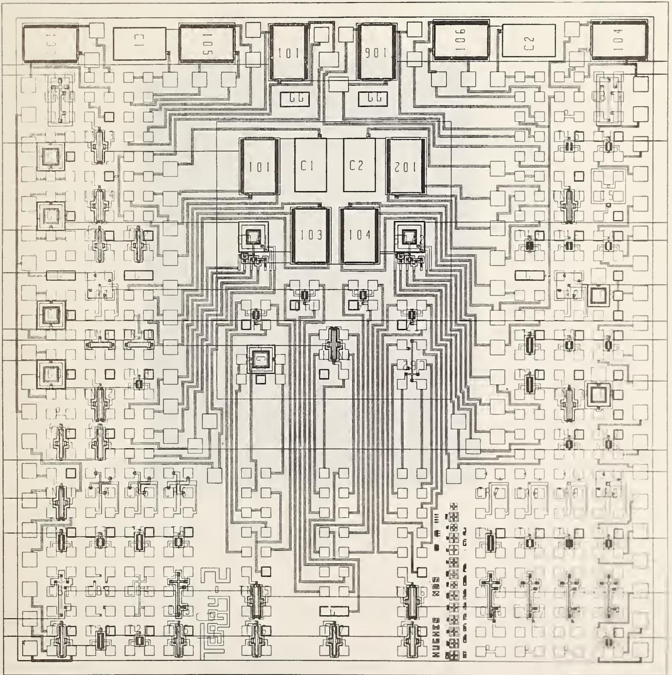
Figure 80a. TERRY-2 test chip layout schematic produced by the CAD system used to digitize the chip.
