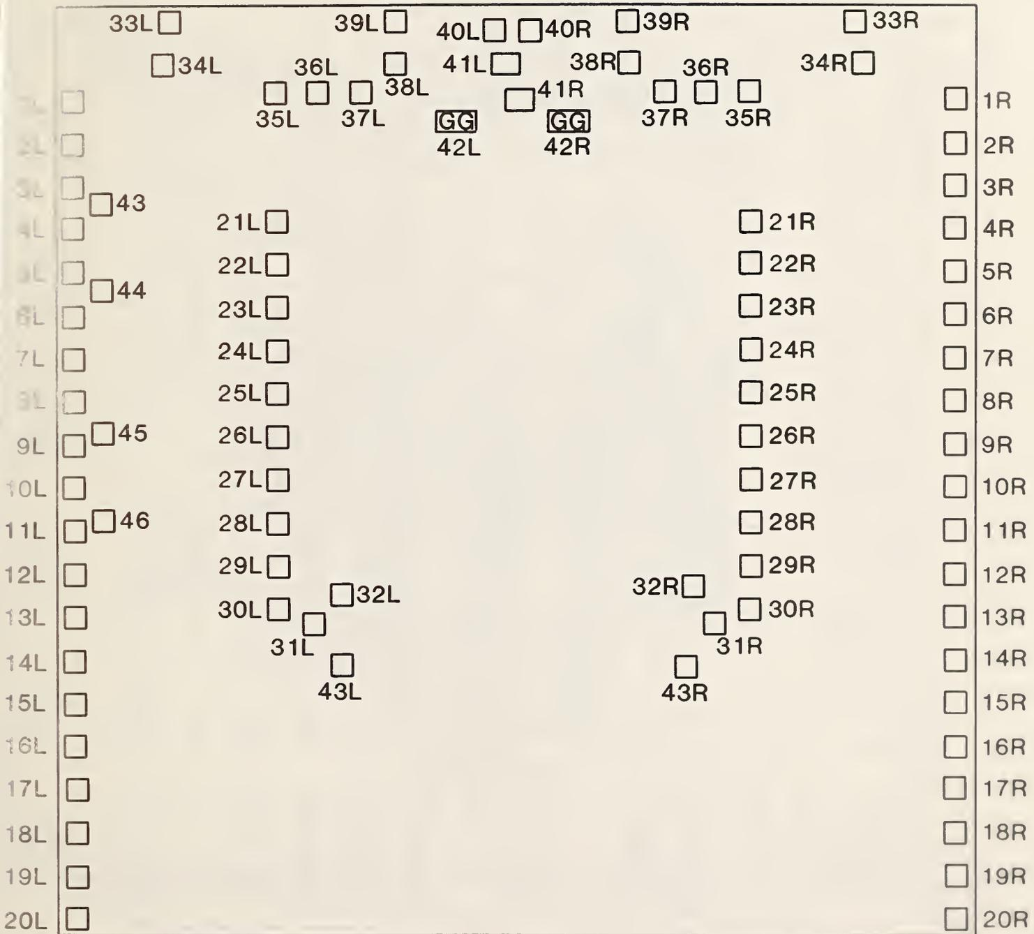
Figure 78. Schematic of TERRY-2 showing the locations and identifications of bonding pads.
