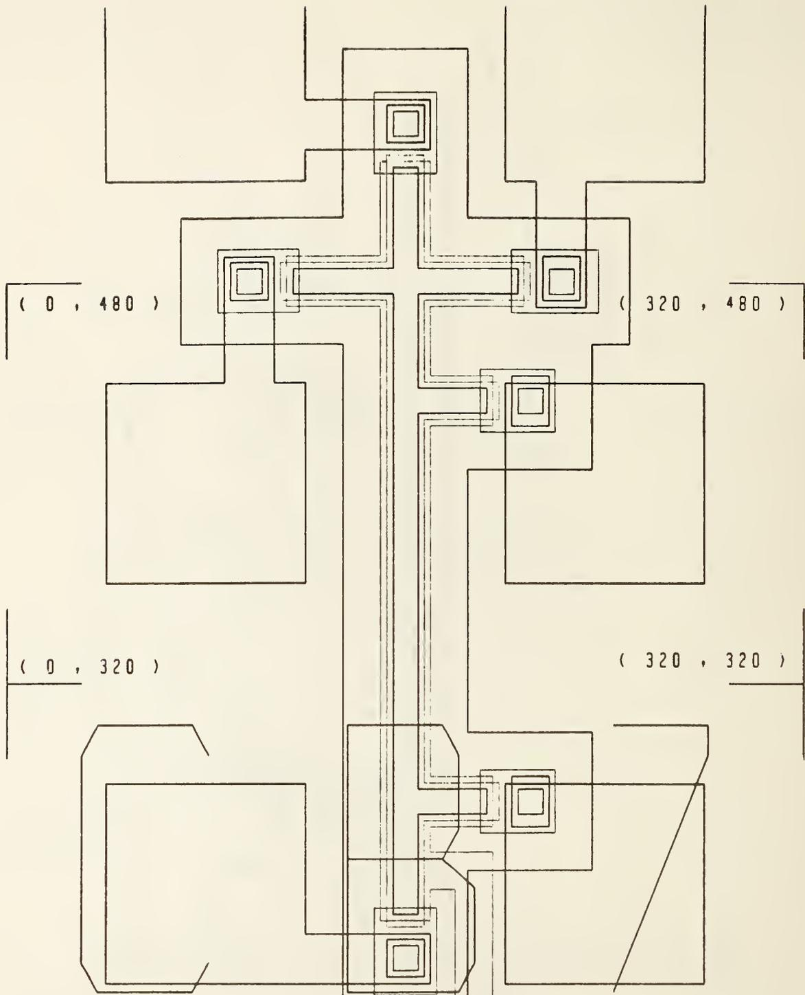
Figure 6. Cross-bridge sheet resistor CB-7.
