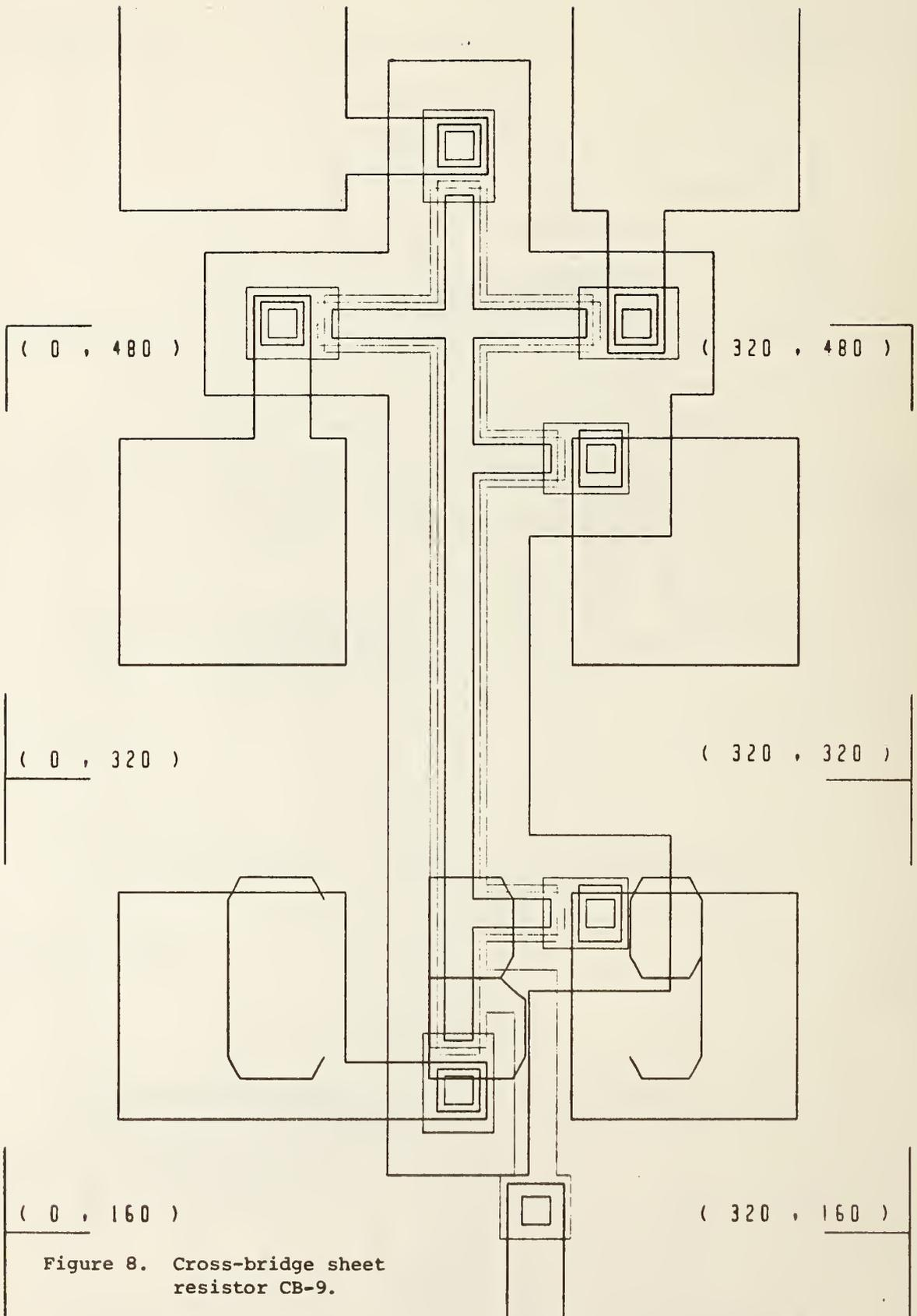
Figure 8. Cross-bridge sheet resistor CB-9.
