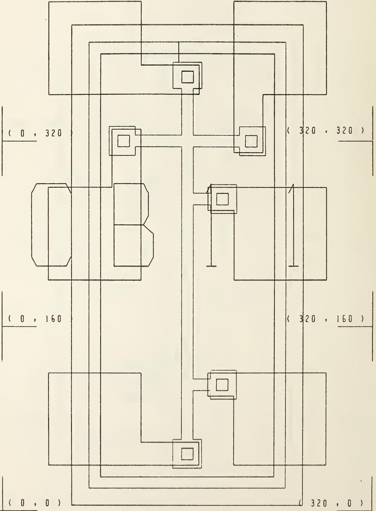
Figure 10. Cross-bridge sheet resistor CB-11,
