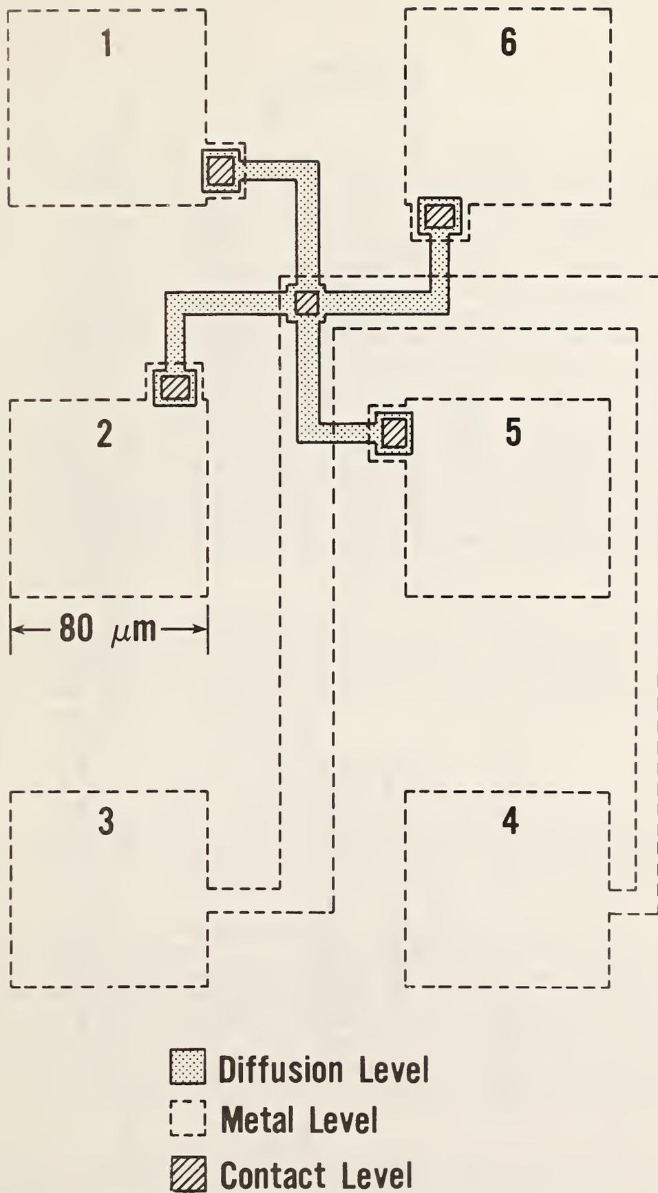
Figure 81. Schematic of a six-terminal metal-to-diffusion contact resistor (from Proctor *et al.*, 1983).
