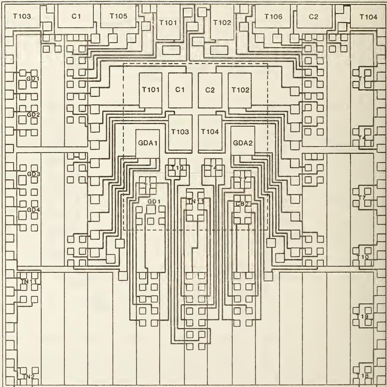
Figure 79. Schematic of TERRY-2 showing interconnections between test structures, probe pads, and bonding pads.
