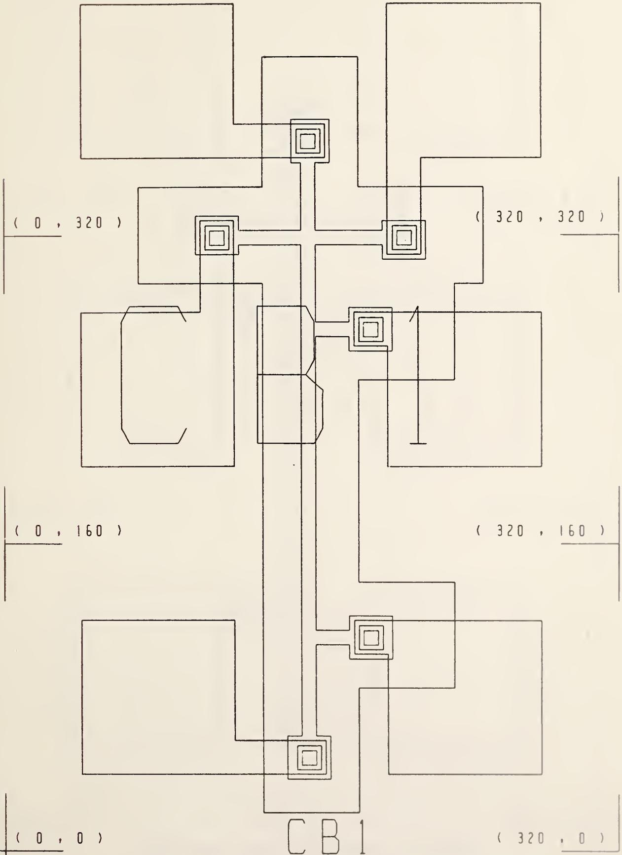
Figure 1. Cross-bridge sheet resistor CB-1.
