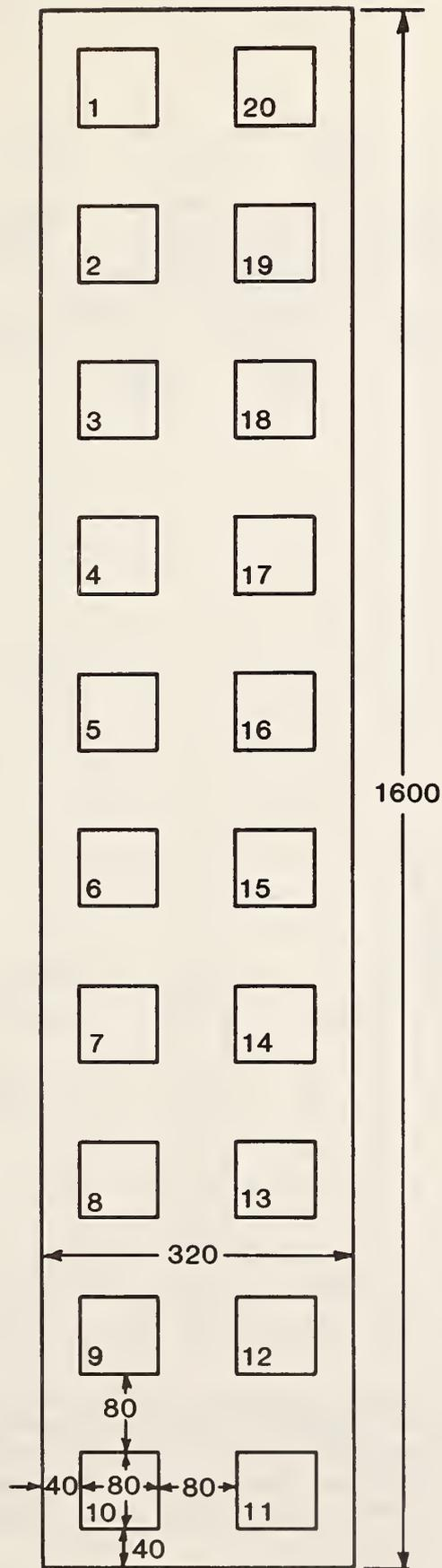
Figure 76. Cell probe pad array used for TERRY-2. Dimensions shown are in micrometers. Probe pads are numbered as shown at the lower left in each pad.
