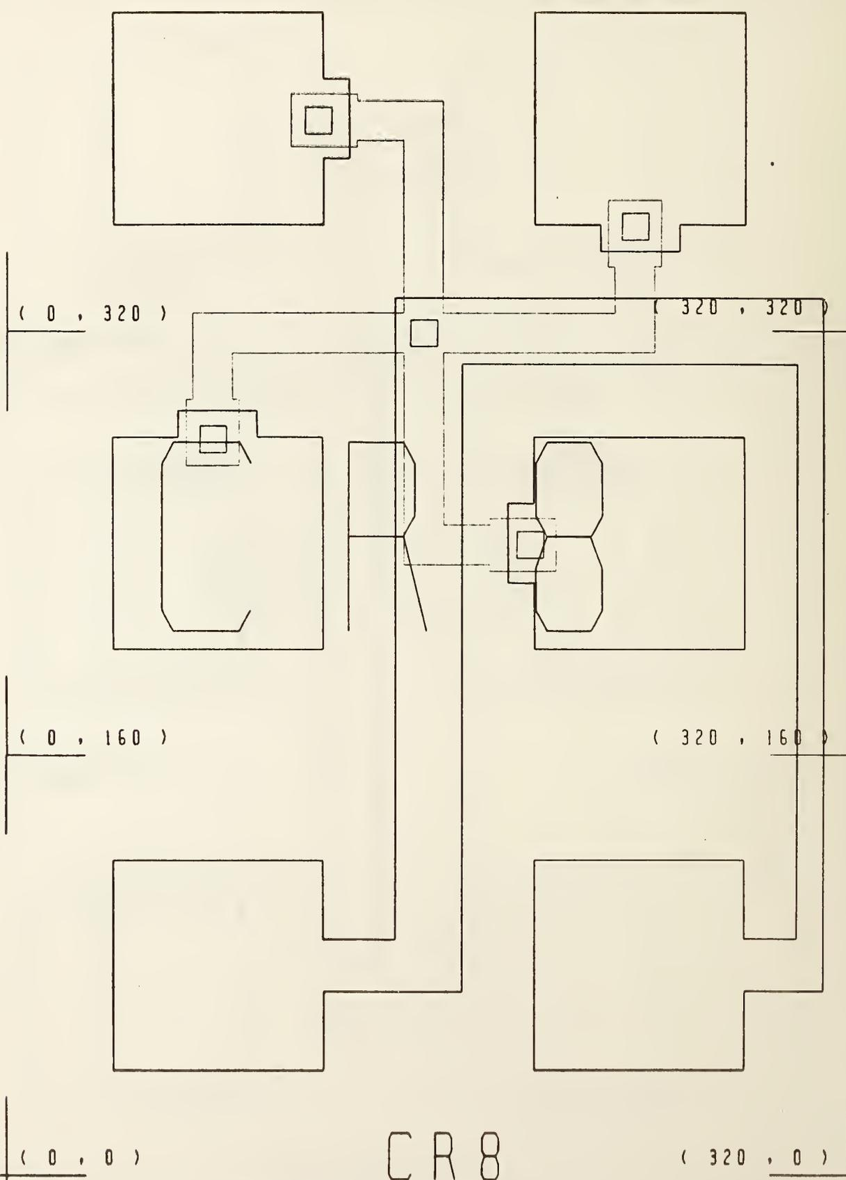
Figure 18. Contact resistor CR-8.
