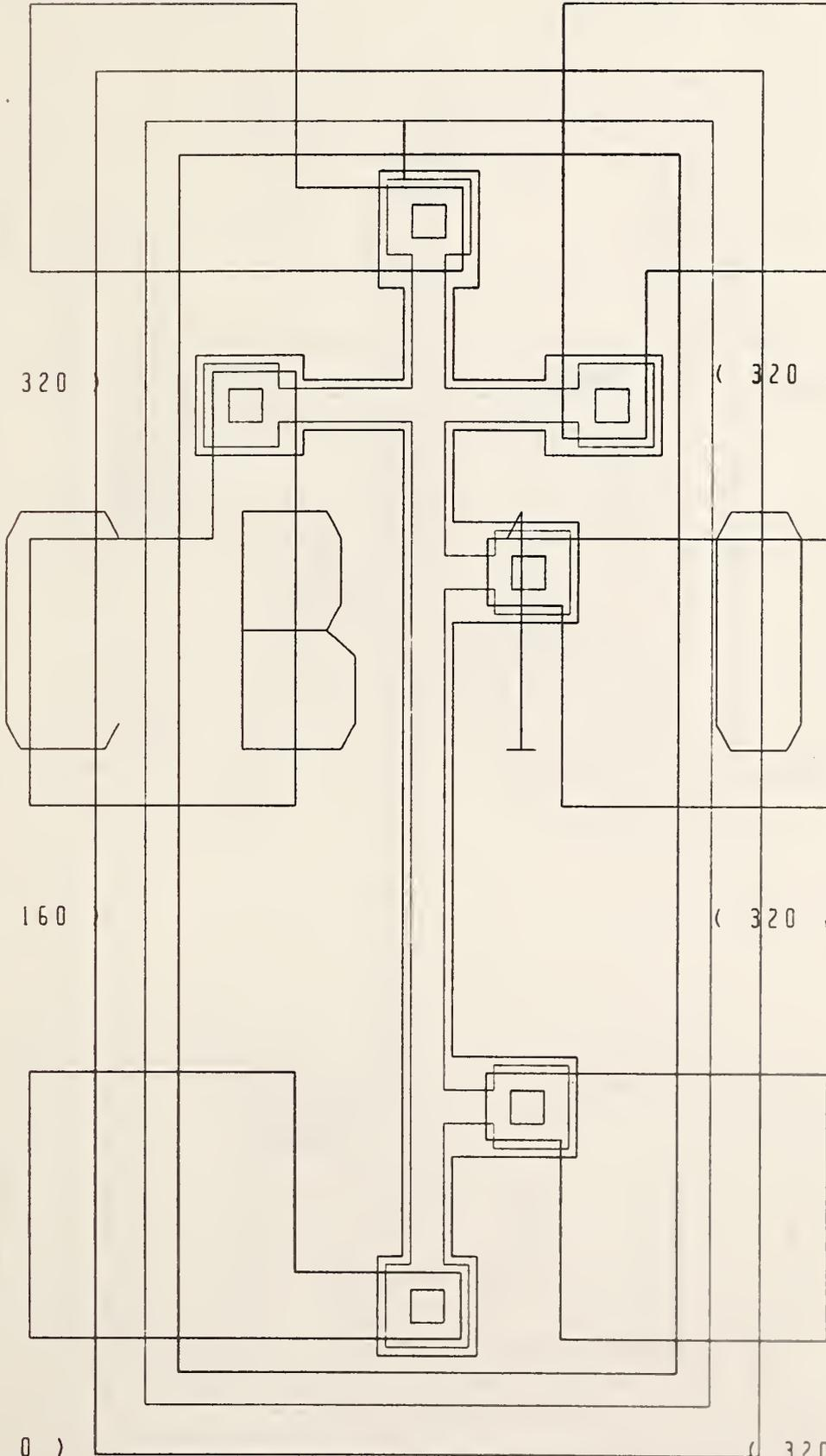
Figure 9. Cross-bridge sheet resistor CB-10.
