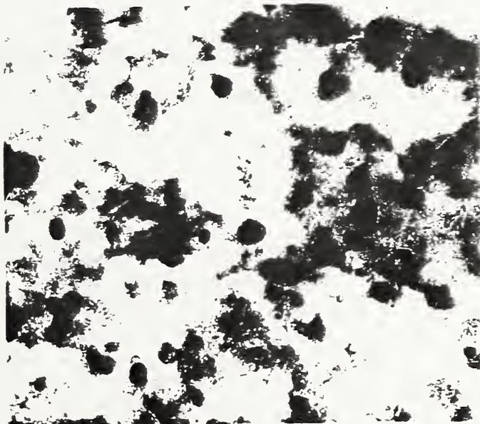
Figure 3 High resolution TEM micrograph of FZN showing faint contrast of precipitates, X200,000.
