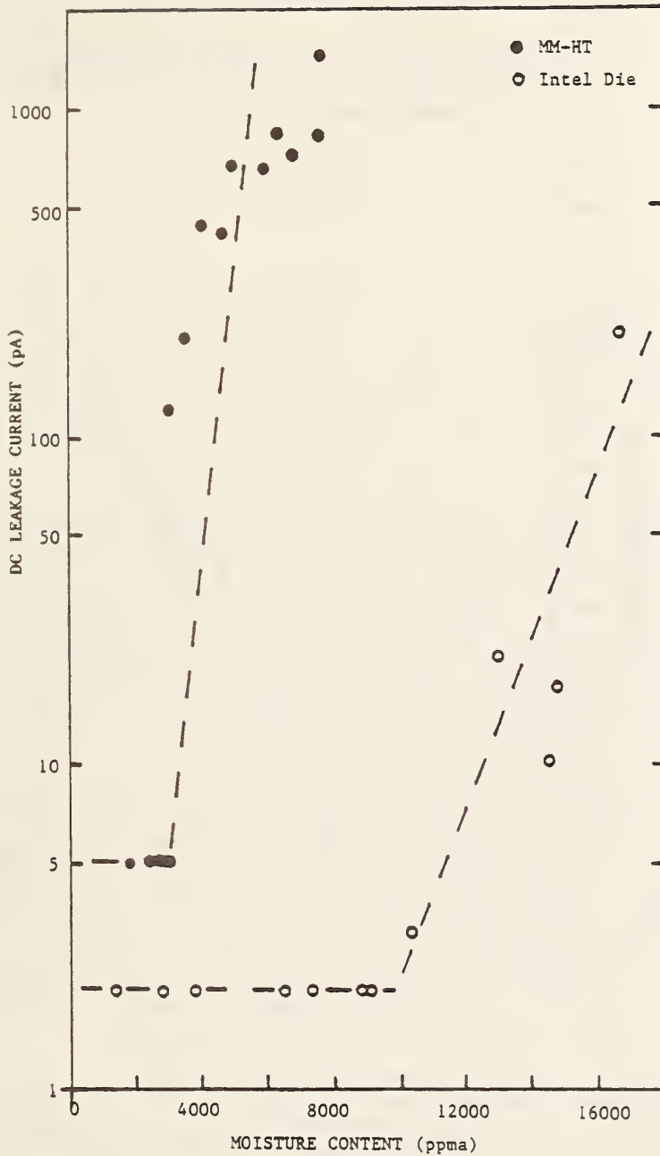
Figure 5 The DC leakage current versus internal moisture (measured by RGA) for the Panametrics MM-HT and the Intel die. The dotted lines are guides for the eye. The lowest current points for each die were actually fluctuating around zero. All such points were plotted at the measured noise level for graphical clarity.
