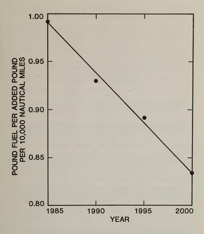
Figure E-1. Sensitivity of Incremental Fuel Consumption to Increased Weight, 1985-2000
