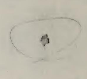
Figure 4. Typical delaminated blister of restoration coatings
