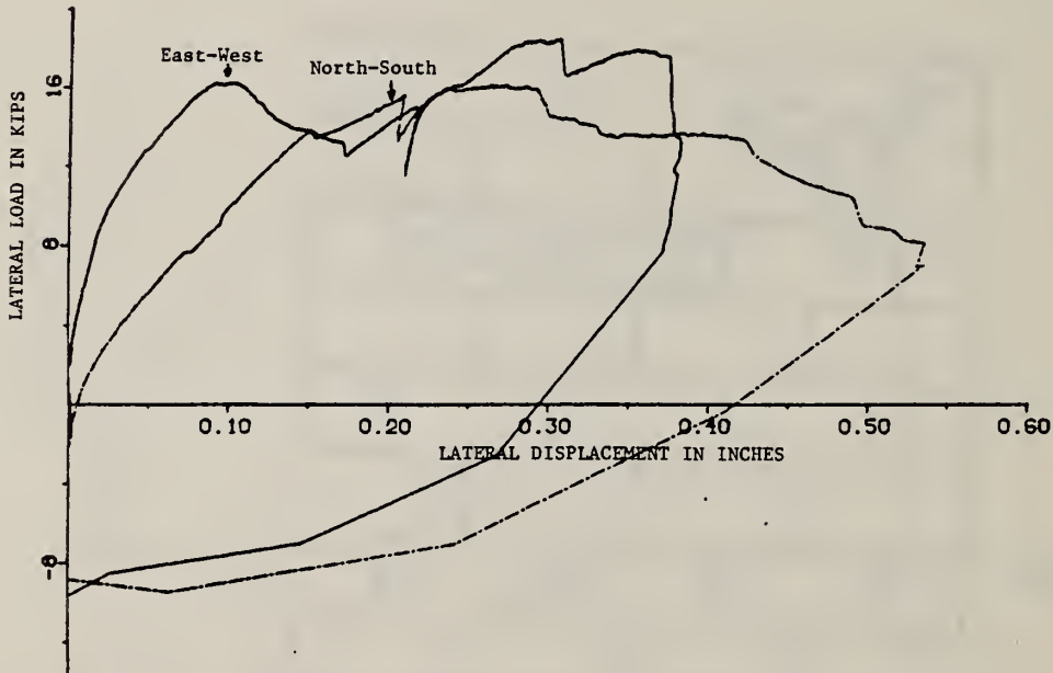
Figure 6.99. Lateral load versus wall displacement for wall C5
