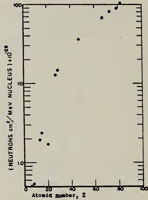
Fig. 31. Absolute neutron yield as a function of atomic number. The neutron yield from calcium ( Z = 20 ) is particularly low in comparison with the other elements because its (\gamma, n) threshold is high compared to the mean energy of the giant resonance.
