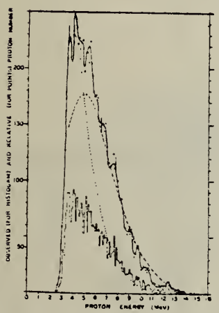
Fig. 6. Energy distribution of total observed protons and calculated distributions by the statistical theory from P^{31} . Full line: Observed spectrum smoothed out by the method of Ferreira and Valoshek. Broken line: Calculated spectrum using w = C \exp[2\sqrt{0.52E}] \text{ MeV}^{-1} Dotted line: Calculated spectrum using w = C \exp[2\sqrt{2.42E}] \text{ MeV}^{-1} . Each curve is normalized to best fit to experimental points.
