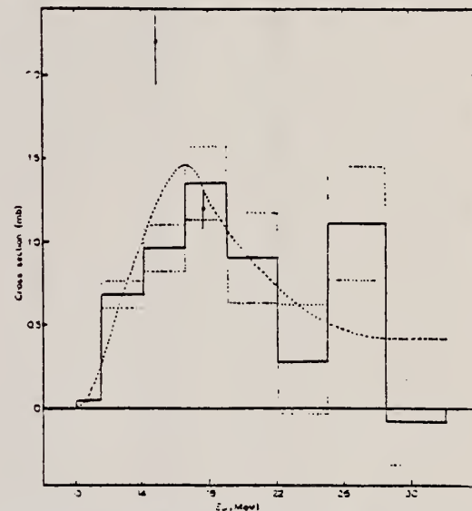
Fig. 6(a). The \text{Li}^7(p, \text{He}^6) excitation curve. The dotted smooth curve was derived from the solid curve of fig. 5. The dotted portions of the histogram indicate the magnitudes of the standard deviations. The two points with error bars in (a) represent the results of Titterton and Brinkley 1) obtained for \gamma radiation of energy 14.8 and 17.4 MeV.
