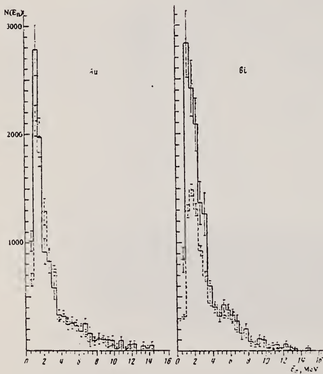
FIG. 3. Photoneutron energy spectra from Rh, Ta, Au, and Bi for irradiation of the samples by bremsstrahlung with maximum energy E_{\gamma \text{ max}} = 20 (dashed line) and 28.5 (solid line) MeV for angles \theta with maximum neutron yield. For each nucleus the histograms given for E_{\gamma \text{ max}} = 20 and 28.5 MeV have been combined in the interval E_n = 4-4.5 MeV.
