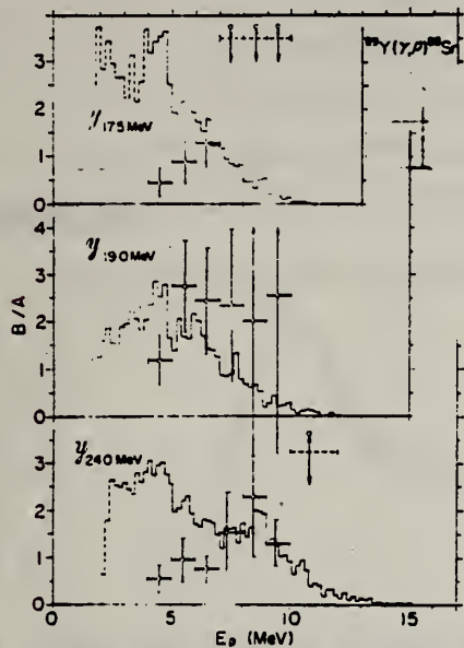
Fig. 4. Energy dependence of the anisotropic factor B/A of the angular distributions for photoprotons from ^{89}\text{Y} . A sign \frac{-}{+} indicates that B/A is too large to plot the figure.
