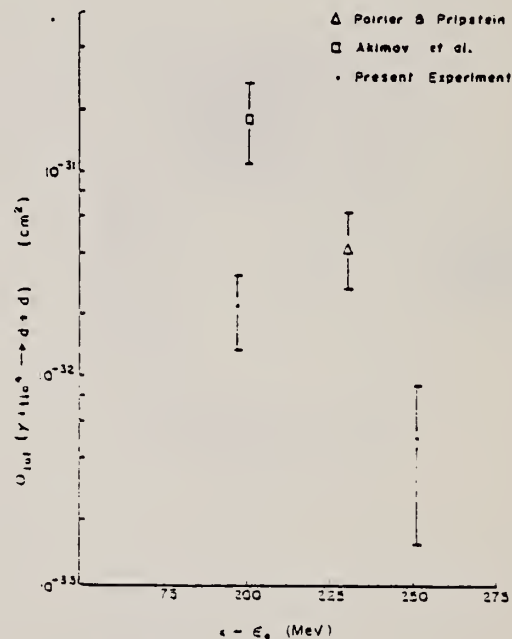
FIG. 5. The high-energy experimental cross sections for \gamma + \text{He}^4 \rightarrow d + d . The cross section due to Akimov et al. and the upper limit of Poirier and Pripstein were inferred from their measurements of the inverse cross section \sigma(d + d \rightarrow \text{He}^4 + \gamma) . Threshold energy \epsilon_0 = 23.9 MeV.
