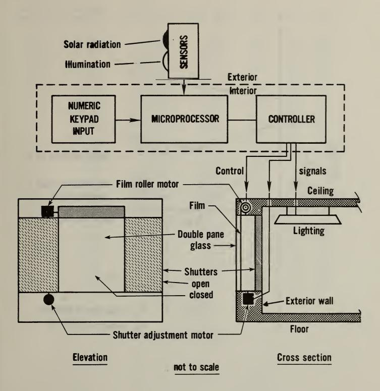
Figure 1. Schematic of typical control systems
