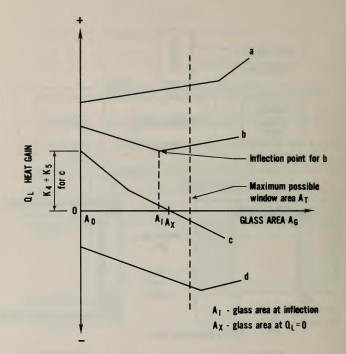
Figure 2. Heat gain  $\textbf{Q}_L$  as a function of glass area  $\textbf{A}_G$
