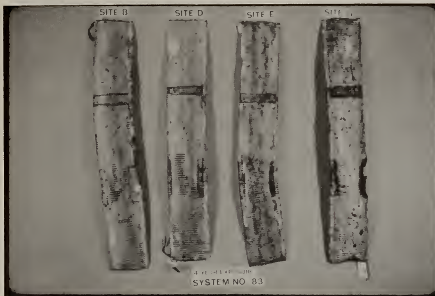
Figure 34. Outer Shield: System 83, Sites B, D, E, and G, left to right, exposed for four years. Severe corrosion at the window area on the specimen from Site G.
