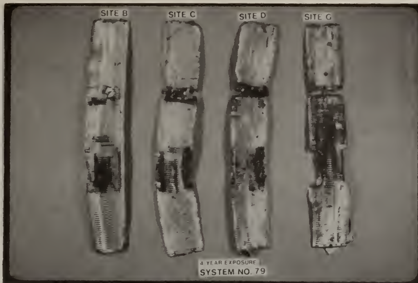
Figure 26. Outer Shield: System 79, Sites B, C, D, and G, left to right, exposed for four years. Dark areas indicate corrosion with severe corrosion at the window and ring areas.
