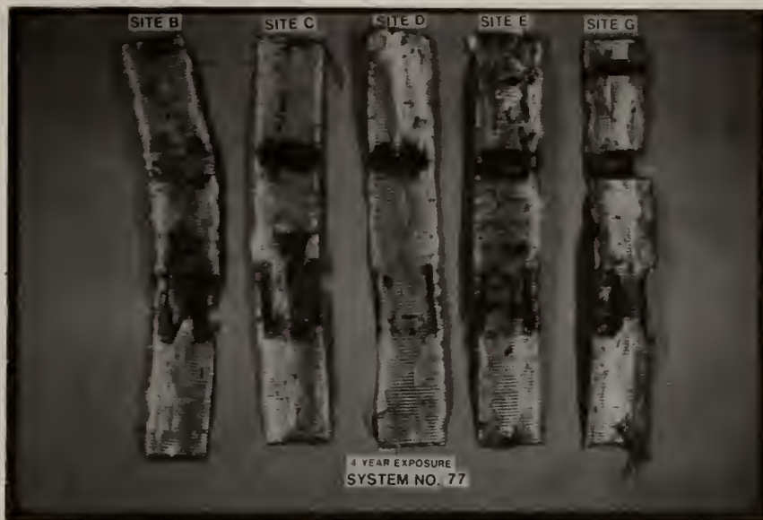
Figure 22. Outer Shield: System 77, Sites B, C, D, E, and G, left to right, exposed for four years. Dark areas indicate corrosion with severe corrosion at the window and/or ring areas on all the specimens.
