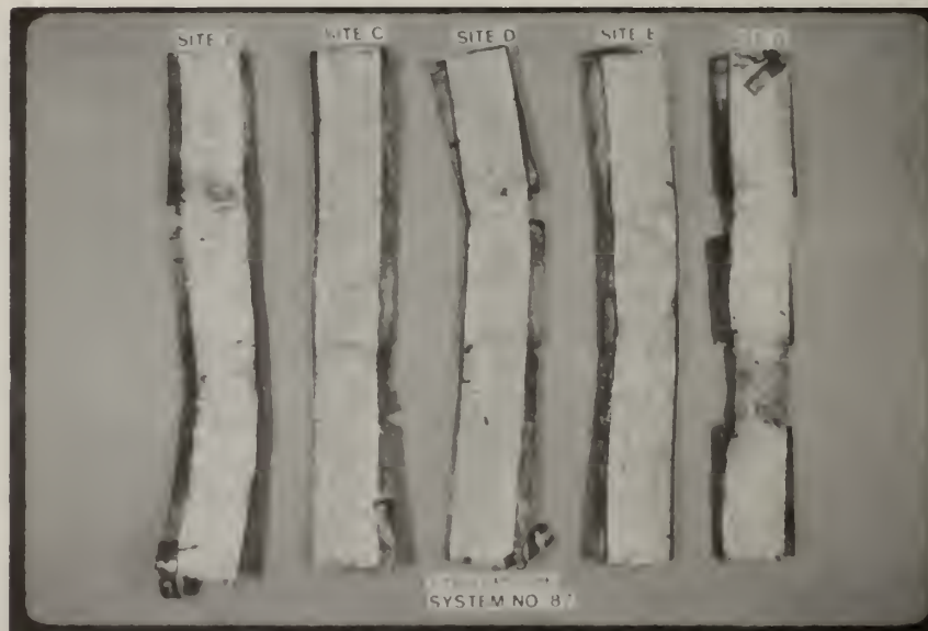
Figure 41. Inner Shield: System 87, Sites B, C, D, E, and G, left to right, exposed for four years. The specimen from Site G was severely degraded.
