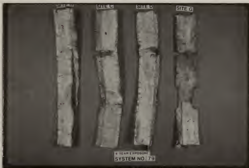
Figure 27. Inner Shield: System 79, Sites B, C, D, and G, left to right, exposed for four years. Severe degradation on the specimen from Site G and the ring area on the specimen from Site C.
