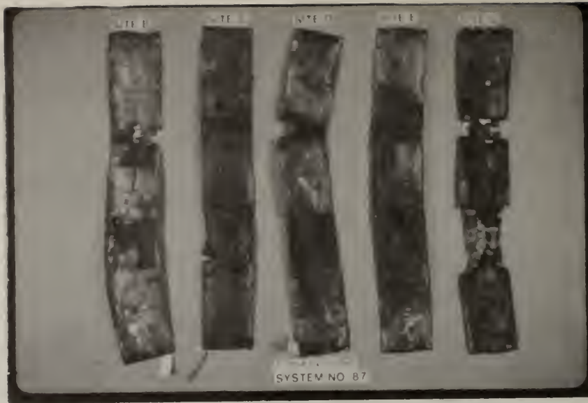
Figure 40. Outer Shield: System 87, Sites B, C, D, E, and G, left to right, exposed for four years. Dark areas indicate corrosion with severe corrosion at window and ring areas on specimens from Sites B, C, D, and G.
