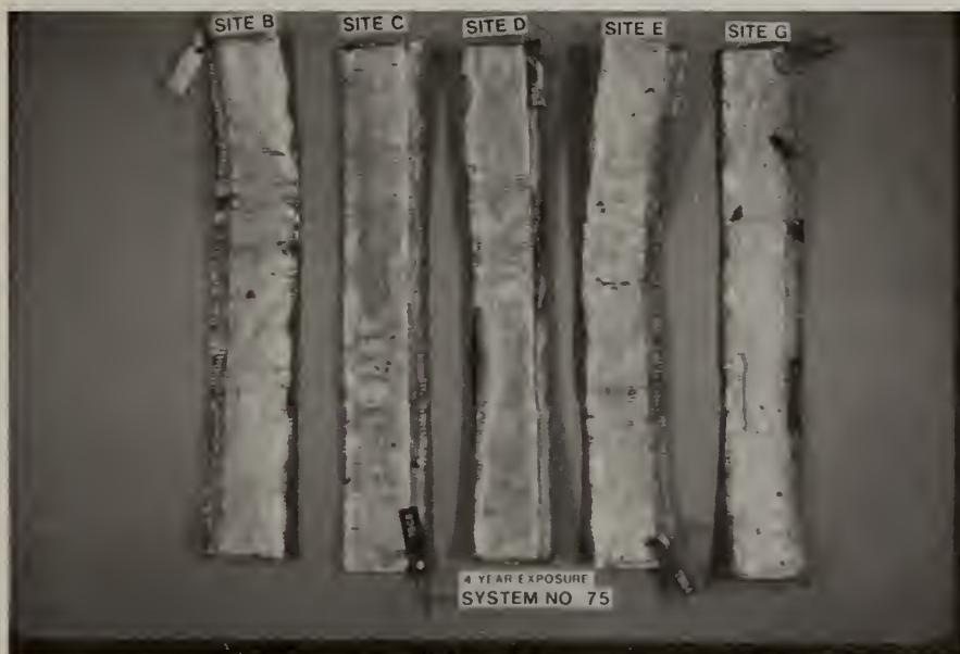
Figure 19. Inner Shield: System 75, Sites B, C, D, E, and G, left to right, exposed for four years. Specimens were unaffected by corrosion.
