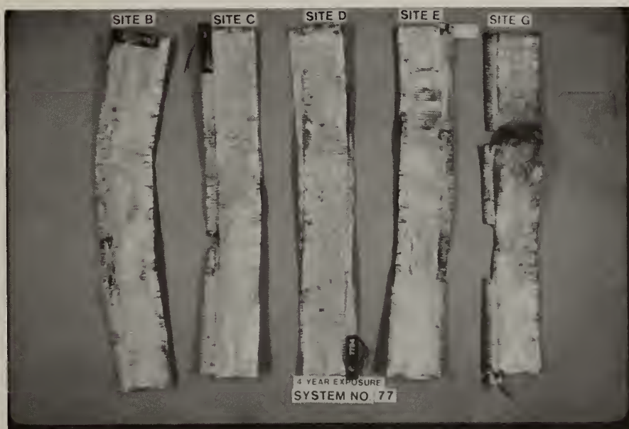
Figure 23. Inner Shield: System 77, Sites B, C, D, E, and G, left to right, exposed for four years. Severe degradation of the window and ring area on the specimen from Site G.
