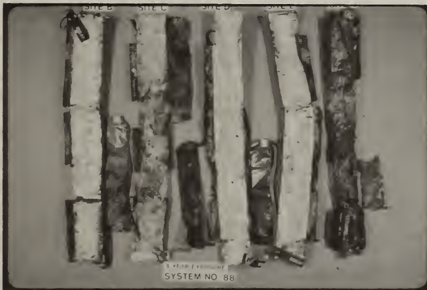
Figure 43. Inner Shield: System 88, Sites B, C, D, E, and G, left to right, exposed for four years. Coupling this system to copper accelerated degradation on the specimens from Sites C and G.
