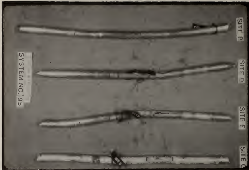
Figure 4. Outer Shield: System 95, Sites B, D, E, and G, top to bottom, exposed for two years. Degradation at the window and ring areas on the specimen from Site G.
