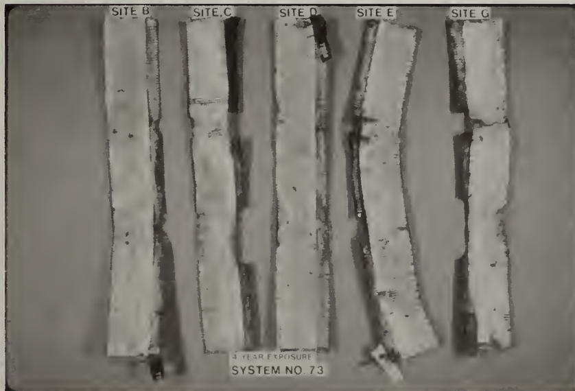
Figure 15. Inner Shield: System 73, Sites B, C, D, E, and G, left to right, exposed for four years. Severe degradation at the window and ring areas on the specimen from Site G.
