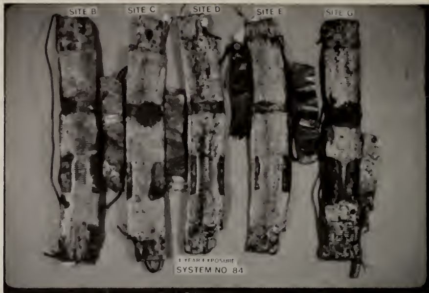
Figure 36. Outer Shield: System 84, Sites B, C, D, E, and G, left to right, exposed for four years. Coupling this system to copper accelerated corrosion at the window and ring areas.
