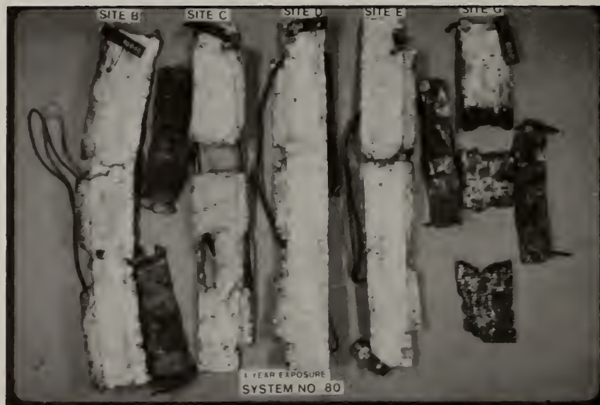
Figure 29. Inner Shield: System 80, Sites B, C, D, E, and G, left to right, exposed for four years. Coupling this system to copper accelerated the degradation on all specimens.
