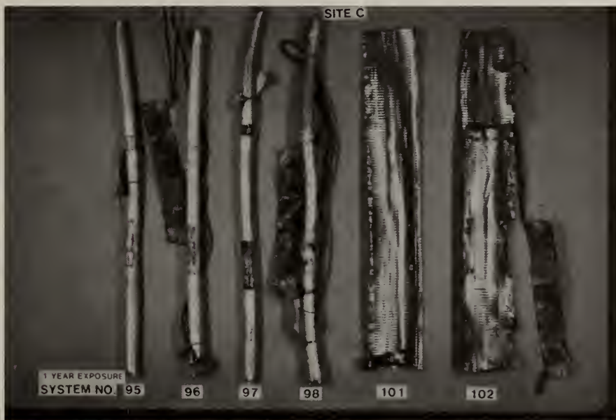
Figure 3. Outer Shield: Systems 95, 96, 97, and 98, Inner Shield: Systems 101 and 102, left to right, exposed at Site C for one year. Severe corrosion on Systems 96, 98, and 102 at window and/or ring areas.
