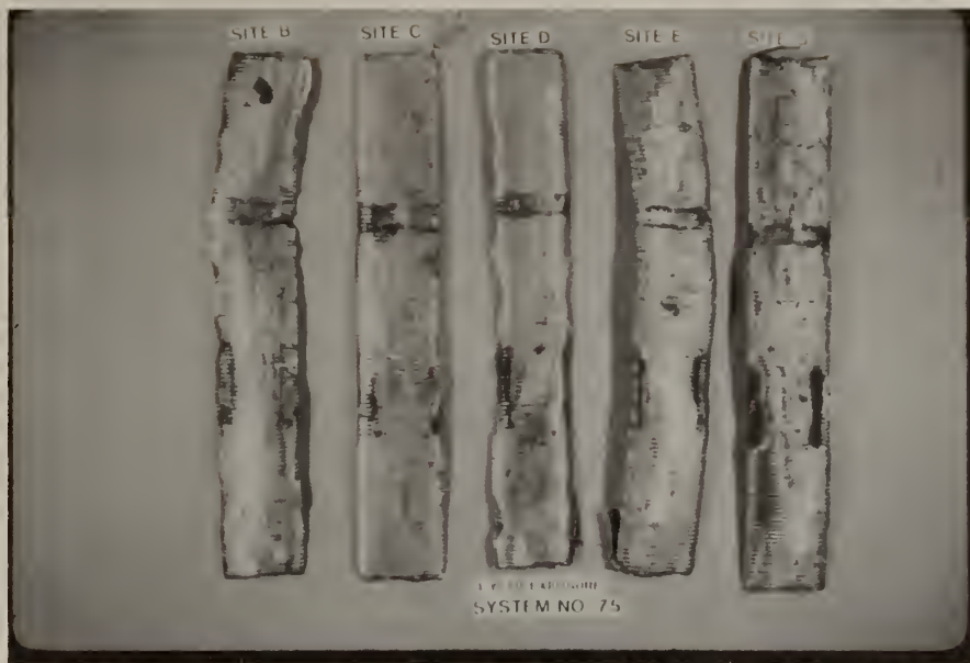
Figure 18. Outer Shield: System 75, Sites B, C, D, E, and G, left to right, exposed for four years. Dark areas indicate corrosion at the window and ring areas on the specimen from Site G.
