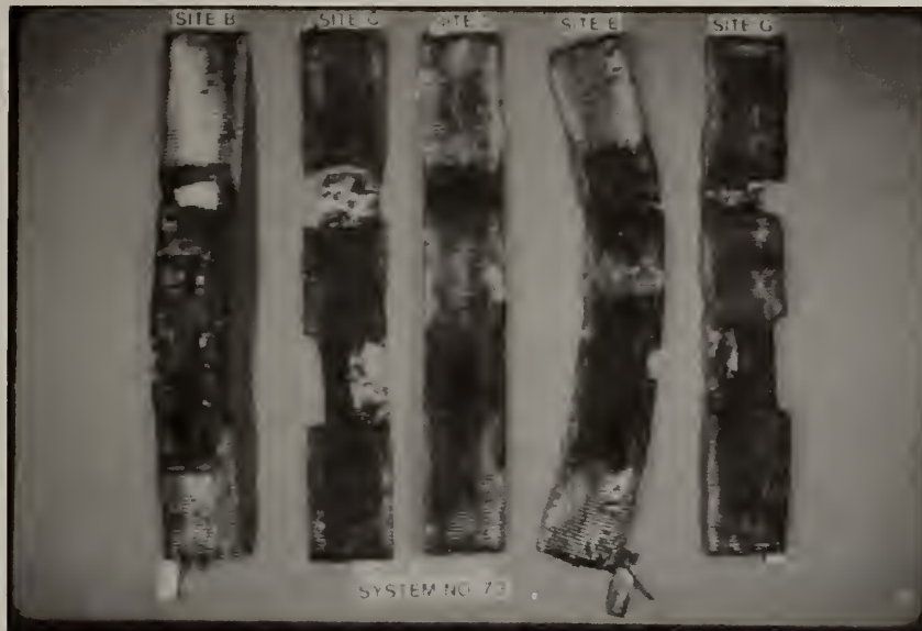
Figure 14. Outer Shield: System 73, Sites B, C, D, E, and G, left to right, exposed for four years. Dark areas indicate corrosion with severe corrosion at the window and rings on specimens from Sites B, C, E, and G.
