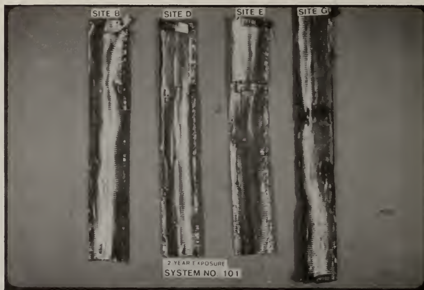
Figure 9. Inner Shield: System 101, Sites B, D, E, and G, left to right, exposed for two years. Dark areas indicate corrosion at the window and ring areas on specimens with severe corrosion on the specimen from Site G.
