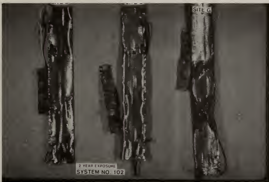
Figure 11. Inner Shield: System 102, Sites B, E, and G, left to right, exposed for two years. Coupling this system to copper accelerated corrosion on specimens at window and ring areas, with severe corrosion on the specimen from Site G.
