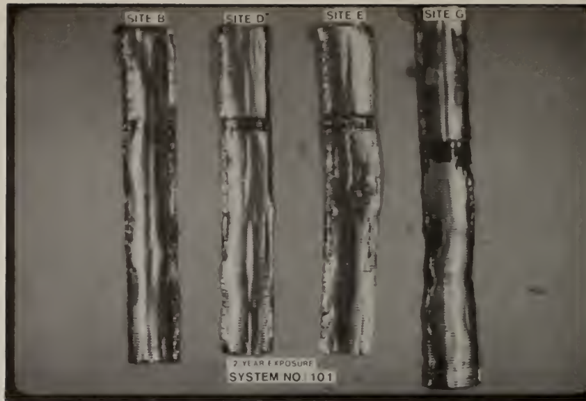
Figure 8. Outer Shield: System 101, Sites B, D, E, and G, left to right, exposed for two years. Dark areas indicate corrosion at the window and ring areas.
