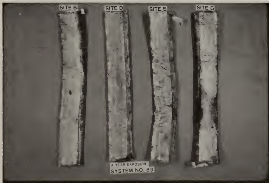
Figure 35. Inner Shield: System 83, Sites B, D, E, and G, left to right, exposed for four years. Dark areas indicate severe degradation at the window area on the specimen from Site G.
