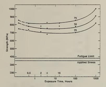
Fig. 5. Strength degradation diagram for yttria-doped, hot-pressed silicon nitride (NCX 34). Temperature of exposure 1200 °C; applied stress 350 MPa.
