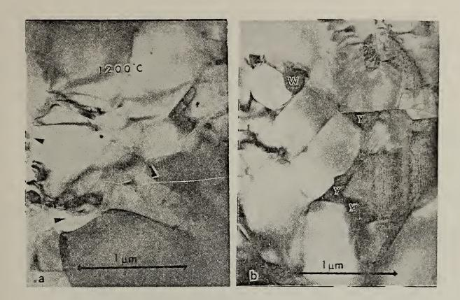
Fig. 9. Transmission Electron Micrographs of hot-pressed silicon nitride: (a) NC 132, (b) NCX 34. The arrows in (a) indicate boundries within the foil that have cracked as a result of creep. The yttria doped material (b) gives no evidence for crack formation. Y indicates the yttria rich phase; W indicates the tungsten rich phase.
