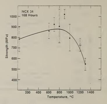
Fig. 2. Strength of NCX 34 after exposure to test temperature for 168 hours. Specimens were exposed and tested at temperature without cooling to room temperature.
