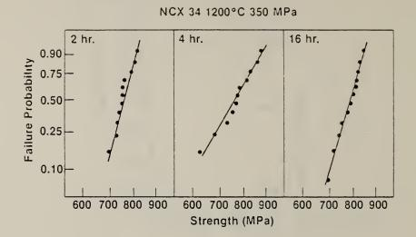
Fig. 4. Strength distribution after 2, 4, and 16 hours of exposure at 1200 °C at a sustained load of 350 MPa.
