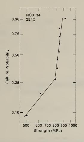
Fig. 3. Initial room temperature strength distribution of yttria-doped, hot-pressed nitride.
