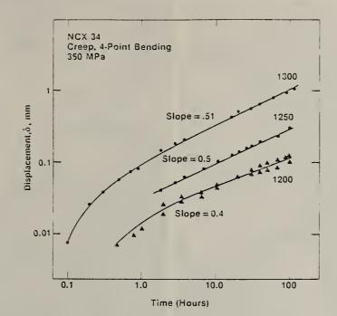
Fig. 7. Creep behavior of NCX 34 at 350 MPa maximum fiber stress. Center point displacement as a function of time.
