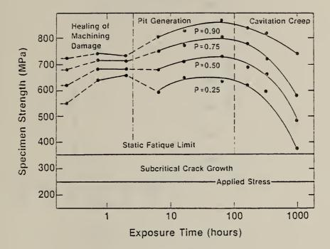
Fig. 1. Strength degradation diagram for magnesia-doped, hot-pressed silicon nitride (NC 132). Temperature of exposure 1200 °C; applied load 250 MPa.
