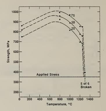
Fig. 6. Effect of temperature on the strength of NCX 34 which is subject to a sustained load of 350 MPa for 100 hours.
