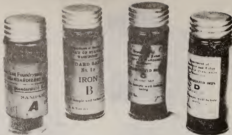
The first four SRMs certified by NBS in 1906 were these four cast iron compositional standards prepared in cooperation with the American Foundrymen's Society
