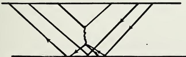
Poor resolution. The strong backward signal mask the weak diffracted signal.
