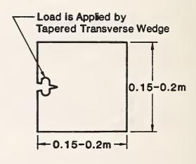
Figure 1. Typical Small Scale Crack Arrest Specimens.
