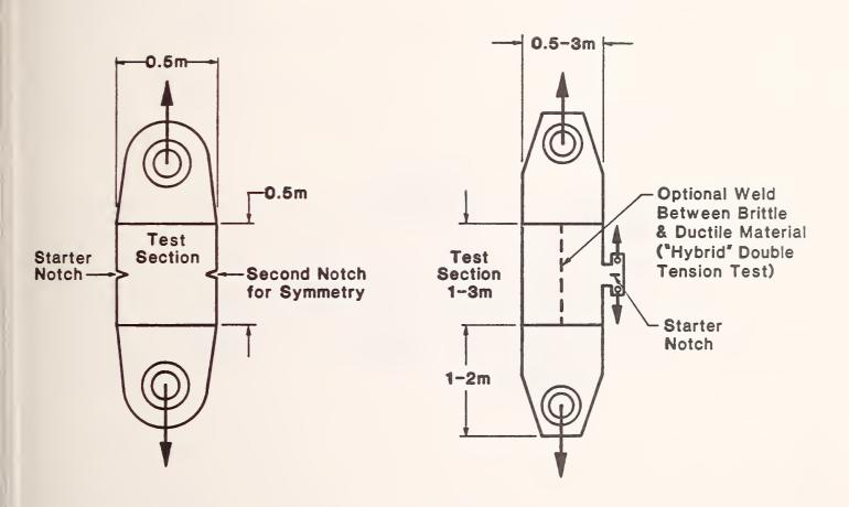
Fig. 2. Large Scale Crack Arrest Specimens.
