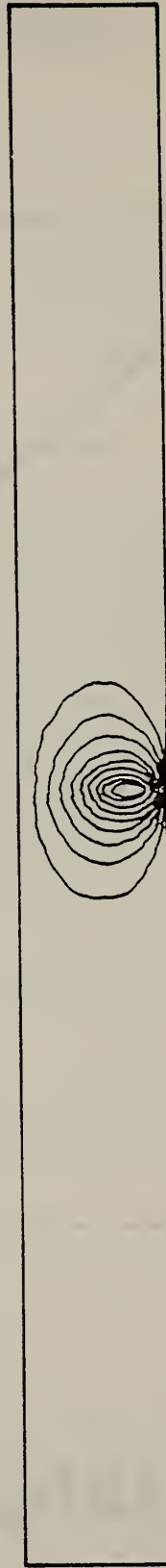
Fig. 4. Equipotential lines between parallel plates for the nonuniform interfacial surface charge density, \rho_2(z) , and with V = 0 .
