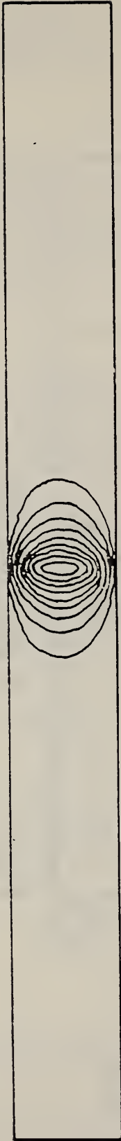
Fig. 3. Equipotential lines between parallel plates for a uniform interfacial surface charge density, \rho_1(z) , and with no voltage applied to the plates, V = 0 .
