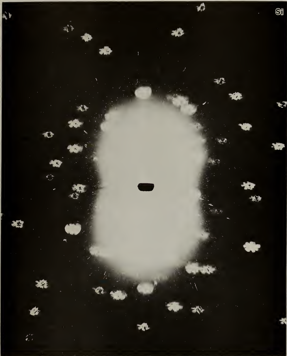
Figure 2 Synchrotron white beam transmission topographs of an electron beam melted and resolidified spot on a 111 surface of Si. Notice the residual stress pattern which extends outward from the weld spot.
