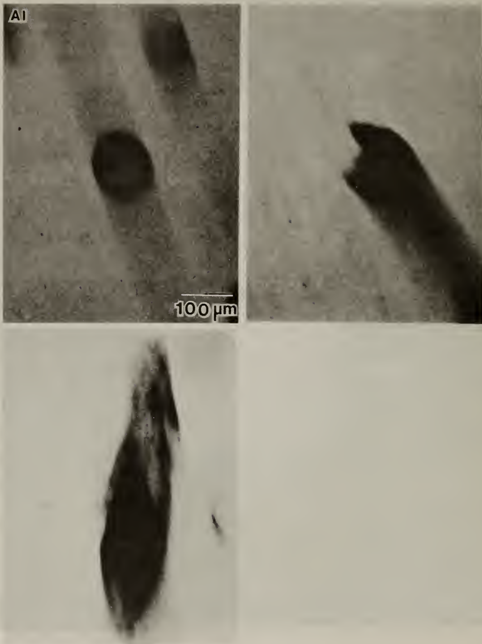
Figure 3 Synchrotron white beam topographs of single Al powder particles solidified with large undercooling. The top left shows a particle which is a single crystal and which had only one nucleus. The top right shows a particle having two grains while the bottom left shows a deformed particle.
