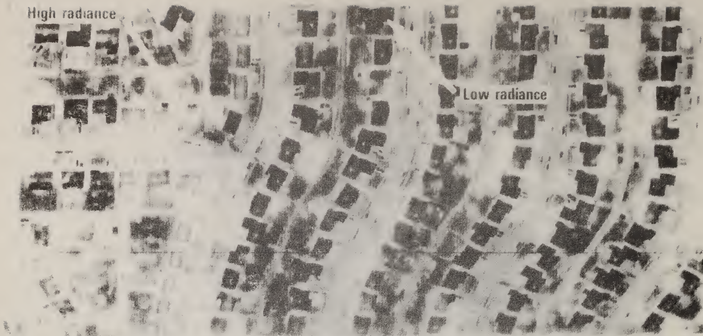
Figure 3.2 An aerial infrared photograph of a large number of residential roofs (provided by Texas Instruments)
