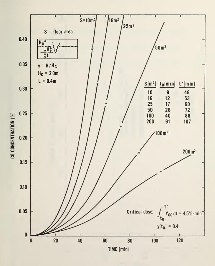
Figure 9. Theoretical results for a chair smoldering in rooms of various volume
