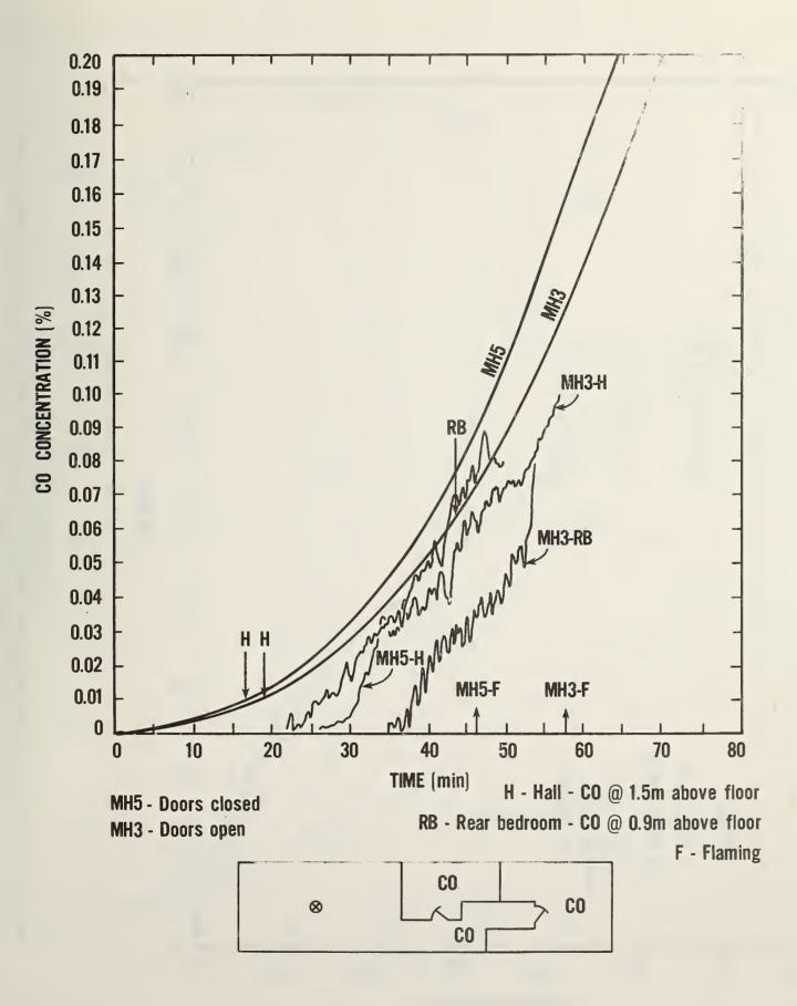
Figure 7. Calculated and measured CO concentrations for a chair smoldering in a closed mobile home. So Chair location
