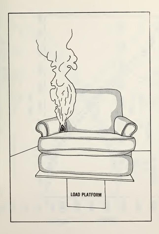
Figure 3. Sketch from a photograph of a smoldering smoke plume
