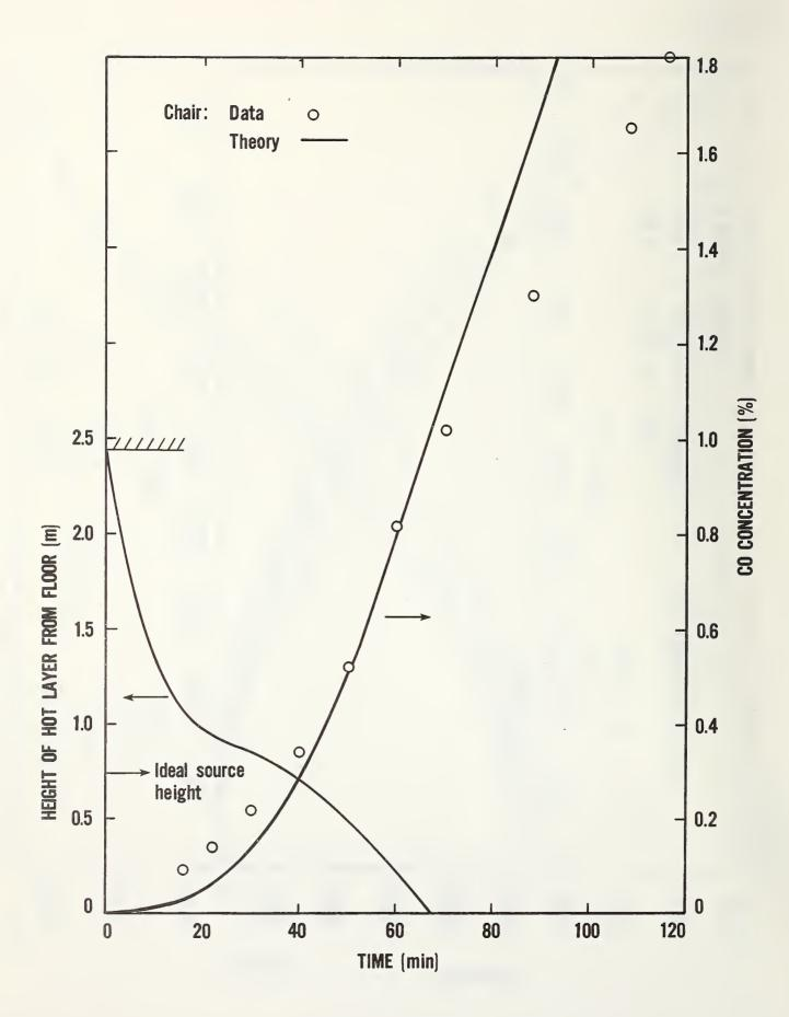
Figure 6. Calculated and measured results for a chair smoldering in a closed room
