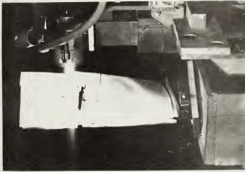
Thermal spraying of fan blade shroud
