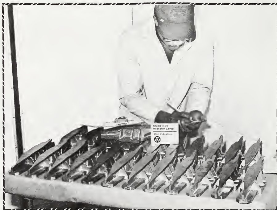
Figure 24. Grumman F-14A Fuselage Braces Made from Ti-6Al-6V-2SN Powder
