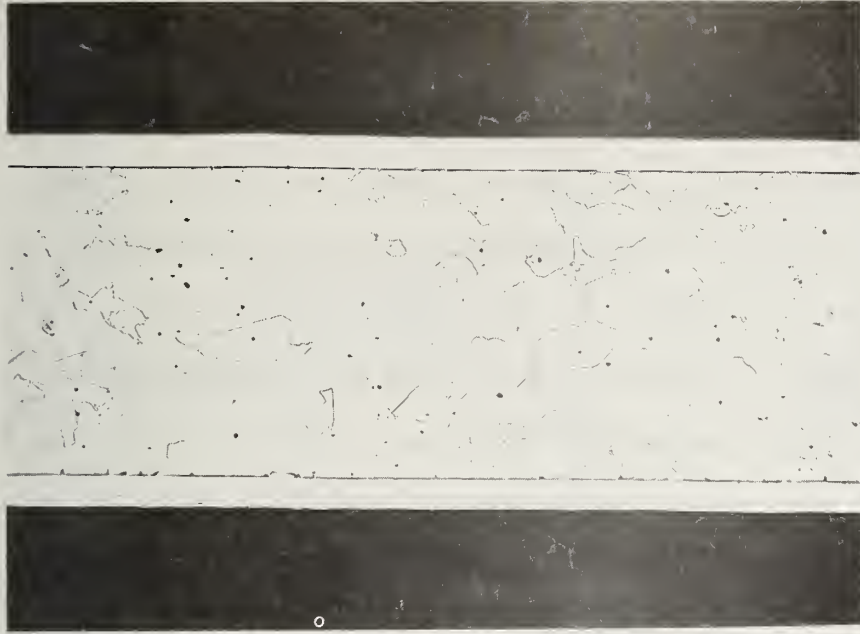
Figure 5 Dilex chromized sheet Nital etch x 50
