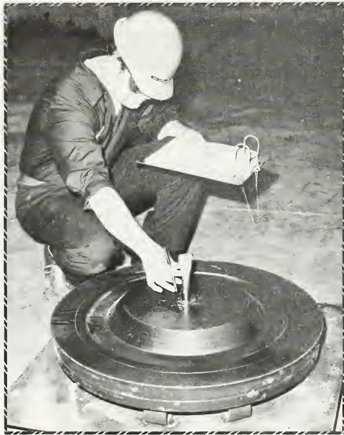
Figure 15. Large P/M Turbine Disk Made Using Metal Container.
