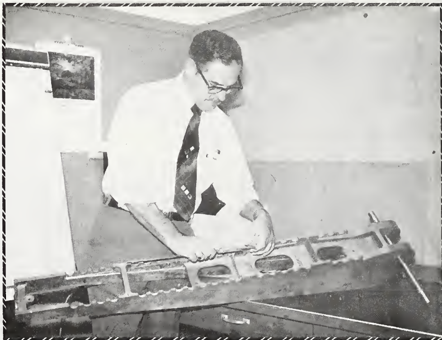
Figure 20. The Northrop F-18 Arrestor Hook Support Fitting P/M Titanium Part.
