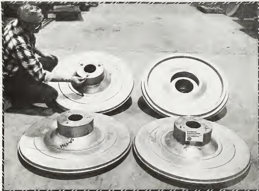
Figure 16. 32-Inch P/M Turbine Disk Made Using Metal Container.
