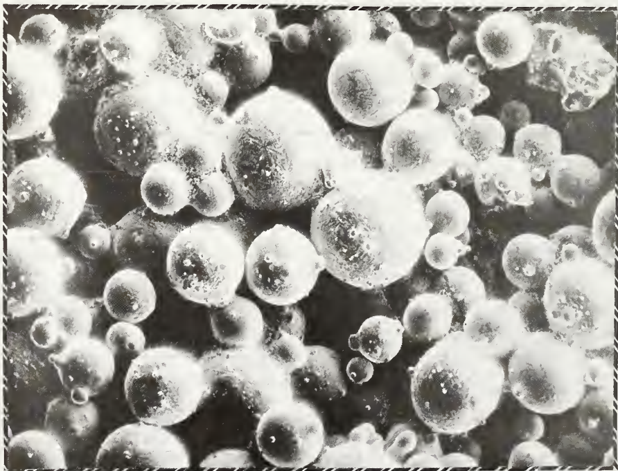
Figure 2. Argon Gas-Atomized Powder.
