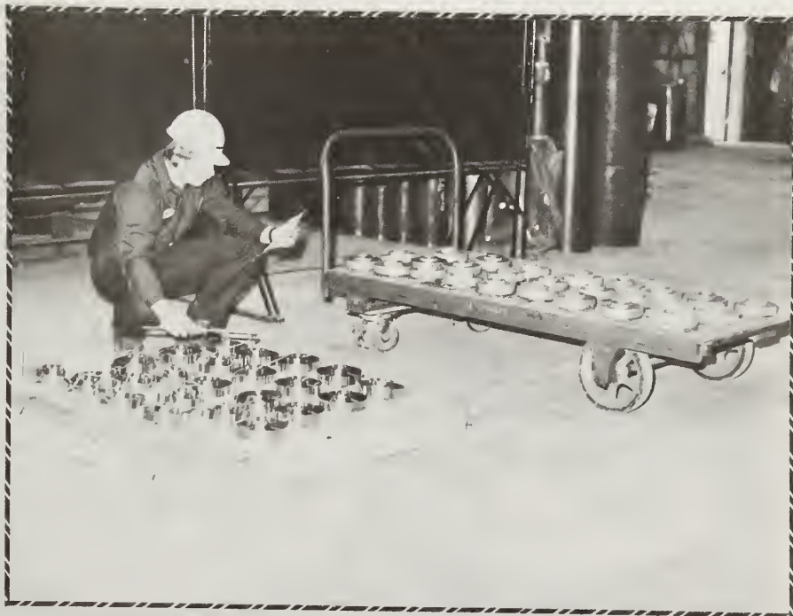
Figure 14. Small P/M Turbine Disks Made Using Metal Container.
