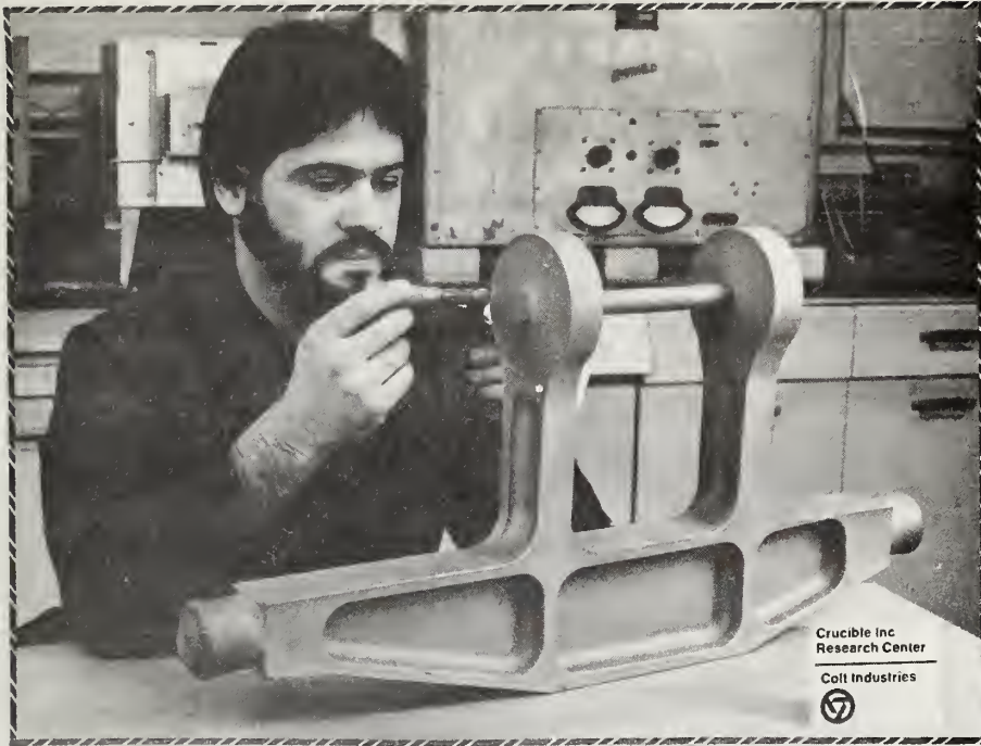
Figure 21. The Boeing 747 Walking Beam Support Fitting P/M Titanium Part.
