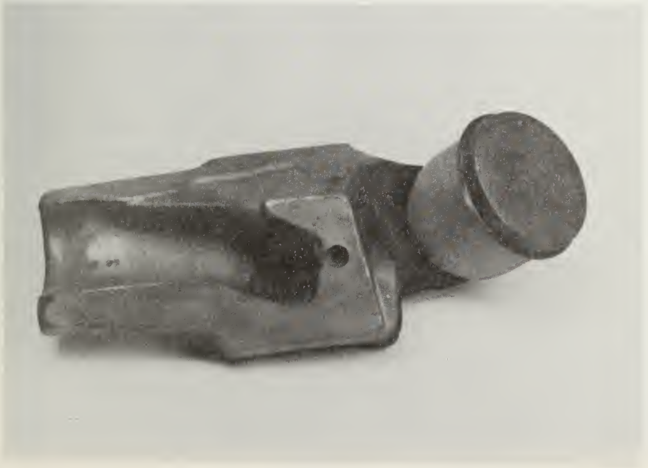
Figure 9 Head Section Of Figure 1 With Cup Packed, Ready For Boronizing.
