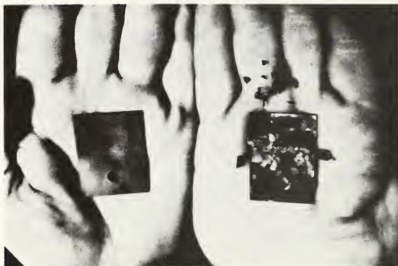
Figure 30. Corrosion Resistance of New Chromium-Free Alloy Compared to That of Ordinary Low Carbon Steel
