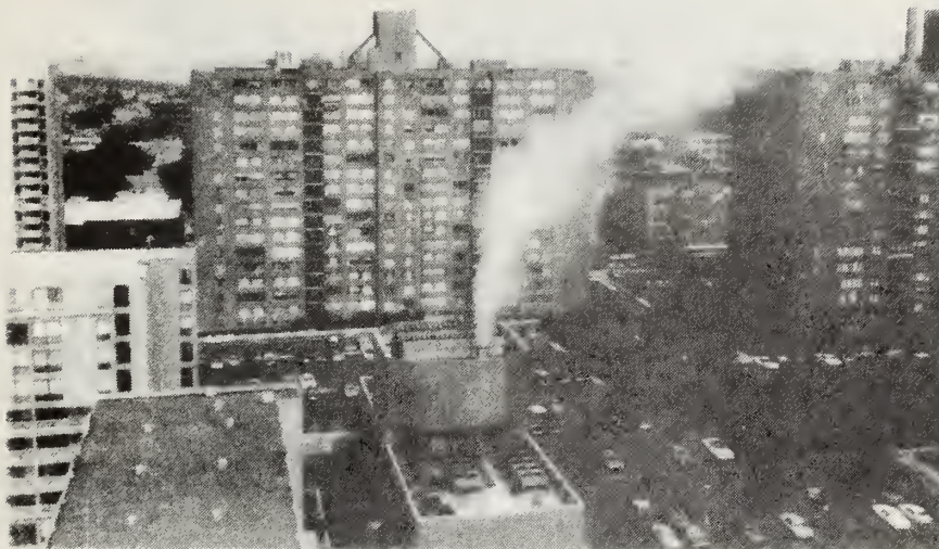
Figure 10.9 Diesel engine exhaust plume with 2-4 mph (0.9 - 1.8 m/s) southerly wind. Visibility of the plume was enhanced by means of a smoke bomb dropped into the stack.
