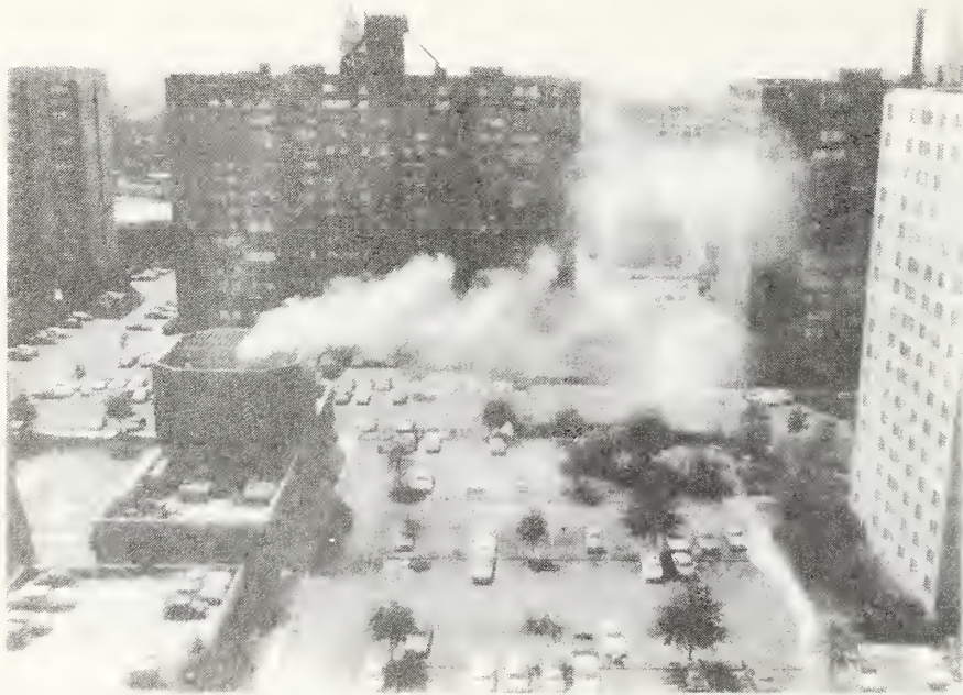
Figure 10.11 Diesel engine exhaust plume with 9-12 mph (4.0-5.4 m/s) southerly wind. Visibility of the plume was enhanced by means of a smoke bomb dropped into the stack.
