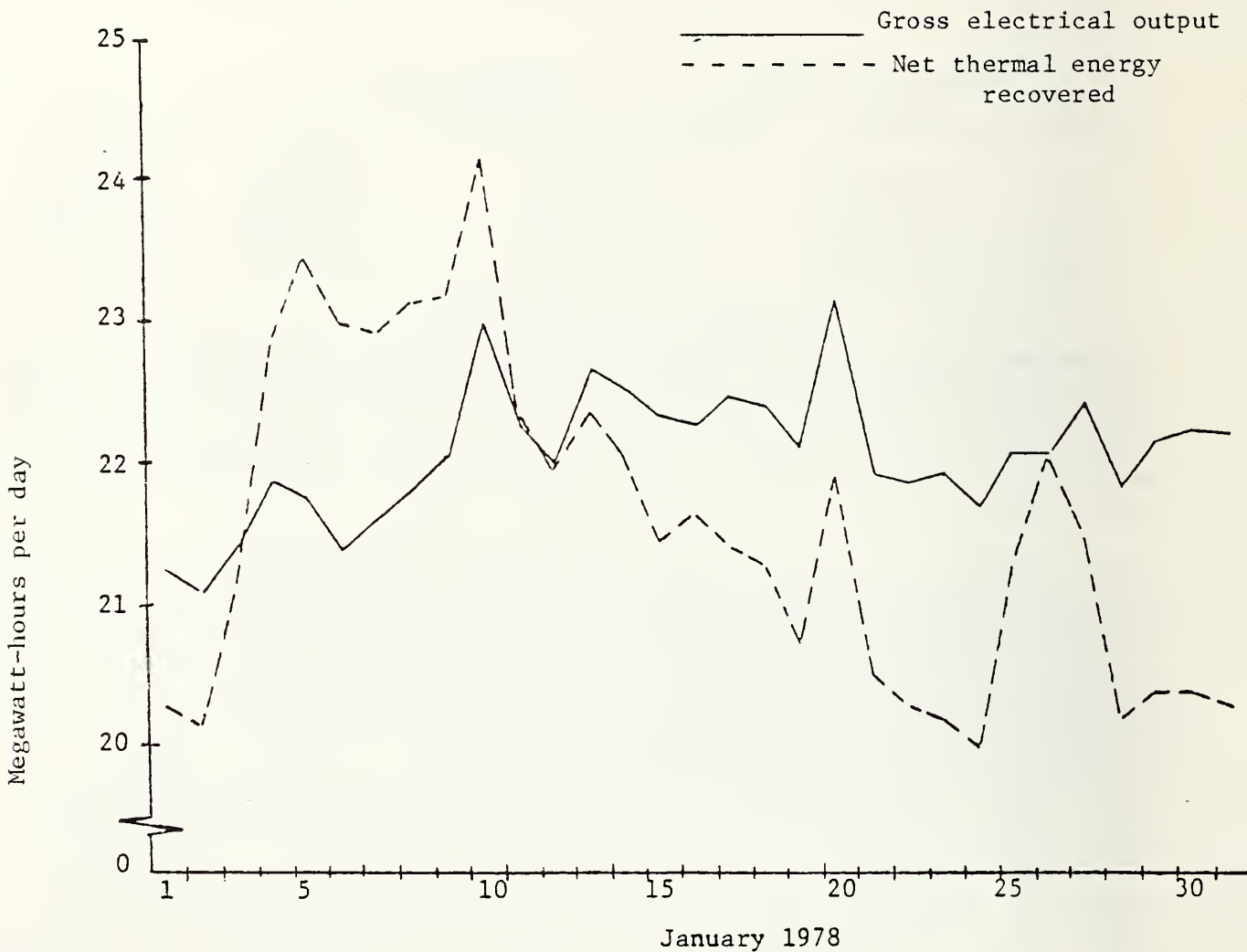
Figure 5.6 Gross electrical output of the three on-line units and net thermal energy recovered from the entire bank of engines. The exhaust gas heat exchangers were cleaned during the period December 26, 1977 through January 3, 1978. On the January 25 and 26, the on-line engines were changed. Two engines with less deposits in their exhaust gas heat exchanger were put on line and consequently a rise in the net thermal energy recovered from the engines is indicated. The overall effects of the deposits in the exhaust gas heat exchangers are reflected in these curves. The jackets and exhaust gas heat exchangers of all five engines were in the PHW loop during the period shown.
