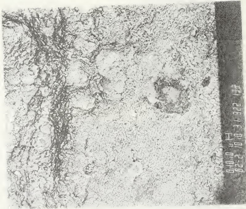
Figure 8.4 Photomicrograph of a replica from the shear lip region at location 8UE. The surface oxidation has removed the fine shear dimpled rupture features in this area. Magnification X250.
