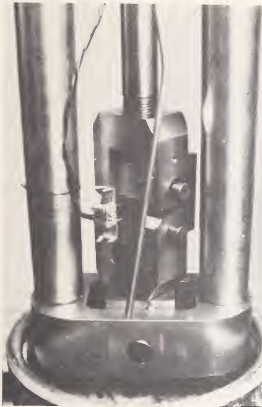
Fig. 1 Low temperature fracture toughness testing apparatus in use at NBS/Boulder.
