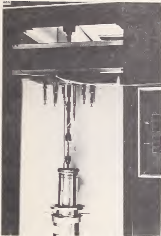
Fig. 4 Low temperature tensile testing apparatus in use at NBS/Boulder.
