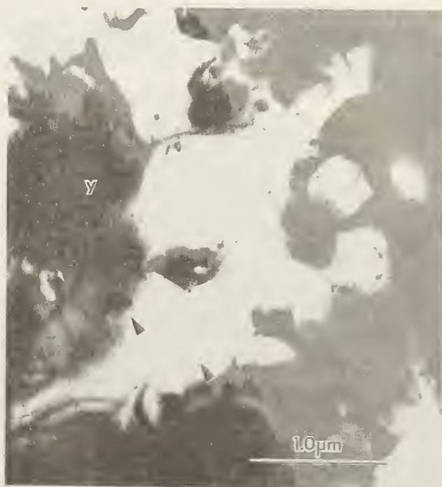
Fig. 3. Material -B- at 750^\circ\text{C} in 5200 Pa after heating for \sim 5 min., showing oxide platelets (arrowed) and reacting yttria phase (Y).
