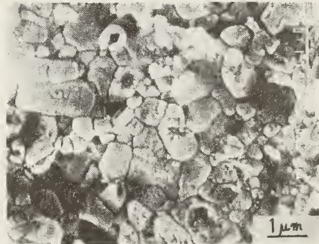
Fig. 10. The fractured surface at 1400°C after etching.
