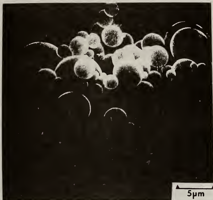
Figure 46. Glass microspheres synthesized in forced draft furnace.
