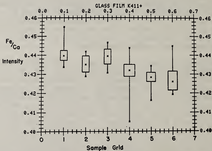
Figure 48. Diagram showing the variability in ratio of Fe to Ca x-ray intensities for six samples analyzed on the electron microprobe.
