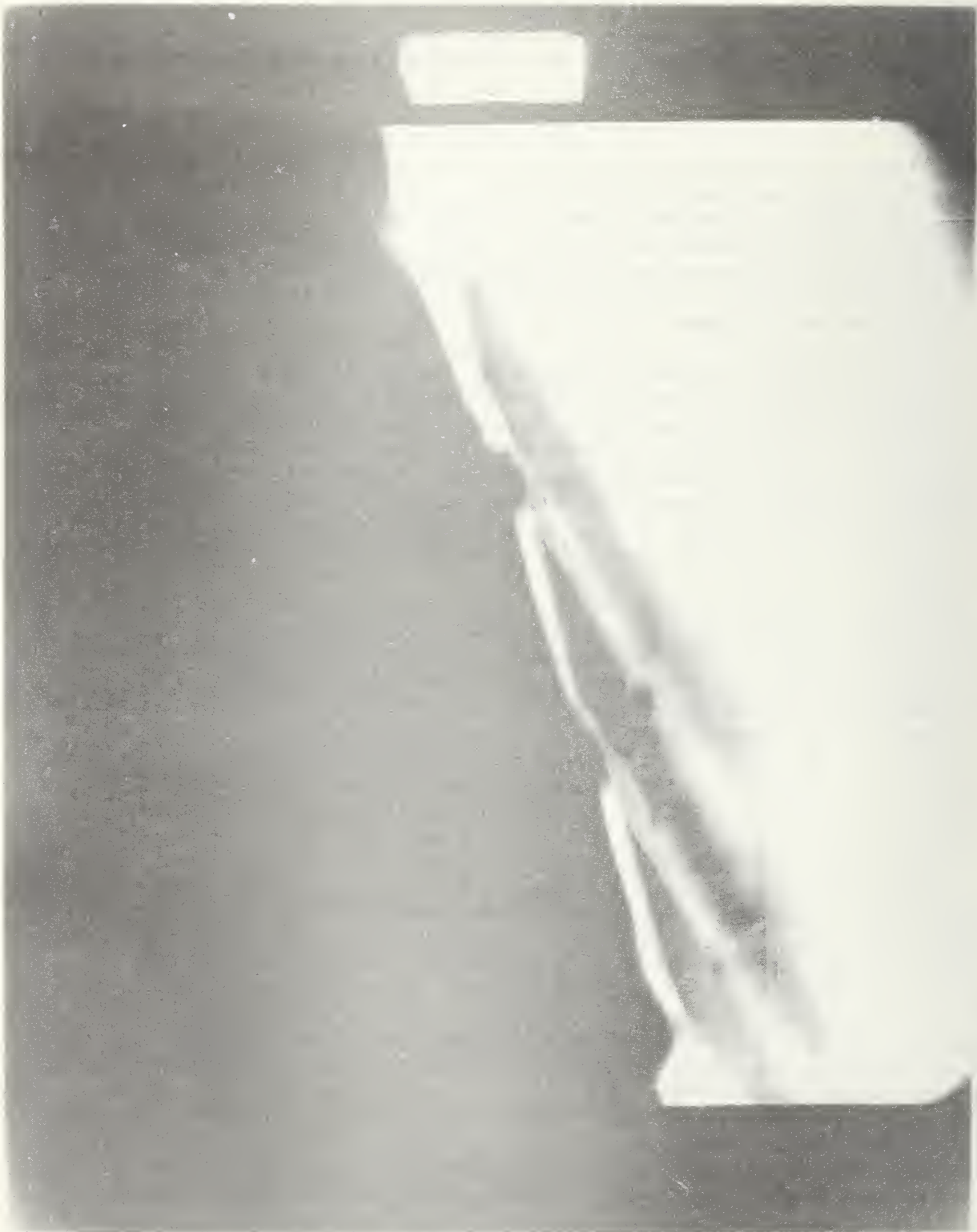
Figure 4.12 Composite secondary electron and EBIC micrograph. The sample was implanted with \text{As}^+ to a dose of 5 \times 10^{15}/\text{cm}^2 at 75 keV and 7-deg tilt, then annealed at 1000^\circ\text{C} for 30 min. The oxide shapes are seen in secondary electron mode, while the bright regions under the implanted states are the EBIC signal.
