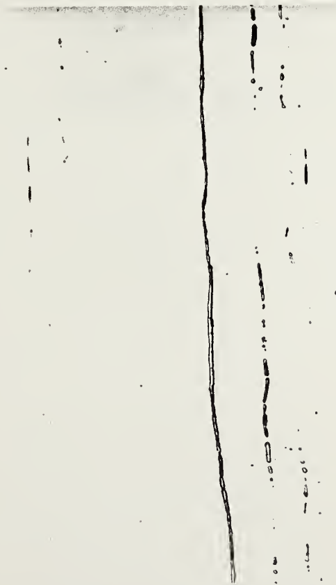
Fig. 7. Photomicrograph at Location D showing typical ferrite stringer. Mag. 500X
