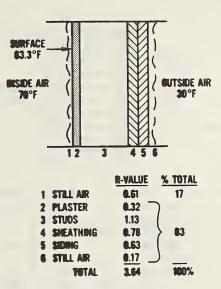
R-value of 3.3. With this type of wall, and the indoor and outdoor conditions described in the first example, the MRT experienced in the above two rooms (i.e., non-corner, or corner) could typically be 68.5 and 67°F, respectively. These conditions would require increases of air temperature of as much as 1.5 and 3 F degrees, respectively, to maintain thermal comfort for typical occupants.
