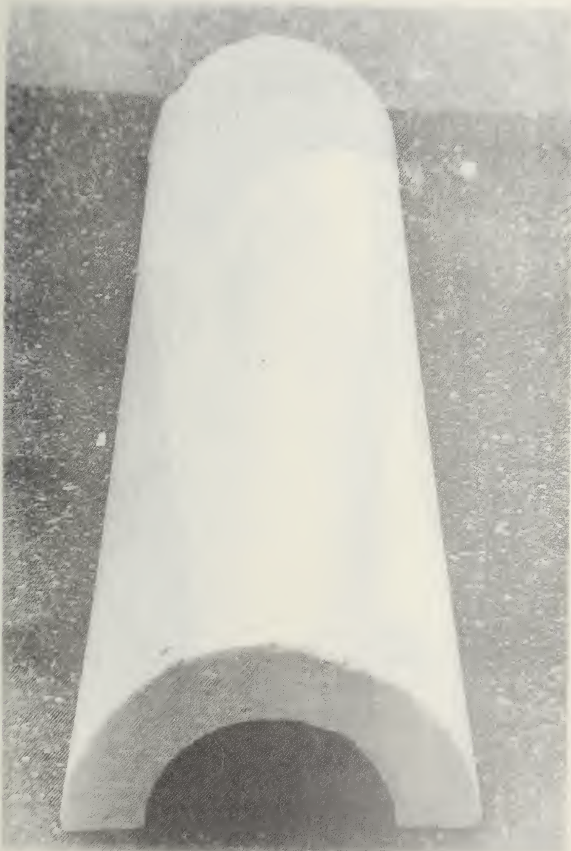
Figure 1/. Conduit side view of PABCO #2 specimen
