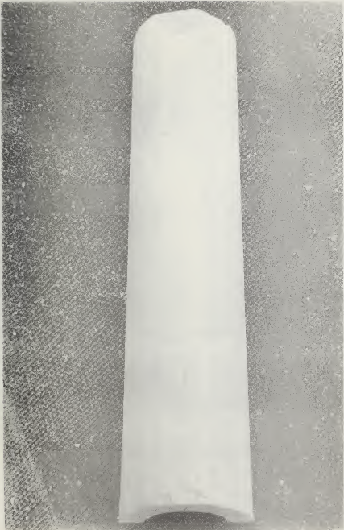
Figure 13. Conduit side view of PABCO #1 specimen
