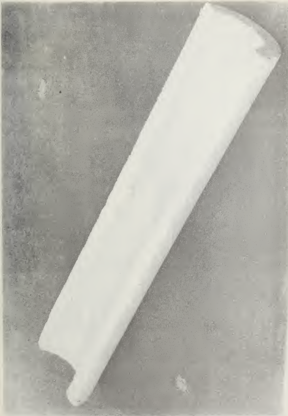
Figure 3. Pipe side view of KAYLO #1 specimen before boiling .
