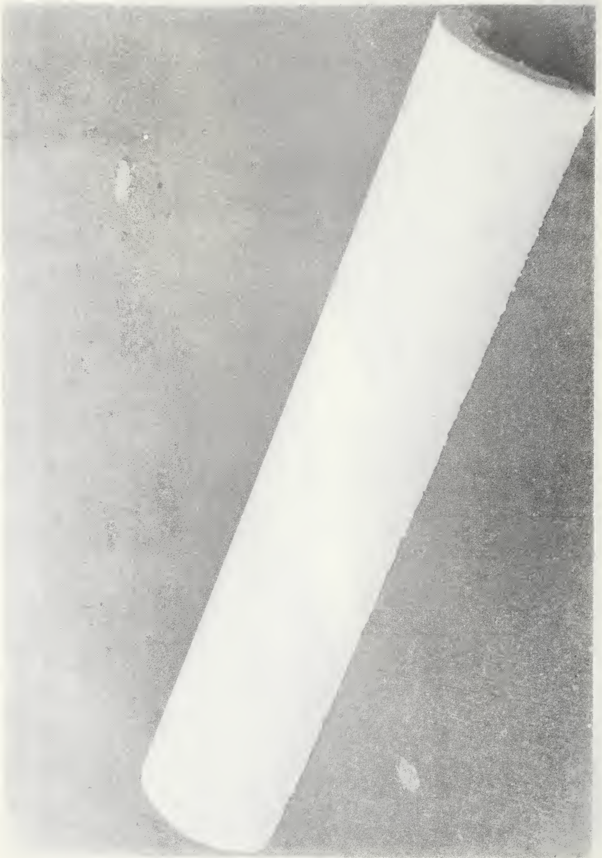
Figure 4. Conduit side view of KAYLO #1 specimen before boiling
