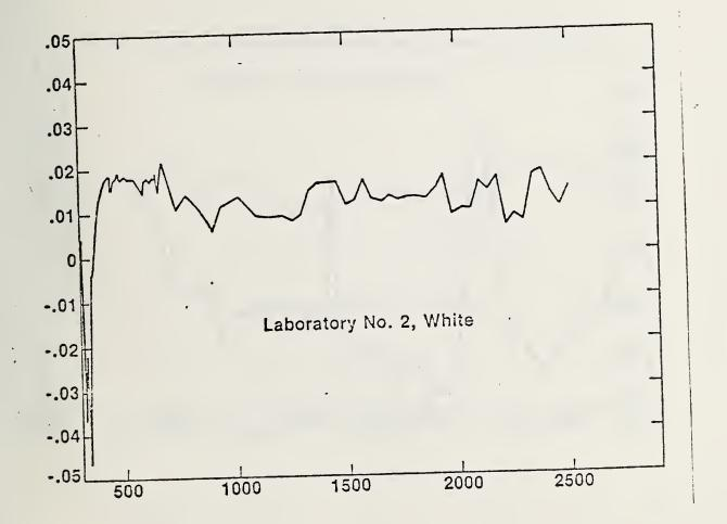
Figure 2 - Difference between data reported by Laboratory 2 and calibration data for the white sample, plotted as a function of wavelength.
