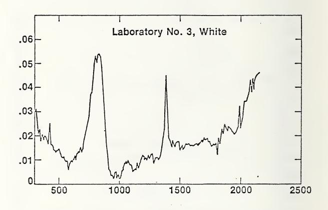
Figure 3 - Difference between data reported by Laboratory 3 and calibration data for the white sample, plotted as a function of wavelength.
