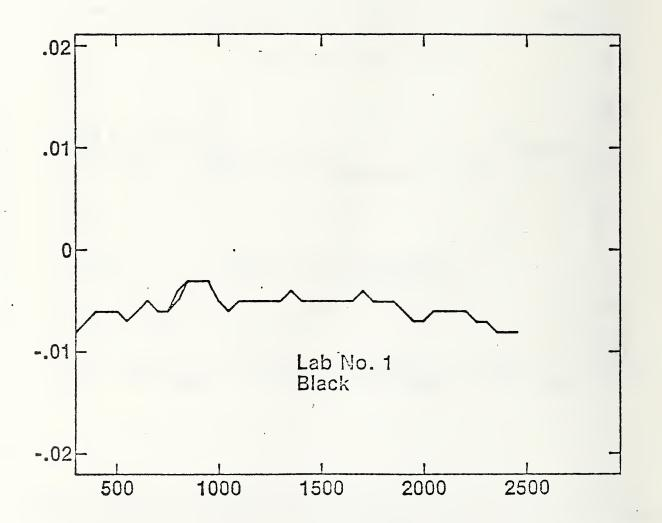
Figure 5 - Difference between the data reported by Laboratory 1 and the calibration data for the black sample, plotted as a function of wavelength.
