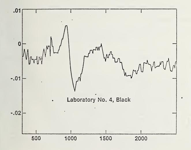
Figure 8 - Difference between data reported by Laboratory 4 and the calibration data for the balck sample, plotted as a function of wavelength.
