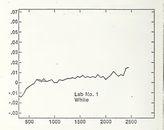
Figure 1 - Difference between the data reported by Laboratory 1 and the calibration data for the white sample, plotted as a function of wavelength.
