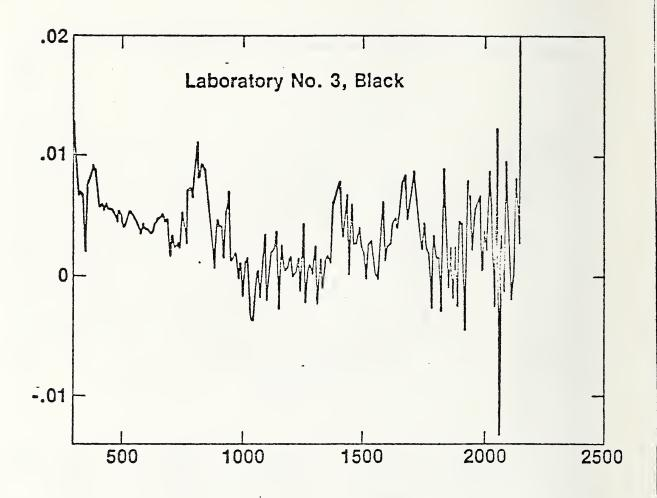
Figure 7 - Difference between the data reported by Laboratory 3 and the calibration data for the black sample, plotted as a function of wavelength.
