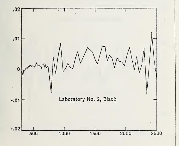
Figure 6 - Difference between the data reported by Laboratory 2 and calibration data for the black sample, plotted as a function of wavelength.
