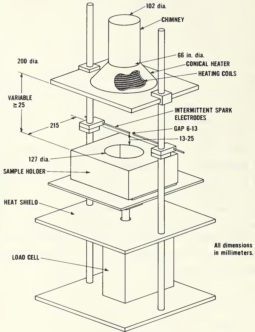
Figure 3. View of ignition test apparatus
