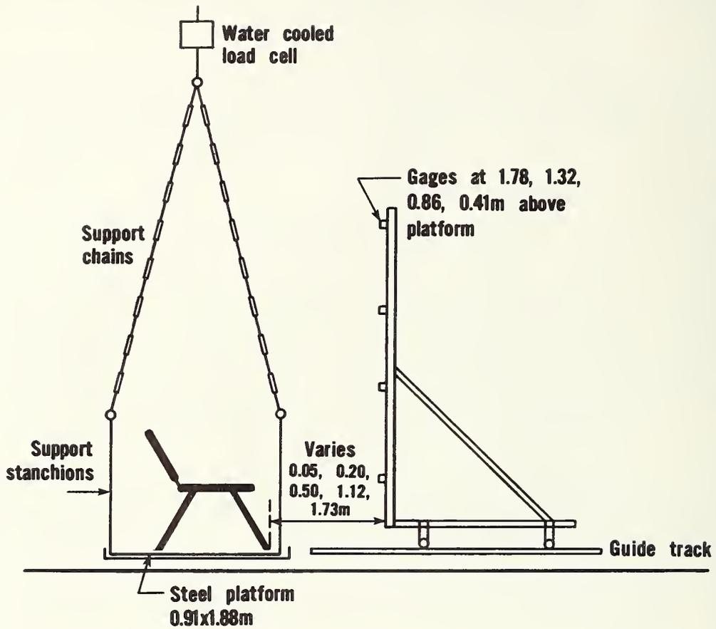
Figure 1. General view of irradiance mapping apparatus and weighing platform
