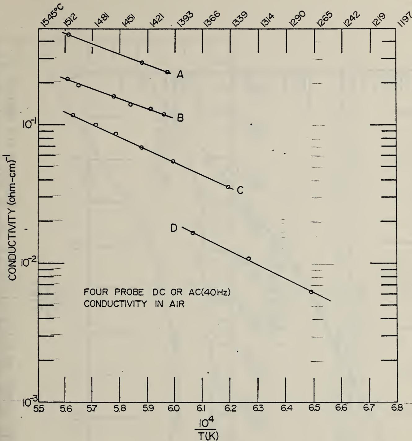
Figure 1. Electrical conductivity vs. temperature of several slags containing amounts of iron. A, B, and C are Eastern slags (Bow, NH) containing 29, 20, and 14 weight percent Fe respectively, but with no added potassium. (See QR April - June 1979, page 33, for base composition). D is a Western slag (Rosebud seam) with 4% iron and with 20%  $K_2SO_4$  added to the melt. (See Table 1, this report, for base composition).
