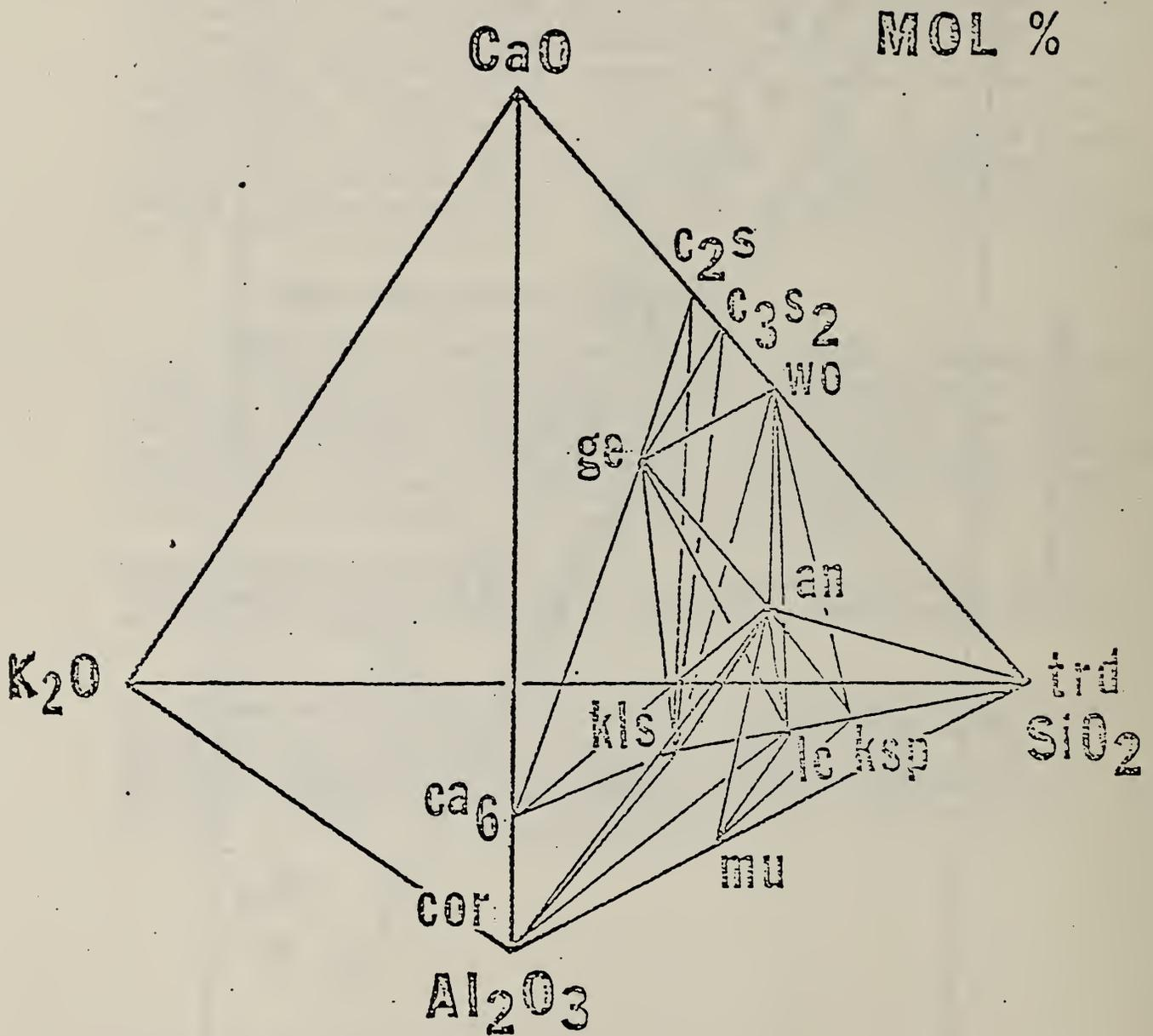
Figure 2. Subsolidus relations for synthetic CaO-K<sub>2</sub>O-Al<sub>2</sub>O<sub>3</sub>-SiO<sub>2</sub> slags, as previously postulated in April-June (1978) Quarterly Report (refer to Table 3 for abbreviations).
