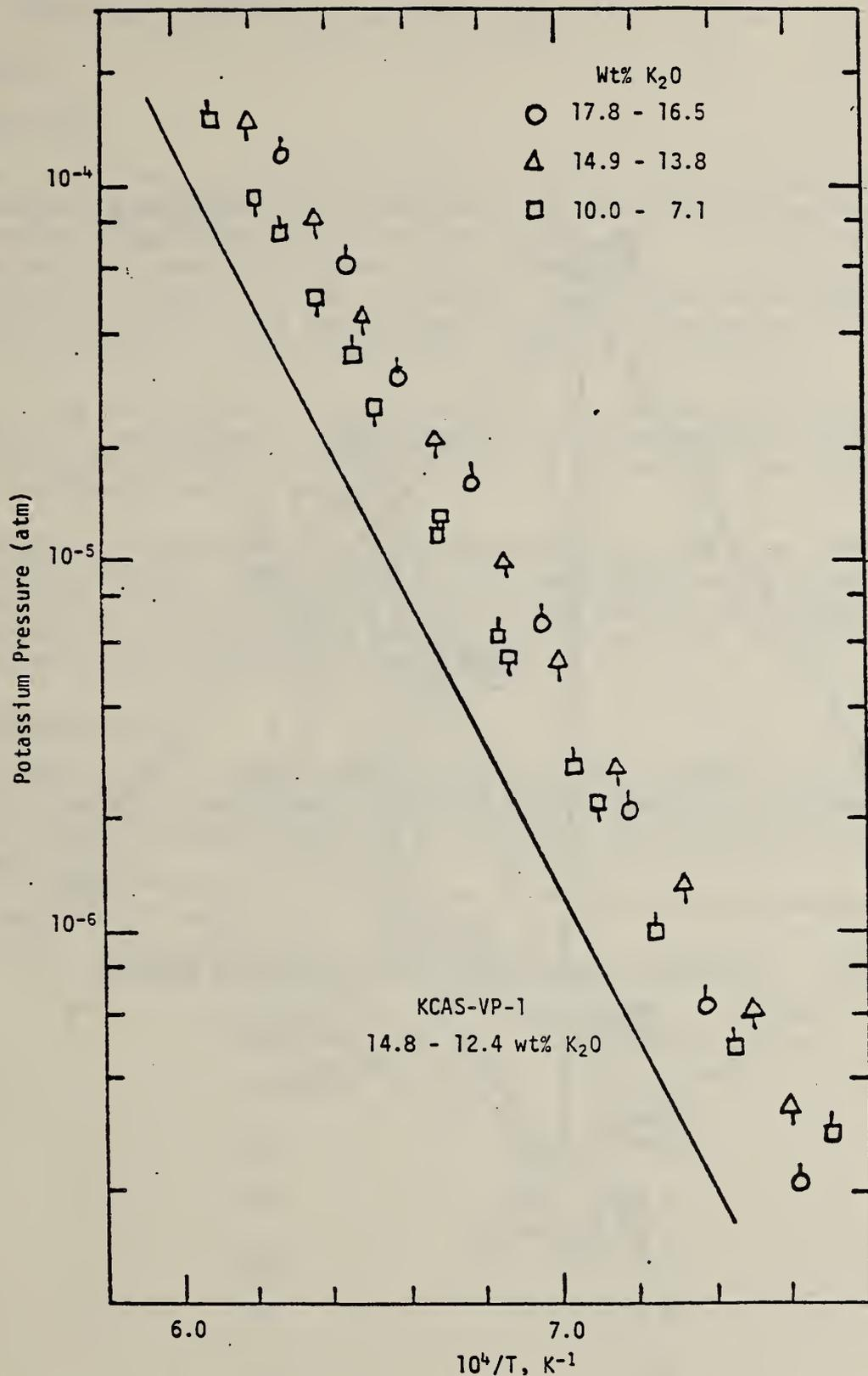
Figure 1. Selected vapor pressures of K above KCAS-VP-4 sample at noted bulk composition of K<sub>2</sub>O vs 10<sup>4</sup>/T. The straight line represents the K pressure over KCAS-VP-1 sample in the K<sub>2</sub>O bulk composition range 14.8-12.4 wt% K<sub>2</sub>O. Upward or downward ticks on points indicate whether temperatures were increased or decreased during the experimental sequence.
