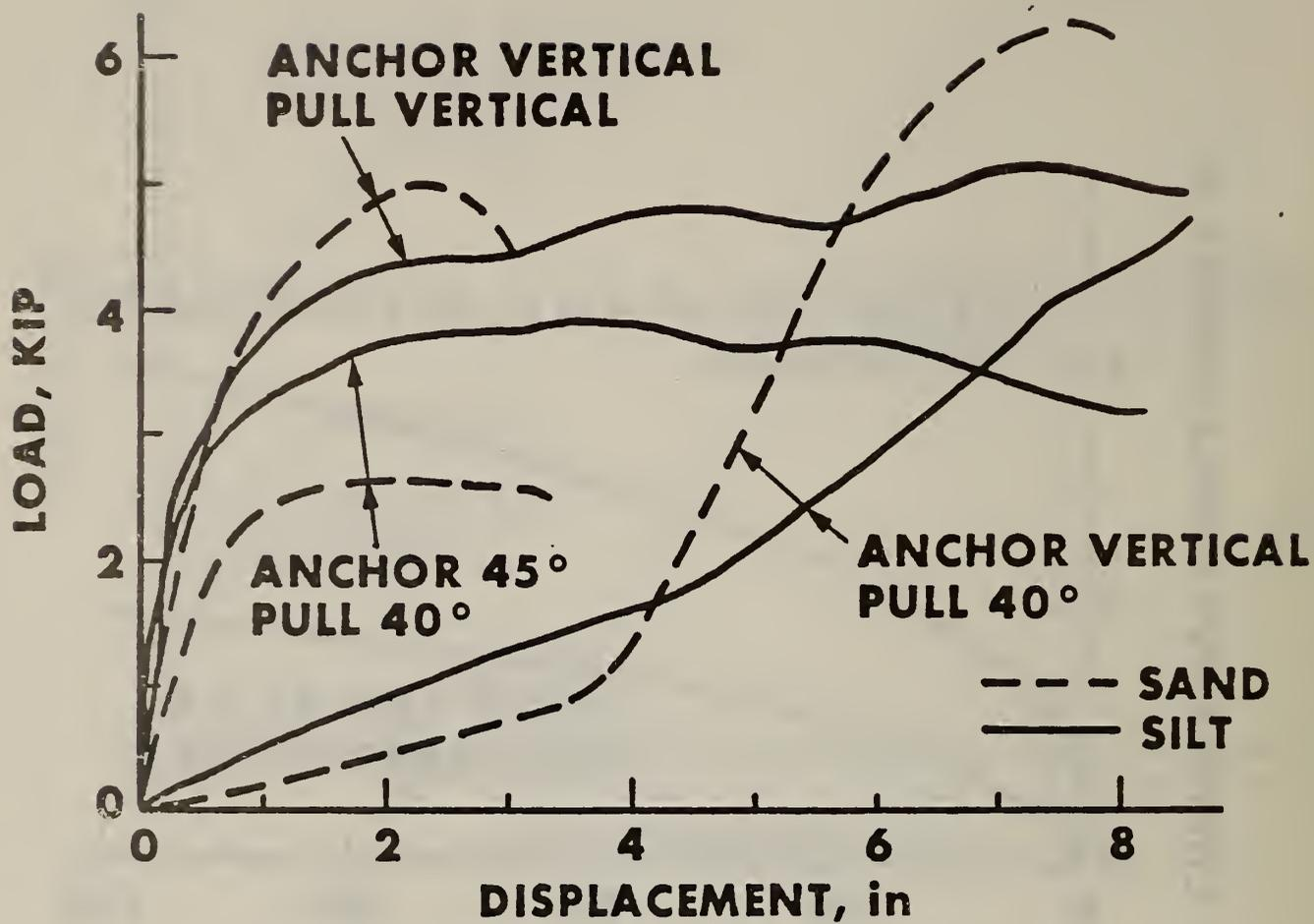
Figure 7. Comparison of monotonic (virgin) loading curves for 6-inch single helix anchors in sand and silt.
