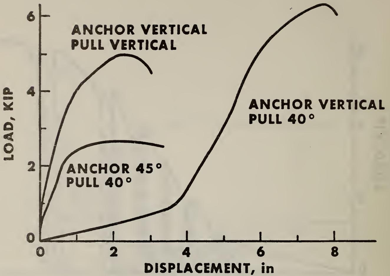
Figure 5. Comparison of the performance of 6-inch single helix anchors in sandy soil under various loading conditions.
