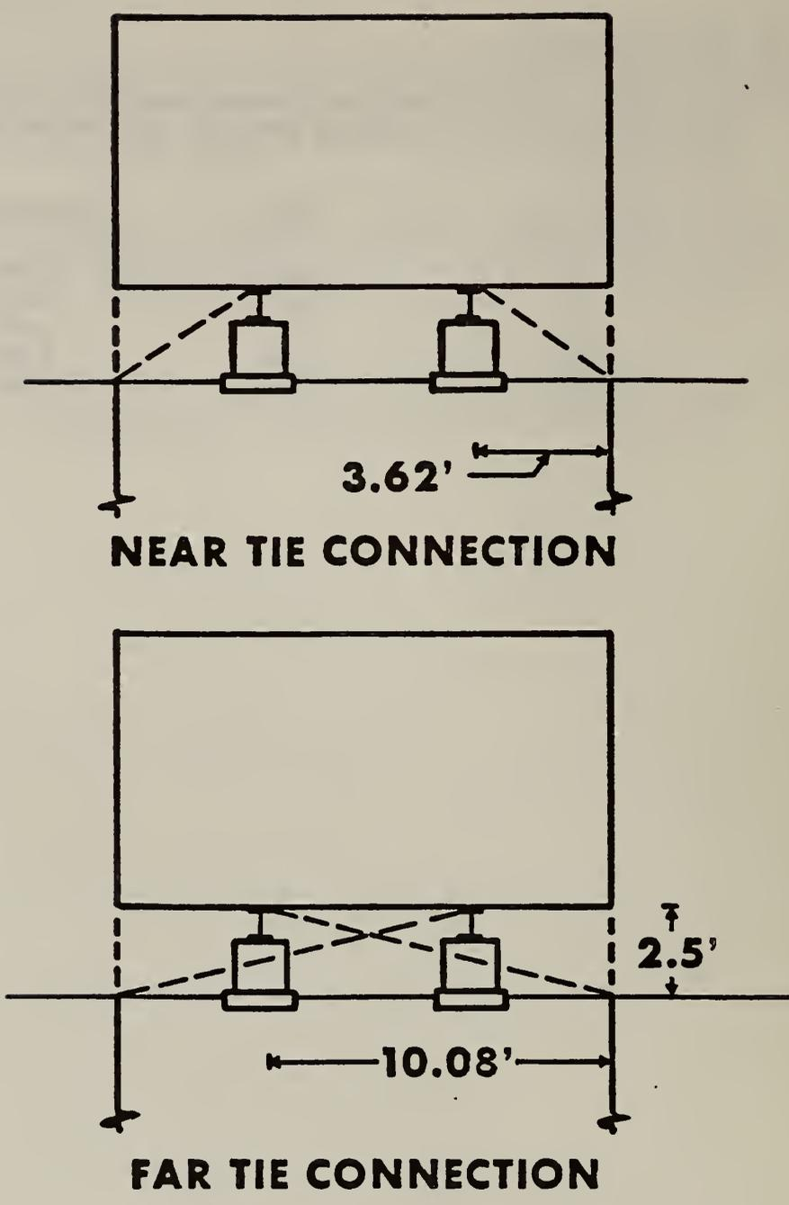
Figure 1. Typical tie down arrangements for a 14-foot wide mobile home.
