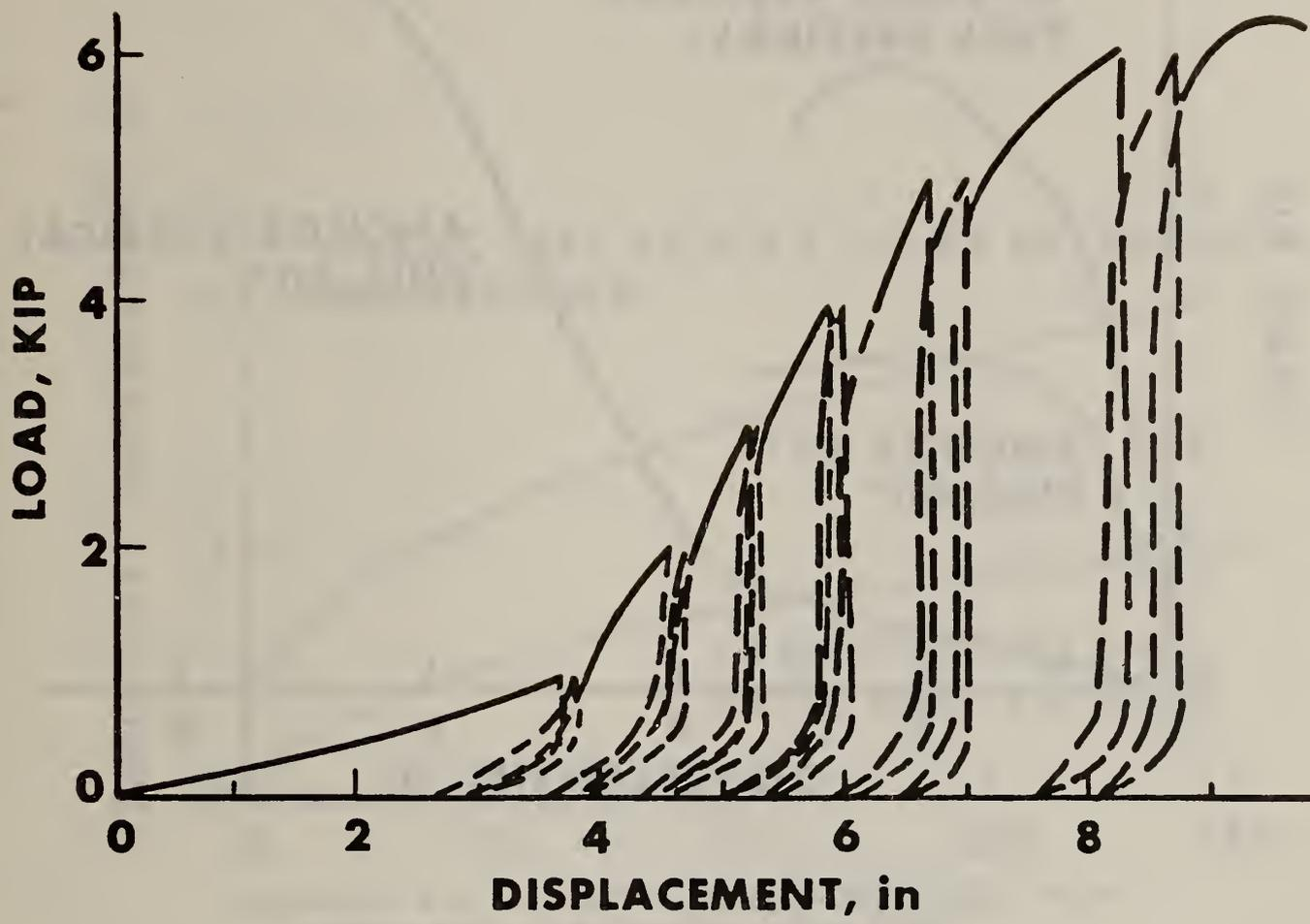
Figure 4. Pullout test load applied at 40° to the horizontal to a vertically installed 6-inch single helix anchor in sandy soil.
