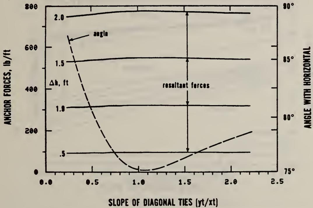
Figure 10 - Resultant Anchor Forces Induced by Floodwater Buoyancy Forces Without Flow Velocity
