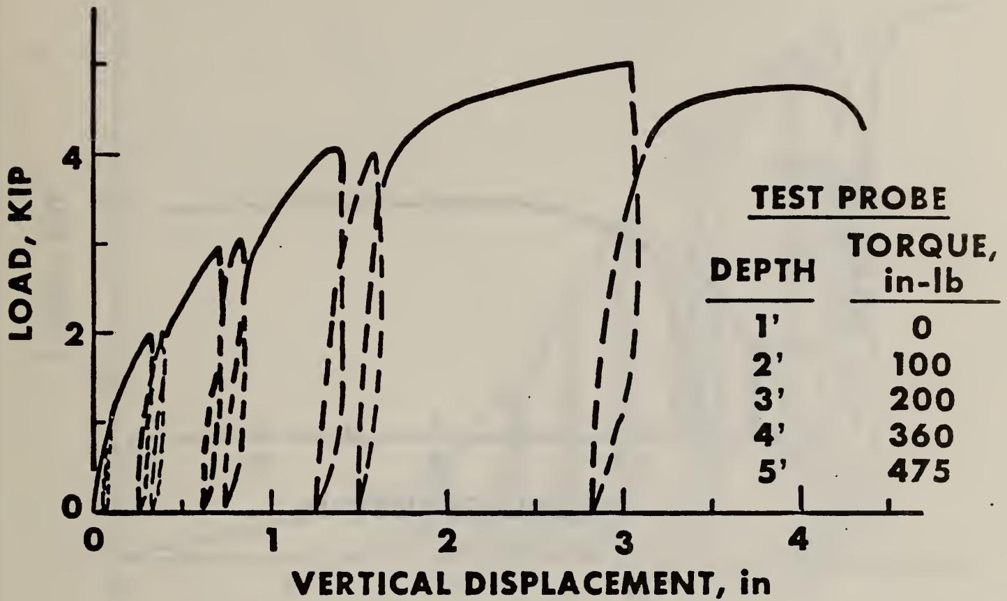
Figure 2. Vertical pullout test on vertically installed 6-inch single helix anchor in sandy soil.
