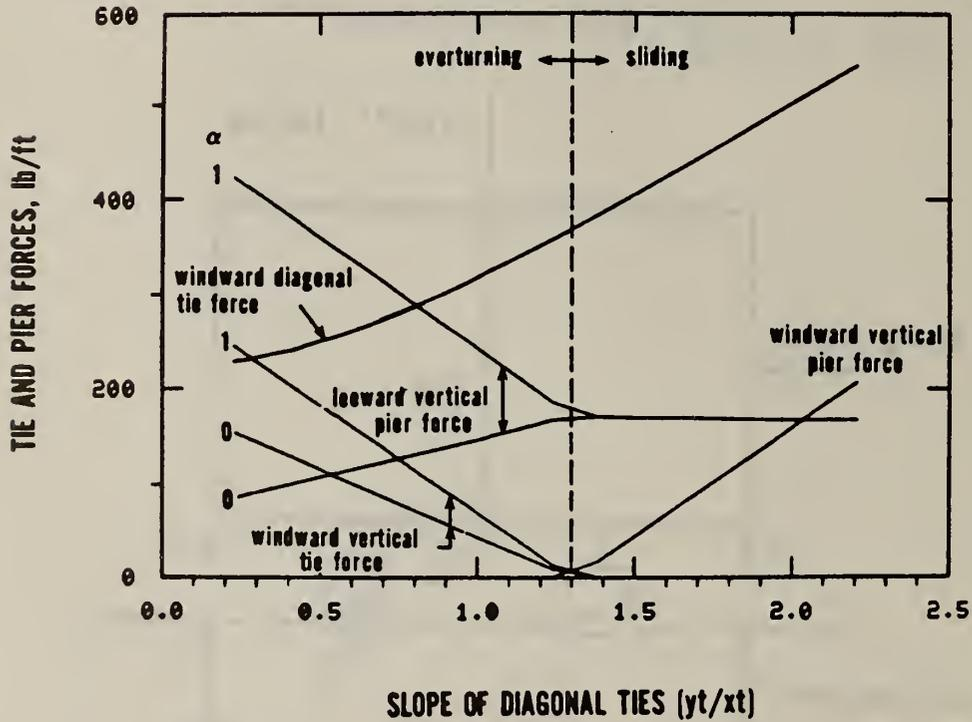
Figure 6 - Tie and Pier Forces for Hurricane Pressures - Near Tie Connection
