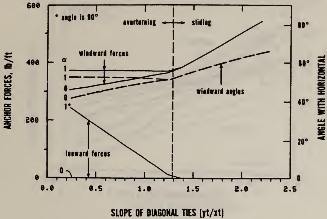
Figure 9 - Resultant Anchor Forces Induced by NBS Hurricane Pressures
