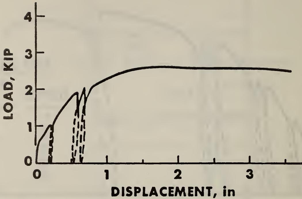
Figure 3. Pullout test load applied at an angle of  $40^\circ$  to the horizontal to a 6-inch single helix anchor installed at  $45^\circ$  to the horizontal in sandy soil.
