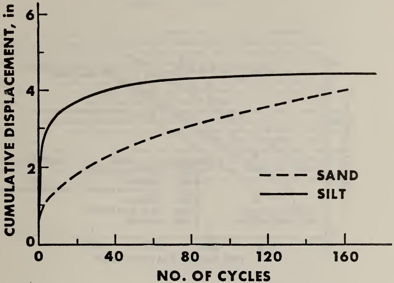
Figure 8. Comparison of cyclic tests on 6-inch single helix anchors installed vertically in sand and silt and subjected to vertical load cycles of 75 percent of ultimate pullout load.
