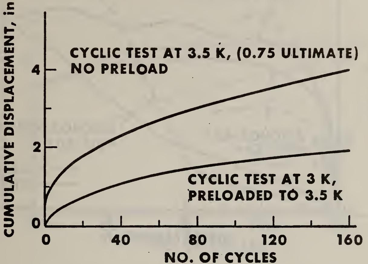
Figure 6. Results of cyclic tests on vertically installed 6-inch single helix anchors in sands subjected to vertical load.
