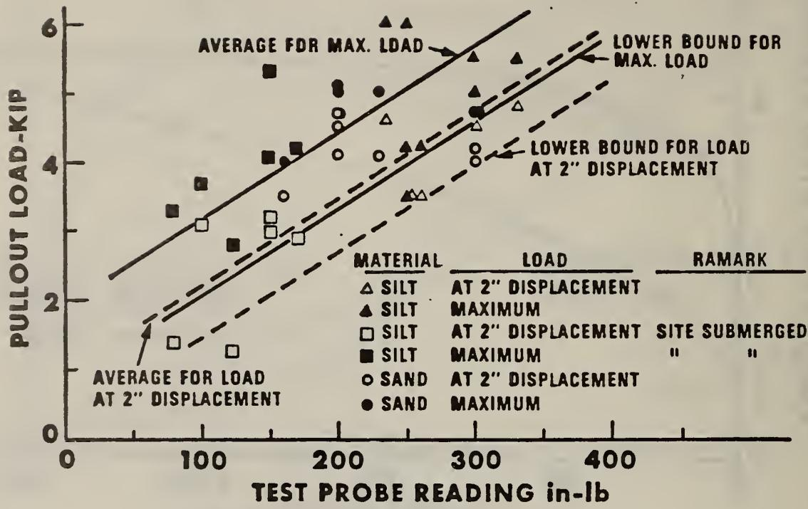
Figure 9. Correlation between test probe readings and 6-inch single helix anchor capacity.
