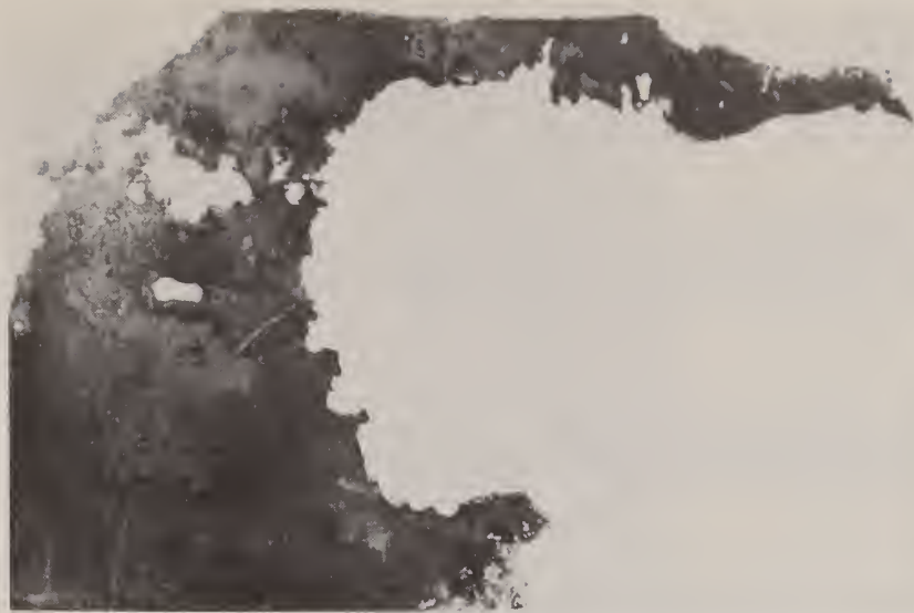
Figure 27. Type 430 stainless steel after burial for approximately 8 years at Site G. This specimen was virtually destroyed due to corrosion. However, a small segment (lower right corner) was unaffected by corrosion. X0.3.
