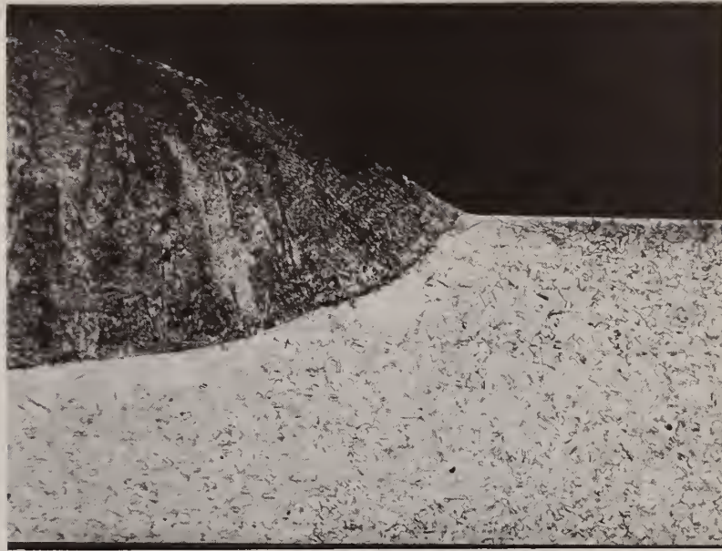
Figure 4. Section from a Type 304 stainless steel specimen at the weld bead area showing little or no apparent heat affected zone adjacent to the weld bead. This was typical for all cross-bead welded materials examined in this study. Etched, 10% oxalic acid. X50.
