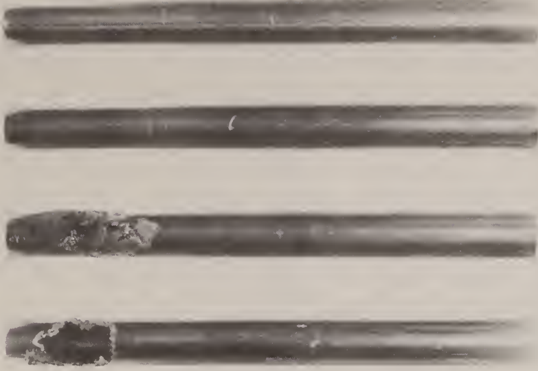
Figure 36. Alloy 18 Cr (Ti) stainless steel tube with a heliarc weld seam after exposure for approximately 7 years at Site C. Note severe corrosion at and adjacent to crevice areas (top ends) on two specimens at the left. Both were perforated due to corrosion. X0.3.
