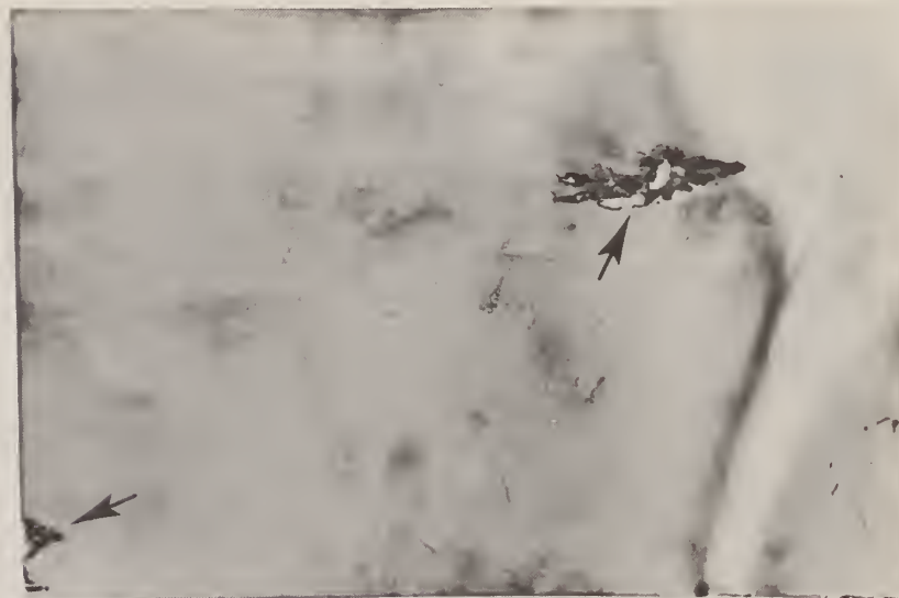
Figure 26. Type 410 stainless steel after burial for approximately 8 years at Site E. Arrows denote areas which exhibited tunneling corrosion. X0.3.
