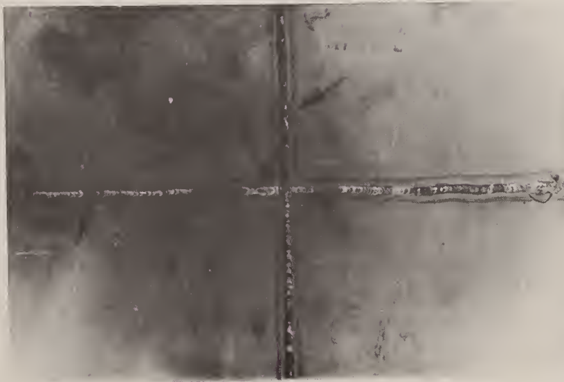
Figure 35. Alloy 18 Cr-2 Mo (Nb) stainless steel with a cross-bead weld after burial for approximately 7 years at Site C. Areas designated by arrows show pitting corrosion observed at the weld beads. X0.3.
