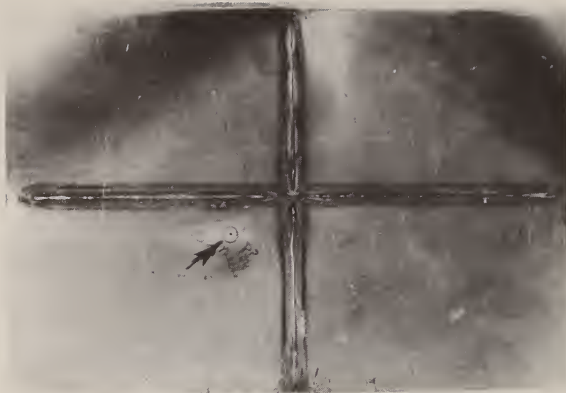
Figure 33. Alloy 18 Cr-8 Ni (N) stainless steel with a cross-bead weld after exposure for approximately 7 years at Site G. Pitting corrosion at area near the weld is shown at arrow. X0.3.
