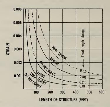
FIGURE A.6 EMPIRICAL RELATIONSHIP BETWEEN STRAIN AND STRUCTURAL DAMAGE
