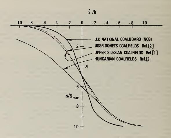
FIGURE A.I MISCELLANEOUS SUBSIDENCE PROFILES
