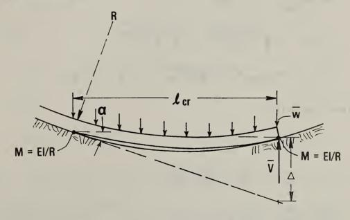
FIGURE B.I ASSUMED IDEALIZED SUPPORT CONDITIONS FOR FLEXIBLE FOUNDATIONS
