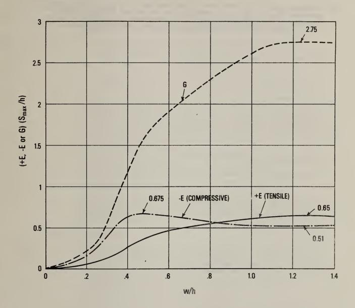
FIGURE A.7 MAXIMUM VALUES OF SLOPE AND STRAINS FOR CRITICAL AND SUBCRITICAL PROFILES
