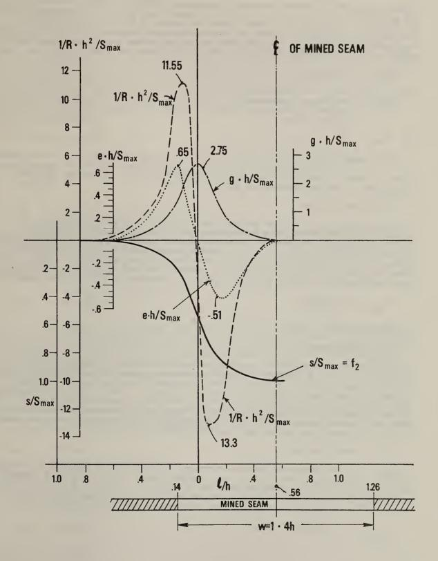
FIGURE A.5 SUBSIDENCE PROFILE CHARACTERISTICS
