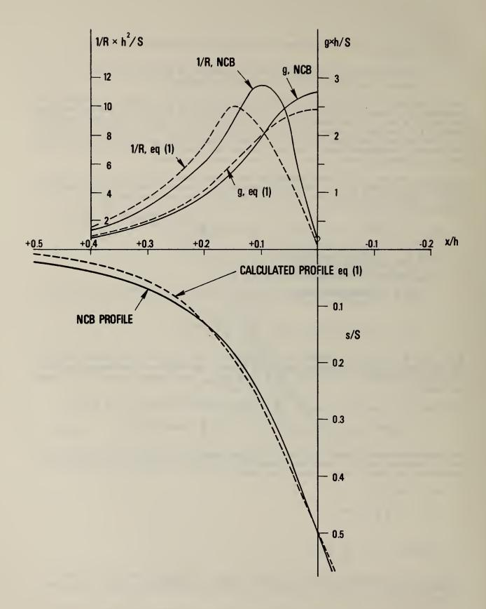
FIGURE A.2 COMPARISON OF NCB CURVE WITH PROFILE FUNCTION
