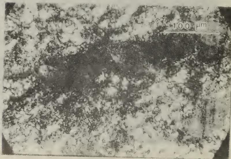
Fig. 7 Light micrographs of an area in a cross-section of a sheet of UH-A polymer molded at 503K. (a) Phase contrast optics, (b) crossed polarizer and analyzer. Note the variation in the sizes of the birefringent structures in (b). The fine variations in contrast in (a) are associated with the birefringent structures in the sample.
