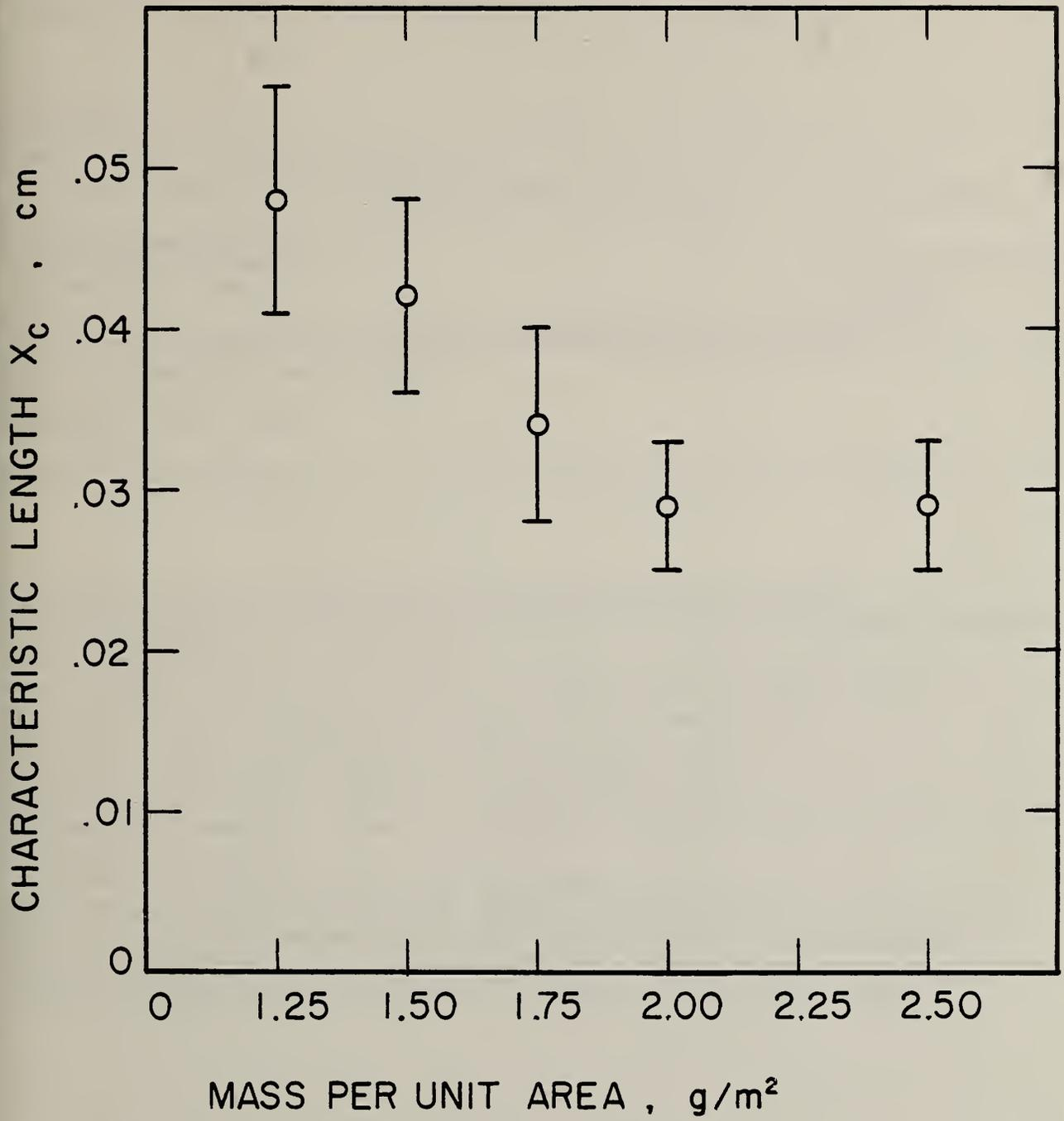
Figure 9. Plot of characteristic lengths  $x_c$  for handsheets of different densities, from table 6.
