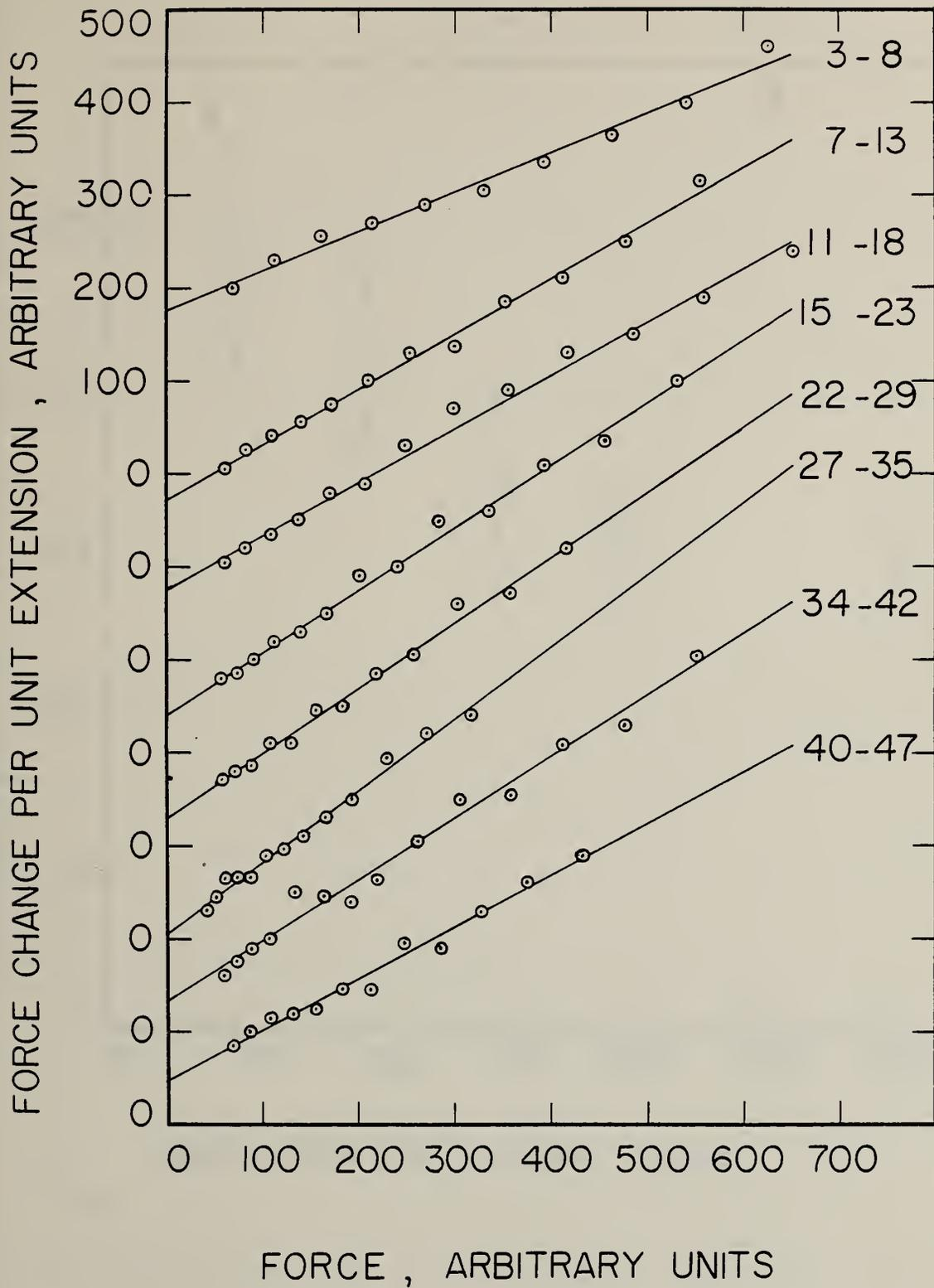
Figure 8. Plots of force change per unit extension versus force for reextension curves, figure 7.
