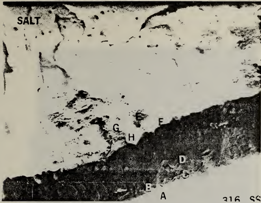
Fig. 45. SEM micrograph, 1160 X, of region 4Z of optical micrograph Fig. 44 showing reaction area at metal-salt interface. Lettered regions correspond to labeled EDX spectra Fig. 46-49.
