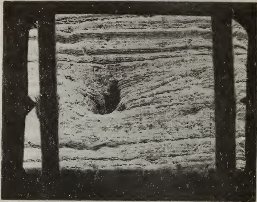
Figure 6. Photoresponse of an EFG cell near a silicon carbide particle producing a point shunt through the cell indicated by the reduced signal as the laser spot approaches the particle.
