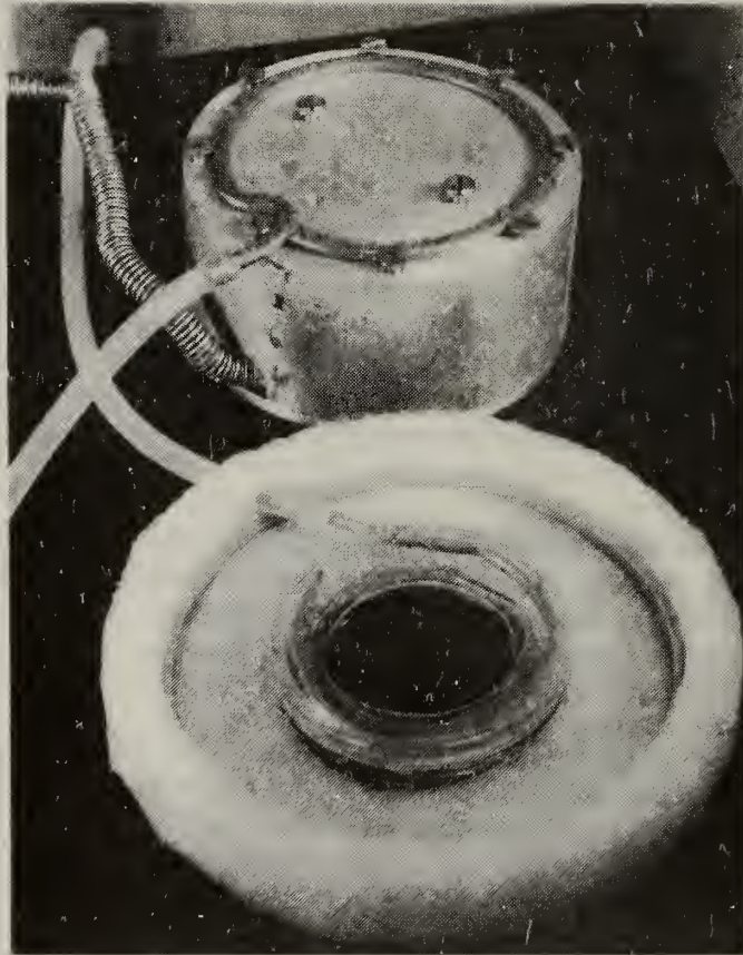
Figure 27. Photograph of the compressor type cooling stage (top) and cover (bottom).
