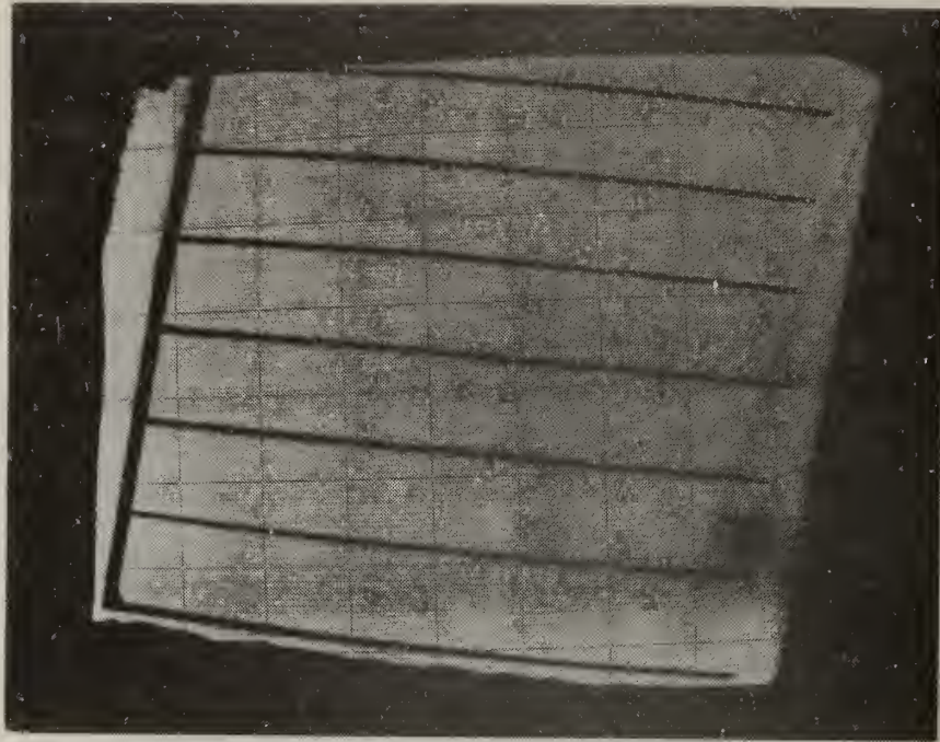
Figure 15. Photoresponse of a high quality 1-cm by 4-cm EFG cell. Laser light is 0.63 \mu\text{m} with no light bias.
