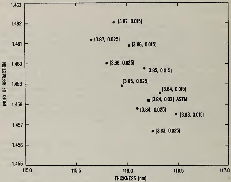
Figure 1. Silicon dioxide thickness and refractive index values calculated from a single set of ellipsometry data by using various silicon optical constants ( $n, k$ ).
